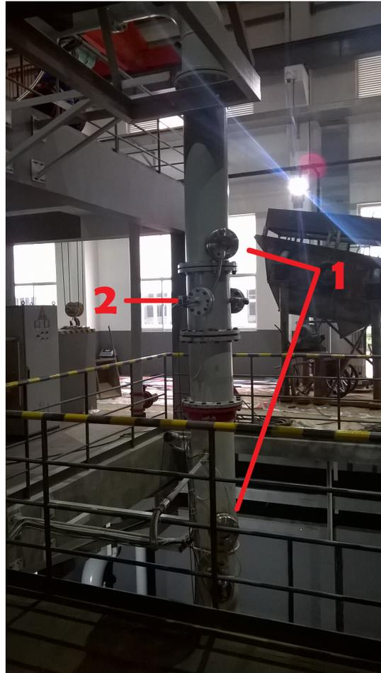
FIGURE 3.2: Upward leg of the U-loop showing pressure sensors (1), and ultrasonic density meter (2).
