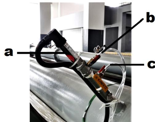
FIGURE 3.3: Pressure tap with: absolute pressure sensor (a), venting tube (b), differential pressure sensor (c). Photo courtesy of M. de Vreede.
