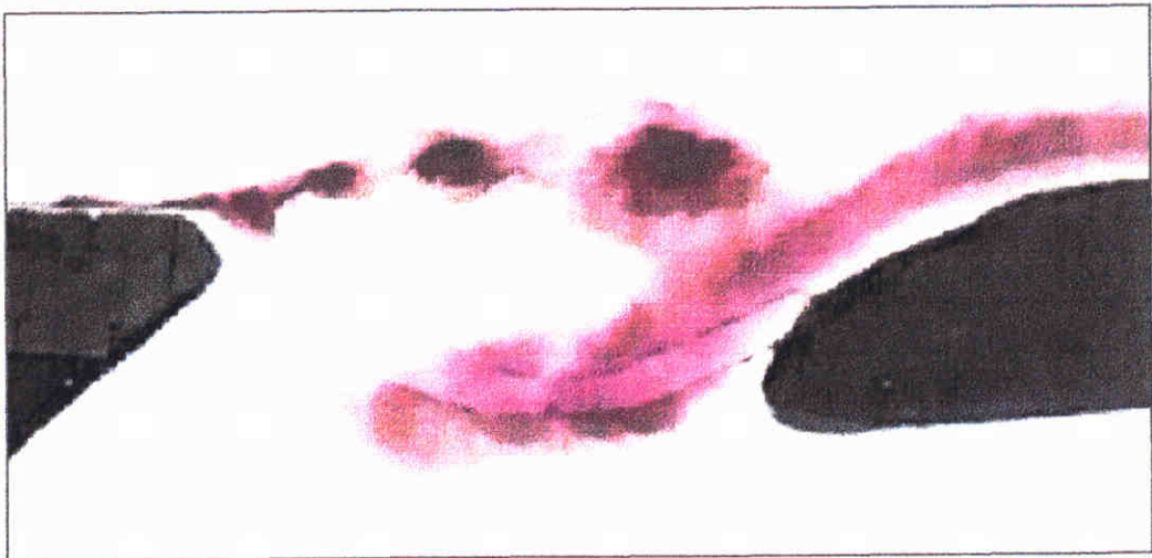
Figure 4.1.3 Top view of a shallow-water mixing layer and flow pattern in a harbour entrance at laboratory scale. Taken from Bijvelds (1997).
