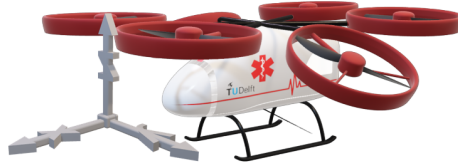
Figure 9.9: Coordinate system used for gust directions
