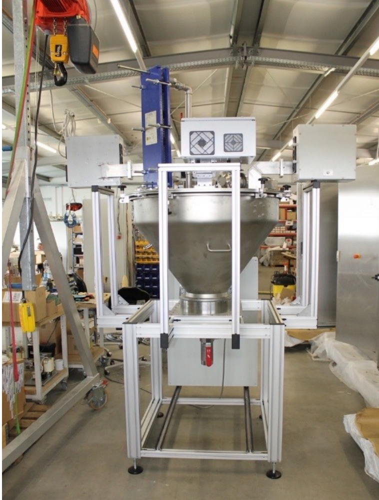
Figure 7-4. The microwave reactor unit version 1 (Photo: D. Brdjanovic)
