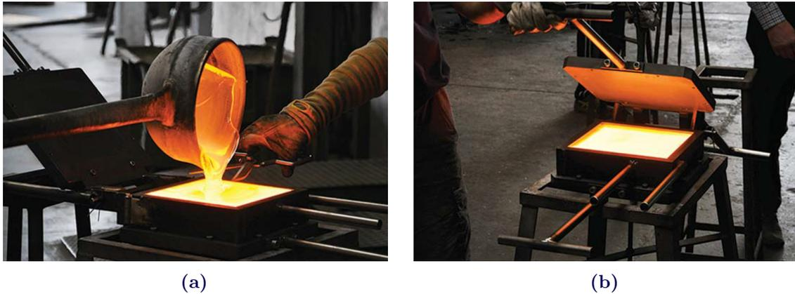
**Figure 5.6:** Cast glass production by Poesia Company, taken from Oikonomopoulou et al. (2014); (a)Casting molten glass into mold; (b)Closing the mold;
