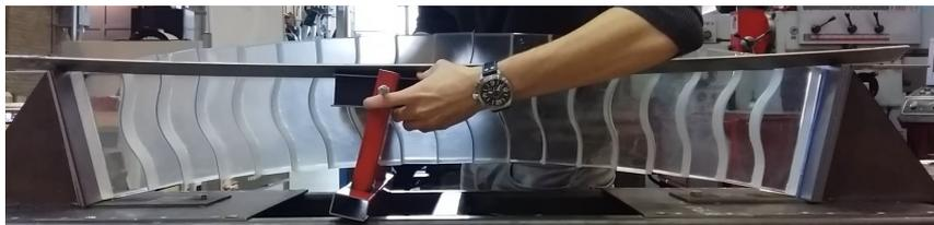
**(c)** Apply lateral (torsional) buckling supports;
