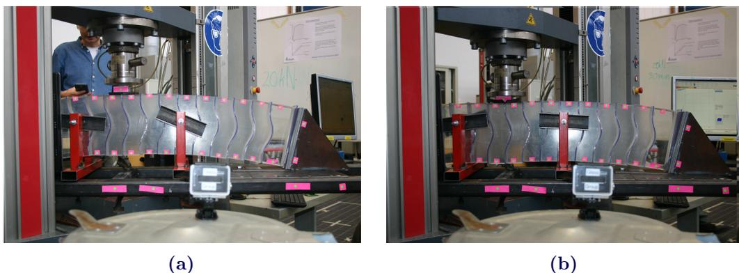
**Figure 9.14:** Photographic displacement measurements; (a)Unloaded; (b)Loaded by 20kN for 30 minutes;
