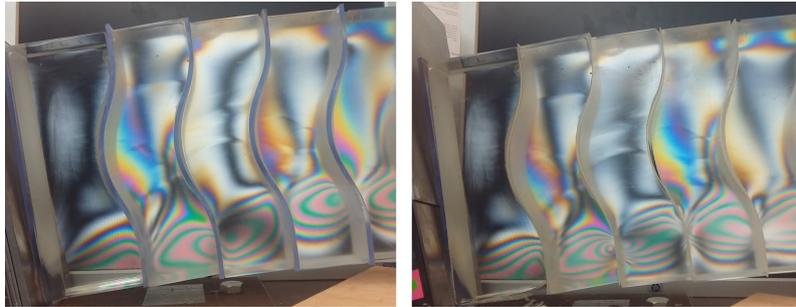
**Figure 9.22:** Polaroid interference pattern at a load of 20kN; (left) 4mm-PVC interlayer; (right) 1mm-PU interlayer;
