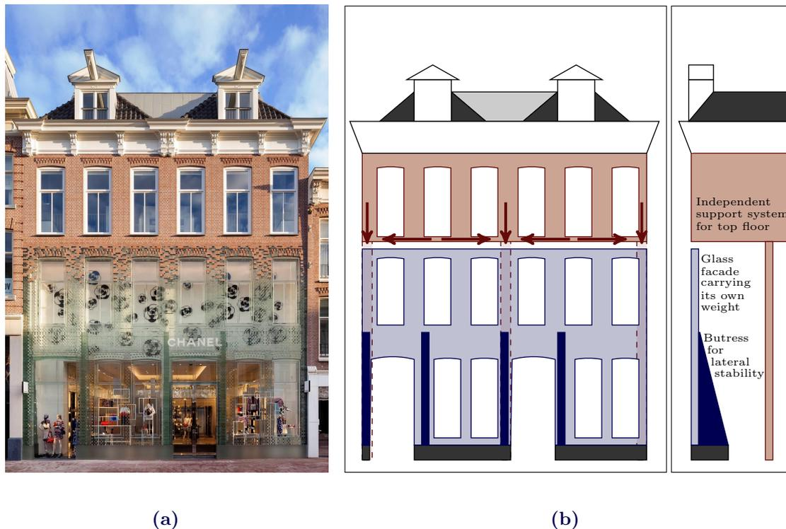
**Figure 3.8:** Crystal Houses; (a) Impression, taken from mvr.dv.nl; (b) Structural scheme;
