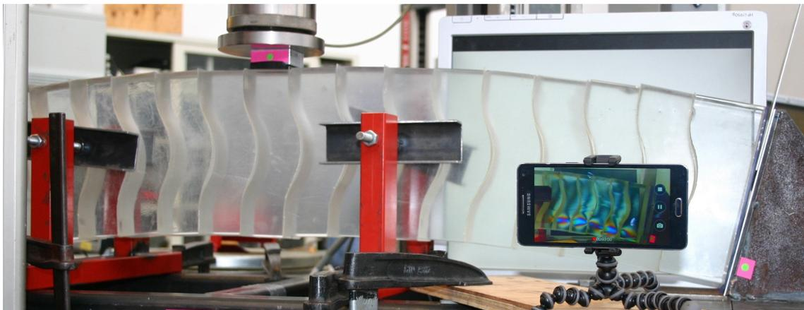
**Figure 9.19:** Plane polariscope setup for optical stress measurements: LCD-screen, glass arch, polaroid filter, camera;
