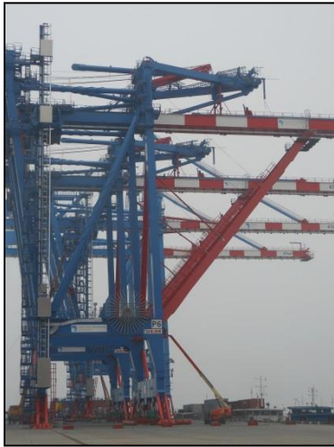
Figure 4.20 A-frame positioned horizontally due to height restrictions experienced during sea transport
