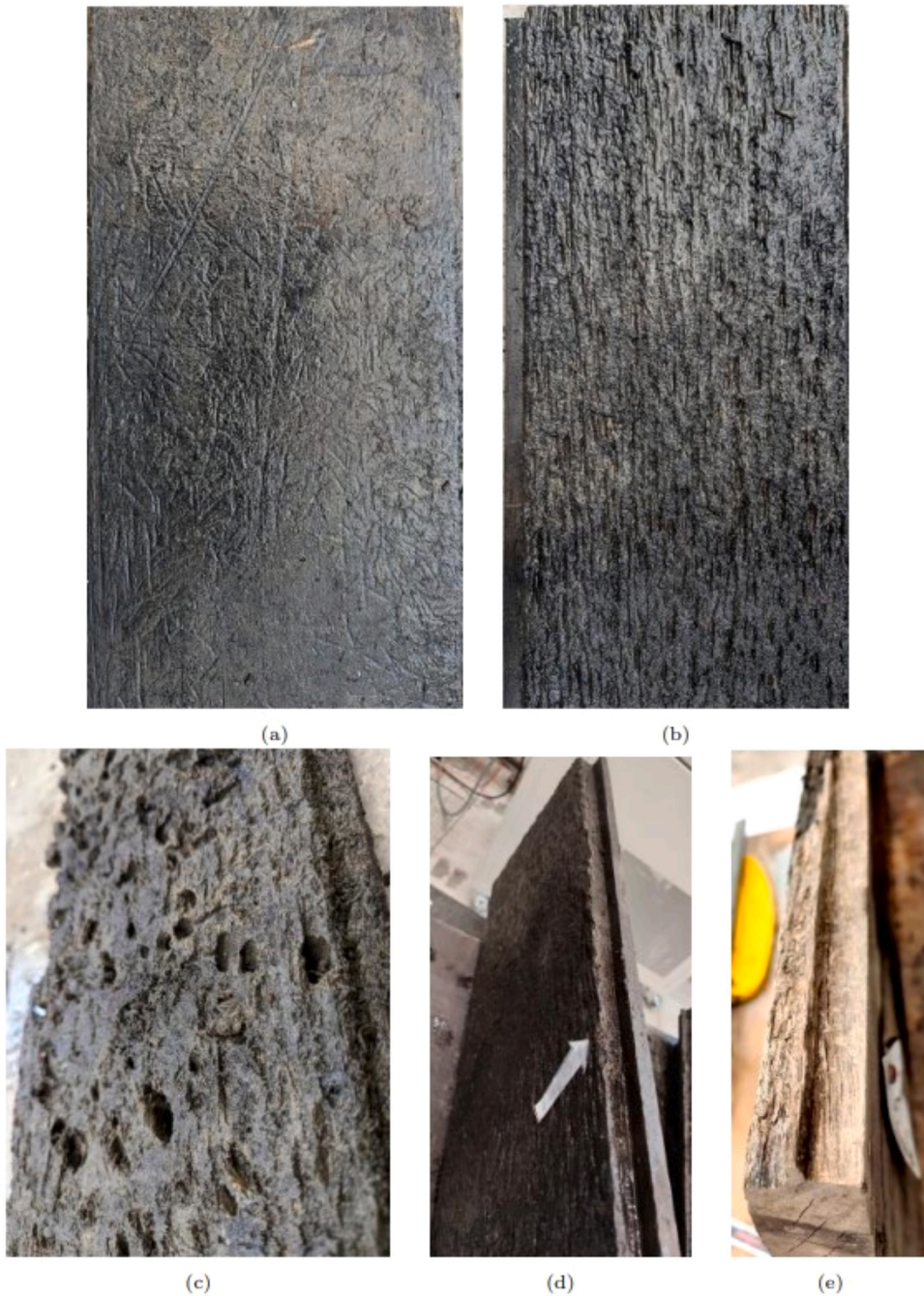
Fig. 9. Deterioration observed on the recovered azobé boards a)Earth side b)Shallow stripes observed on water side c)Severe water side deterioration d)Water side deterioration of the groove e)Water side deterioration of the tongue.
