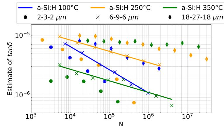
Fig. VII The loss tangents ( $\tan\delta$ ) that we estimated by referencing to a chip directly on top of the c-Si substrate. The x-axis shows the number of photons in the resonator. The symbols denote the CPW slot and line widths.
