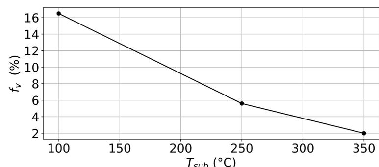
Fig. V The void volume fraction determined by ellipsometry using the Bruggeman effective medium approximation.
