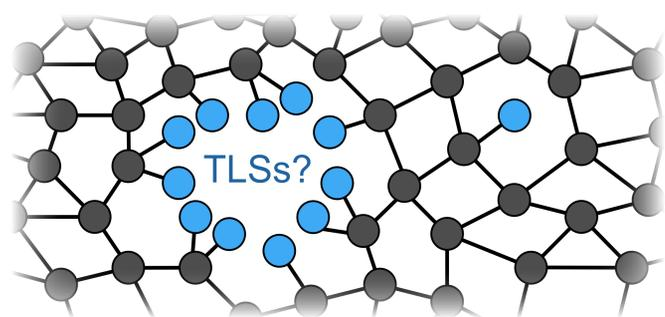
Fig. I Schematic of a-Si:H. Grey: Si atoms. Blue: H atoms. The SiH<sub>2</sub> bonds exist on the surface of voids.
