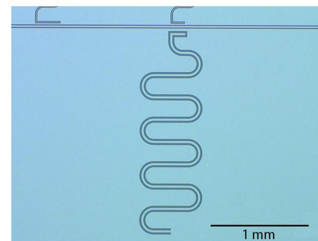
Fig. VI Micrograph of one of the aluminum quarter-wavelength coplanar waveguide (CPW) resonators that we used to measure the loss tangent ( $\tan\delta$ ) at 120 mK and at 5-7 GHz. The chip contains multiple CPW geometries.
