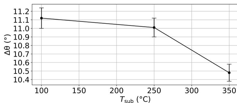
Fig. IV The bond-angle disorder determined by Raman spectroscopy.
