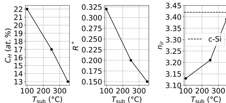
Fig. III Hydrogen content ( $C_H$ ), microstructure parameter ( $R^*$ ), and infrared refractive index ( $n_{\text{ir}}$ ) determined by FTIR spectroscopy. A larger  $R^*$  indicates more voids.
