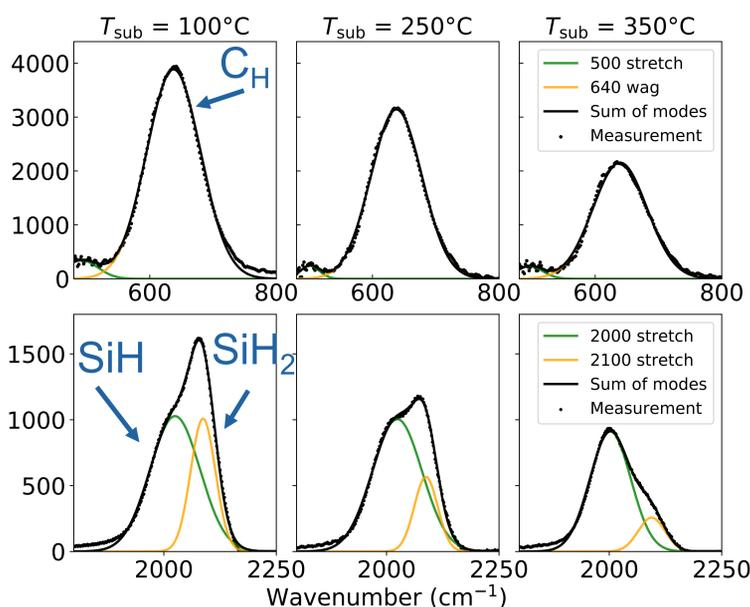
Fig. II Fourier-transform infrared (FTIR) absorption coefficient ( $\alpha$ ) measurements, showing the stretching and wagging modes from which we determined the hydrogen content ( $C_H$ ) and the microstructure parameter ( $R^*$ )<sup>7</sup>.
