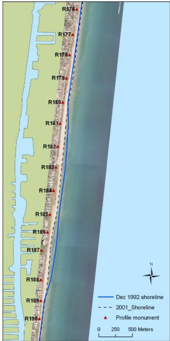
Figure 2.2. Shoreline positions overlaid on georectified aerial photography obtained in 2001. The 1992 shorelines shown were surveyed immediately after construction of the 1992 nourishment project (Dec, 1992) and June 2001 is the last complete survey of the project area prior to the construction of the fourth consecutive nourishment project in April 2002.
