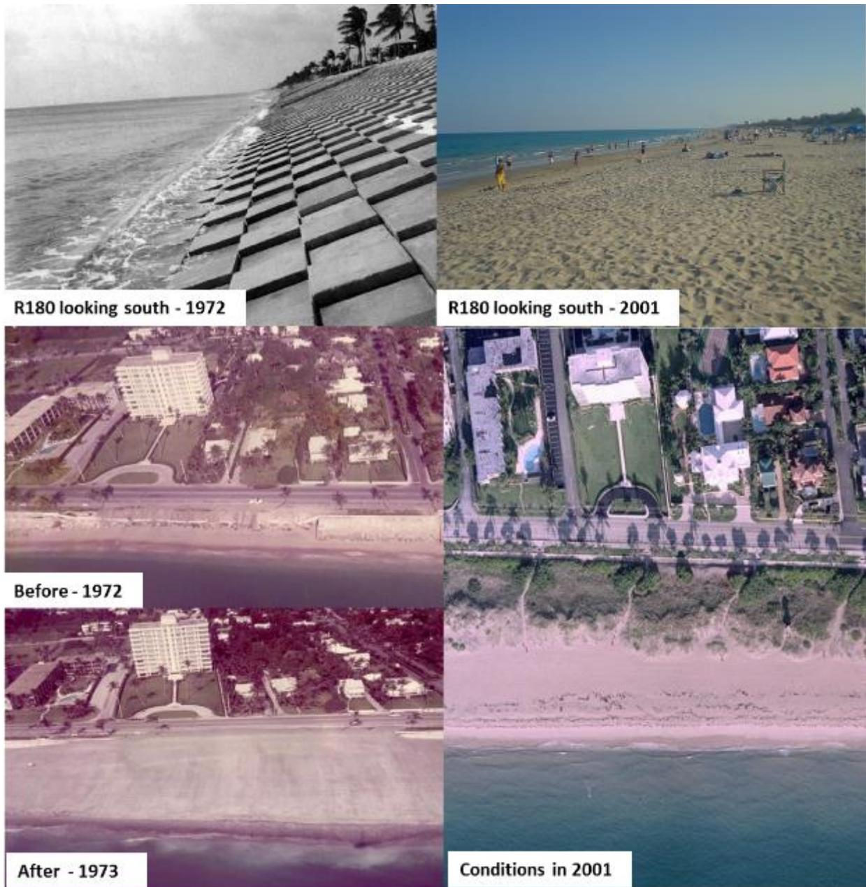
Figure 1.4. Pictures illustrating the conditions of Delray Beach in 1972, before the 1973 beach nourishment project, in 1973 soon after the nourishment construction and in 2001 showing a fully restored beach with dune vegetation well established.
