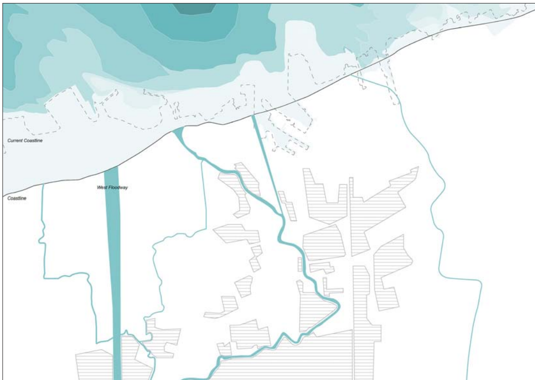
1850: Build West Floodway. The West Floodway was built to channel the water from the hills and Garang river. After the establishment of the floodway, Semarang river lost its role as a port. Moreover, sedimentation phenomenon started to get worse because of smaller water volume, meanwhile the river got polluted from daily use.
