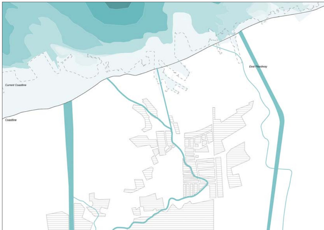
1894: Build East Floodway. The East Floodway was built to channel the water from Penggaron river and solve the flood risk from hilly area.
