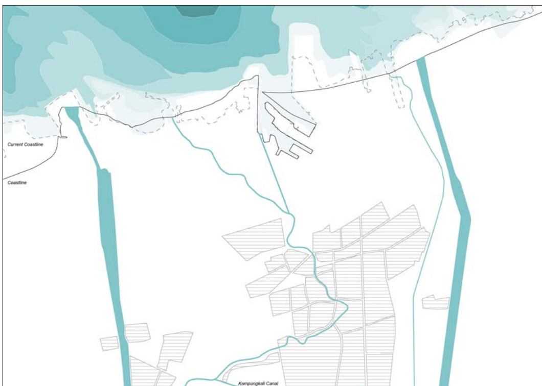
1936: Build several canals in central part. The flood risk in the central part stay severe so several canals were built to direct the water from the hills.
