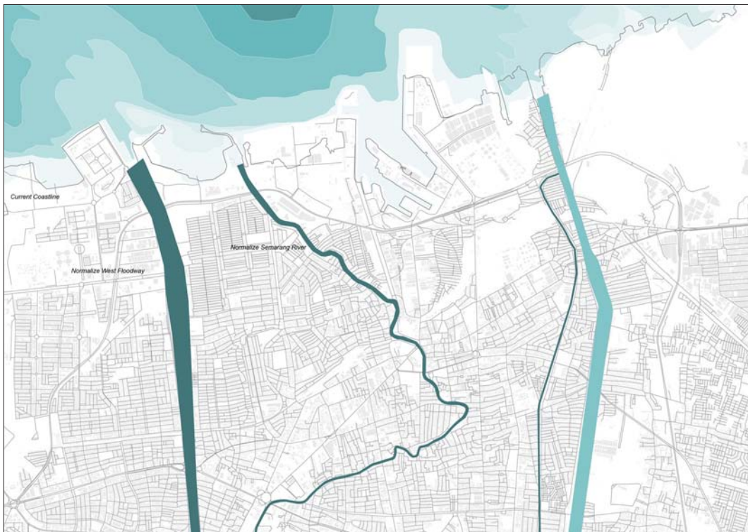
2010: Normalized West Floodway, Garang River, Semarang River. These waterways got silted because of sedimentation, the action of normalization tried to keep them function normally and mitigate the flood.
