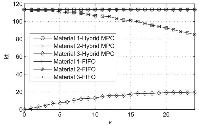
Fig. 16. Comparison of the average quantities of three materials in the stockyard over the course of the simulation.
