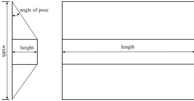
Fig. 7. Side and top views of the trapezoidal stockpile.
