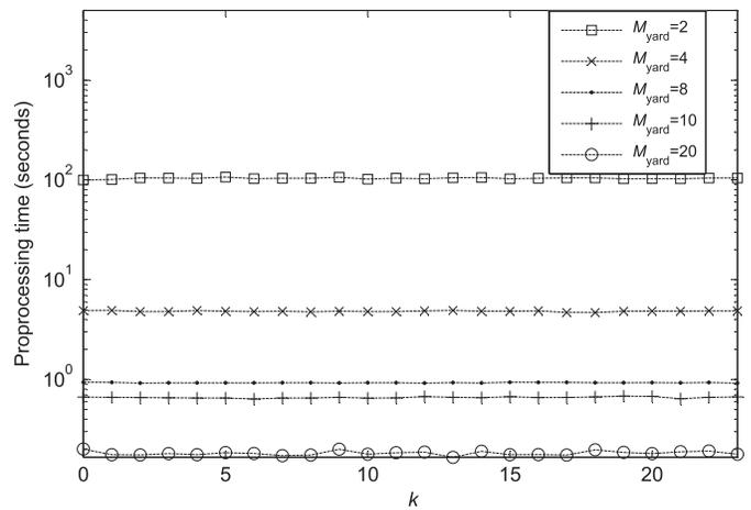
Fig. 12. Average preprocessing time of the MPC controller at each time instant under different  $M_{yard}$  values.
