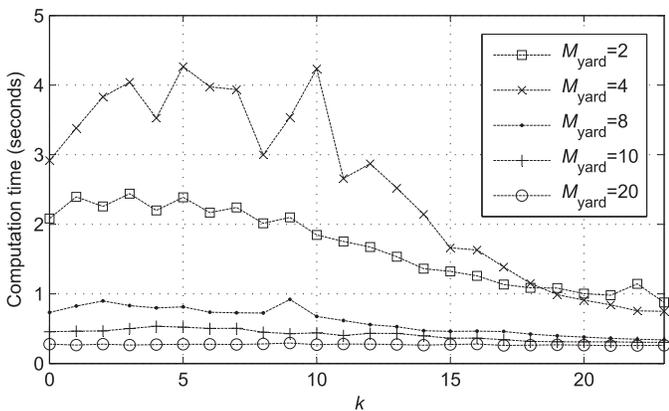
Fig. 10. Average computation time of the MPC controller at each time instant under different  $M_{yard}$  values.
