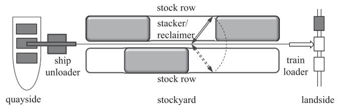
Fig. 1. Schematic of a small import dry bulk terminal.
