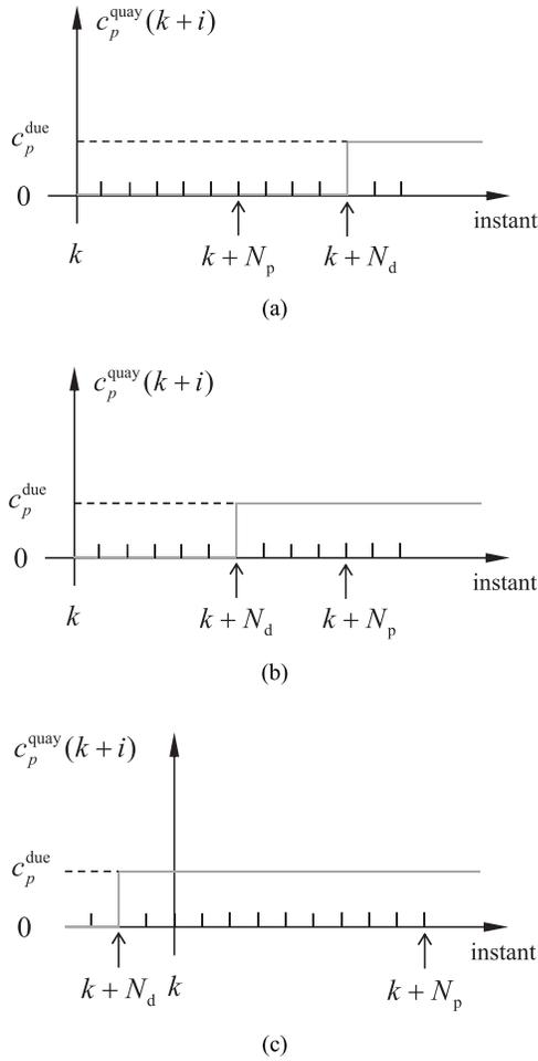
Fig. 5. Curves of  $c_p^{\text{quay}}(k+i)$  under three different conditions. (a) Due time horizon is ahead of the prediction horizon ( $N_p \leq N_d$ ). (b) Due time horizon is within the prediction horizon ( $N_p > N_d$ ,  $N_d > 0$ ). (c) Due time cannot be met ( $N_p > N_d$ ,  $N_d \leq 0$ ).
