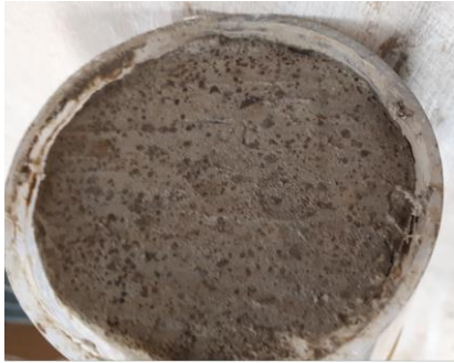
Figure 133: Mottled pattern on the side of core 5 (63mm in inside diameter) at site 1672.
