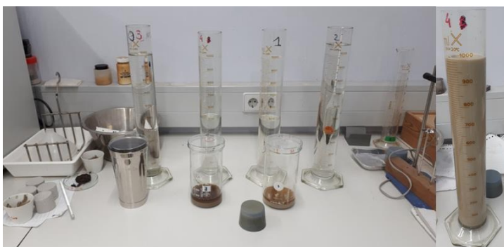
Figure 19: Hydrometer setup on the left and a cylinder full of silt and clay particles on the right
