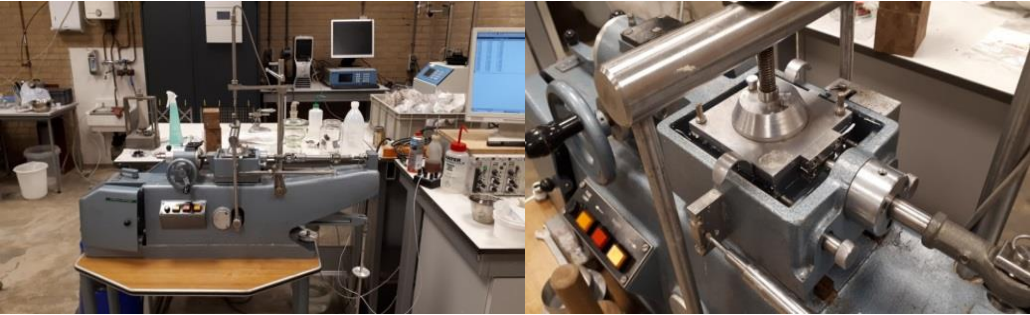
Figure 25: The direct sheartest in the climate room shown with a consolidated sample in a wet condition.
