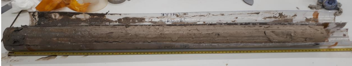
Figure 29: Example of a gravity core 10 opened with the top of the plastic cylinder cut off.
