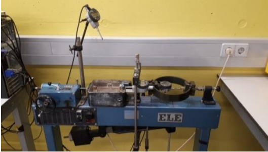
Figure 27: The direct shearbox in the main laboratory.
