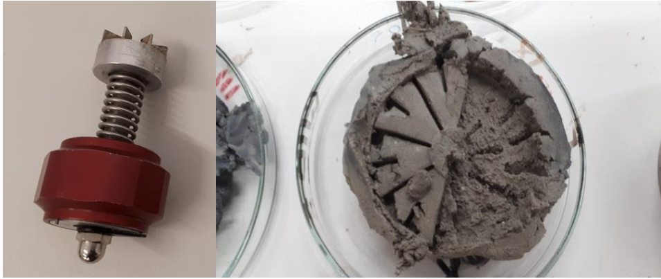
Figure 16: Pocket vane test on the left and tested soil sample on the right with a 55 mm imprint.
