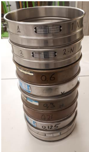
Figure 18: Sieving tower used for wet sieving.
