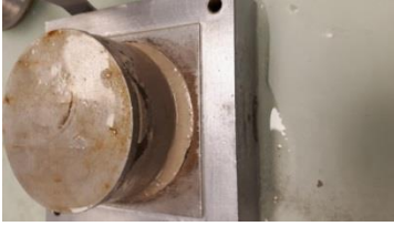
Figure 26: A sheared sample (60mm in diameter) of the direct sheartest from the climate room.
