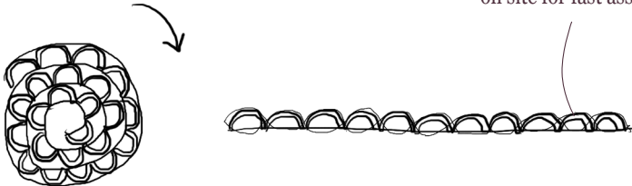
split bamboo flooring panels that are unrolled on site for fast assembly
