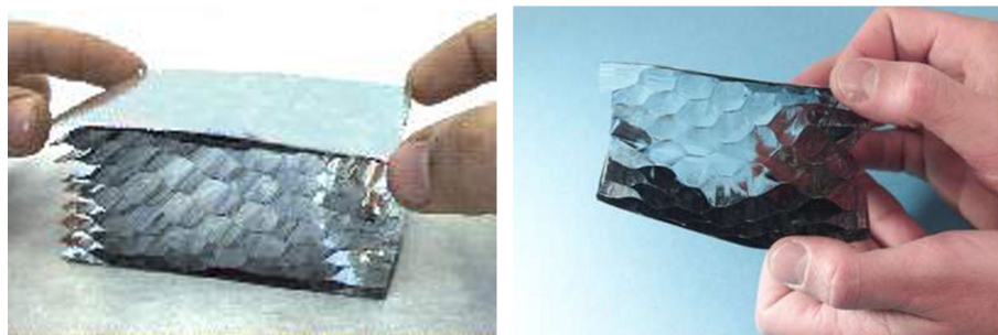
Figure 2.9: Example of an Gas Filled Panel (GFP) insulation material, including the barrier foil and baffle structure inside the GFP. (Jelle, 2011)
