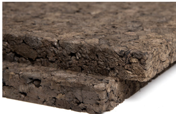
Figure 2.4: Example of cork insulation boards (MaterialDistrict, 2025)
