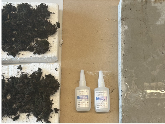
(a) Setup for glueing moss to the panels
