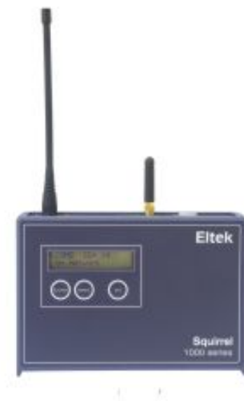
Figure C.3: SRV250 receiver logger (Eltek Ltd., 2025)
