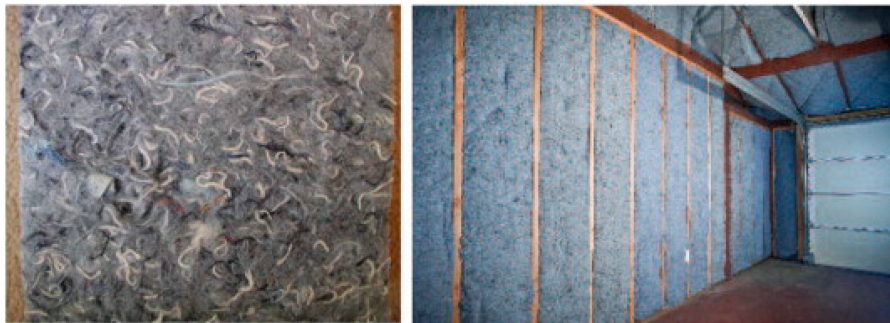
Figure 2.7: Example of insulation boards made from recycled cotton its application to building panel insulation. (Ali et al., 2024)
