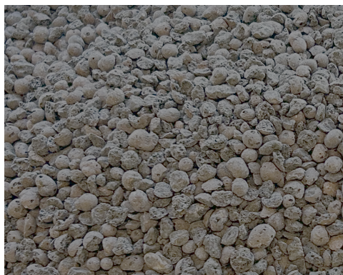
Figure 3.4: Argex 4/8 (coarse aggregates)
