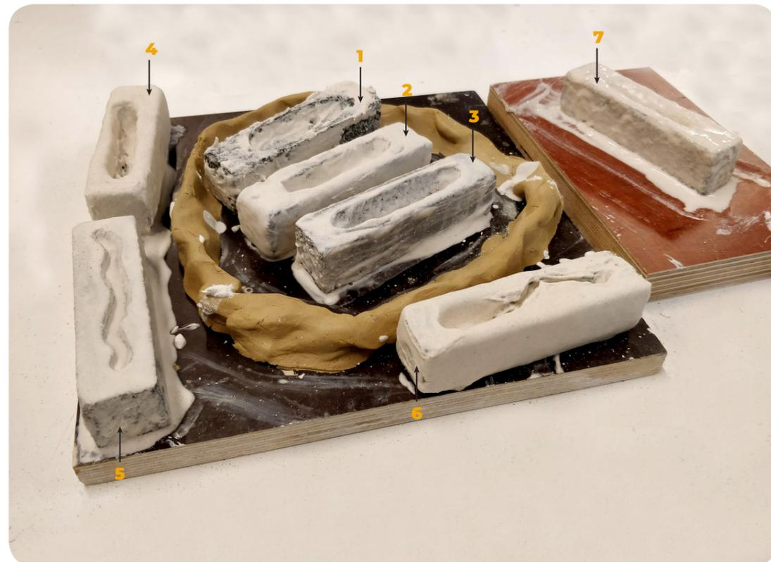
Fig. 06.3 a: Different consistencies of crystal cast tested on top of 3D printed test bar
