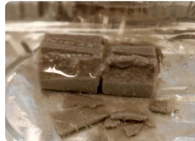
Fig. 06.5 h: No reaction of water to the strength of Anorganik binder system
