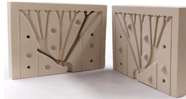
Fig. 07.2 a: 3D printed mould at 1:20 scale
