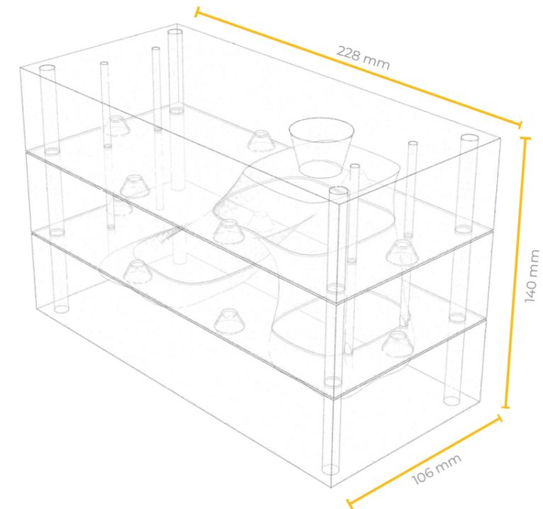
Fig. 07.1 f: Mould of Geometry 2 at scale 1:3
