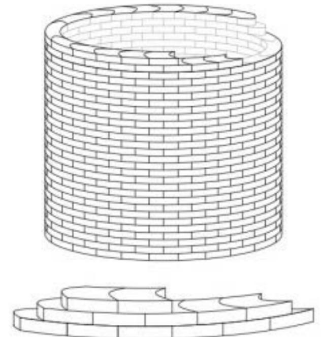
Fig. 03.8 b Atocha memorial adhesively bonded facade system (F. Oikonomopoulou, T. Bristogianni, et al., Interlocking cast glass components, Exploring a demountable dry-assembly structural glass system 2018)
