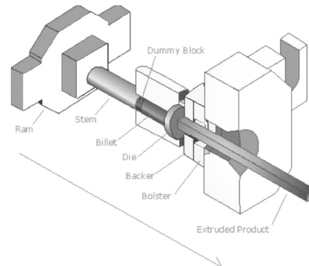
Fig 03.2 d : General process of Extrusion of any material
