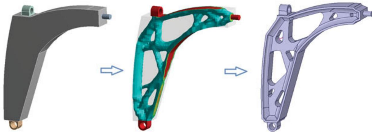
Fig. 03.7 d Topology Optimization of a Automotive part done using Ansys
