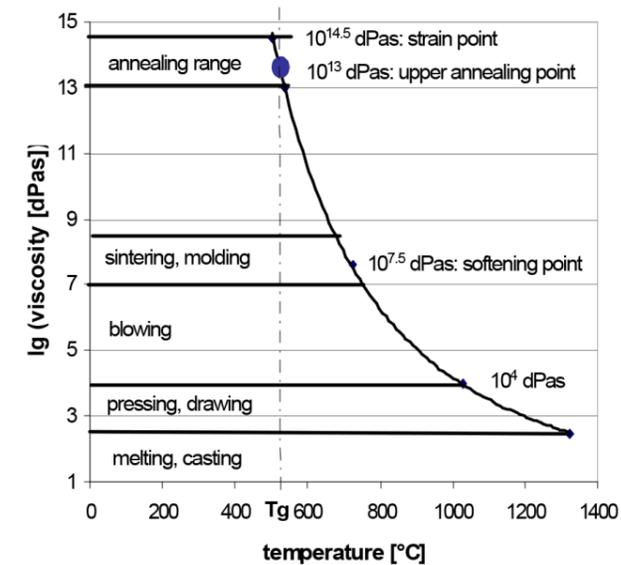
Fig. 03.4 c: Relation of Viscosity as a function of temperature (SchottAG 2004)
