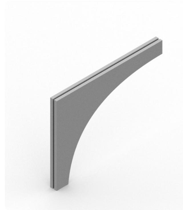
Fig. 05.2 u: New split geometry with 200 thk member and 100 thk gap in between the 2 geometries
