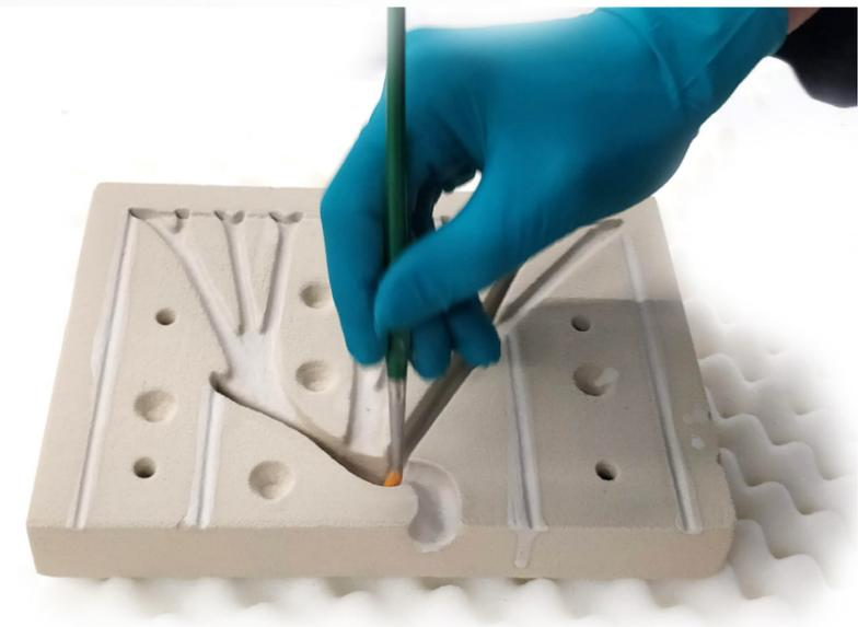
Fig. 07.2 b: Applying a coating of crystal cast for smooth finish of glass using a paint brush
