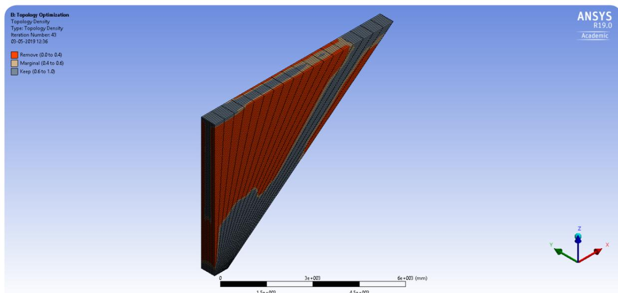
Fig. 05.2 j: Isometric view illustrating the material that is completely removed in red.
