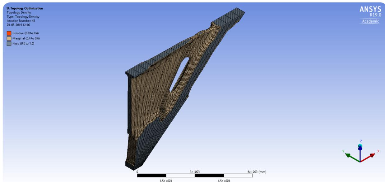
Fig. 05.2 i: Isometric view of the optimized geometry
