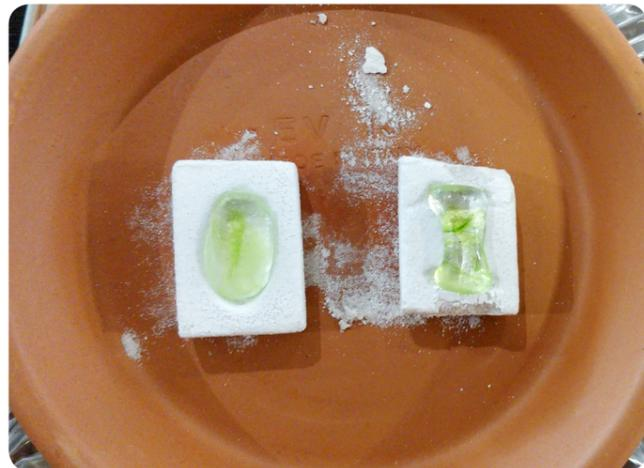
Fig. 06.6 d: Casted glass piece in boron nitride coated moulds
