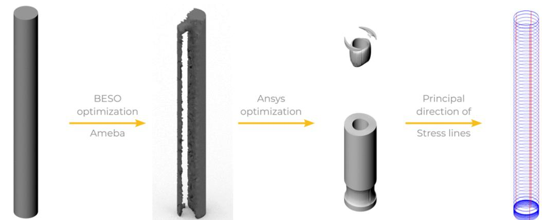
Fig. 05.2 b: Optimization of a straight column & Stress lines
