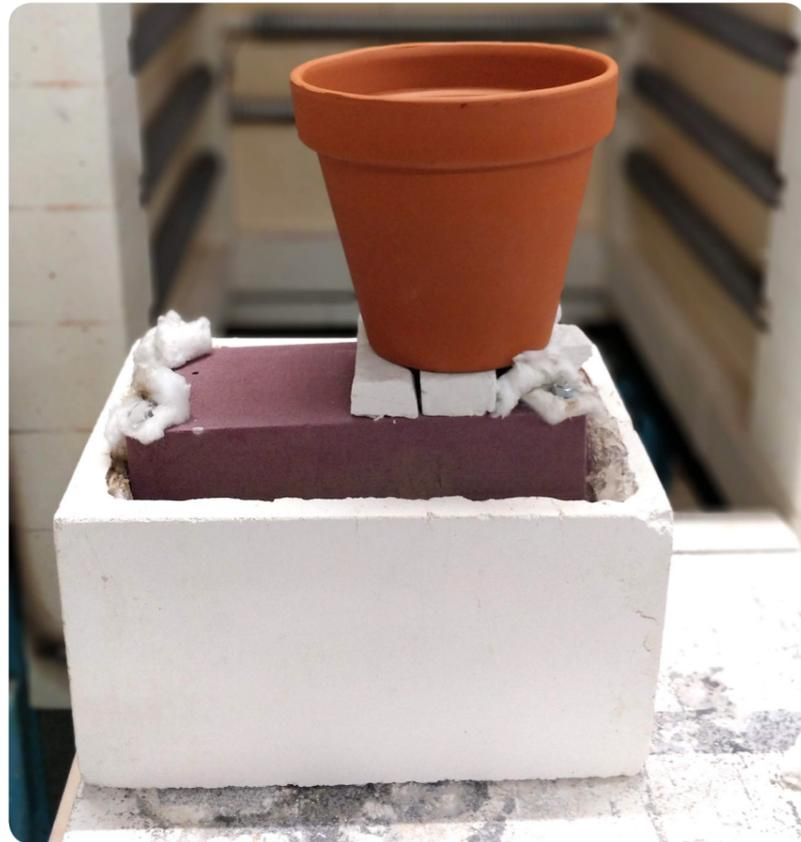
Fig. 07.2 p: Final setup of mould inside the furnace
