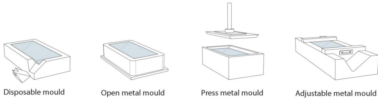
Fig. 03.5 a: Illustration of the most common mould types by F. Oikonomopoulou (F. Oikonomopoulou, et al. 2018)
