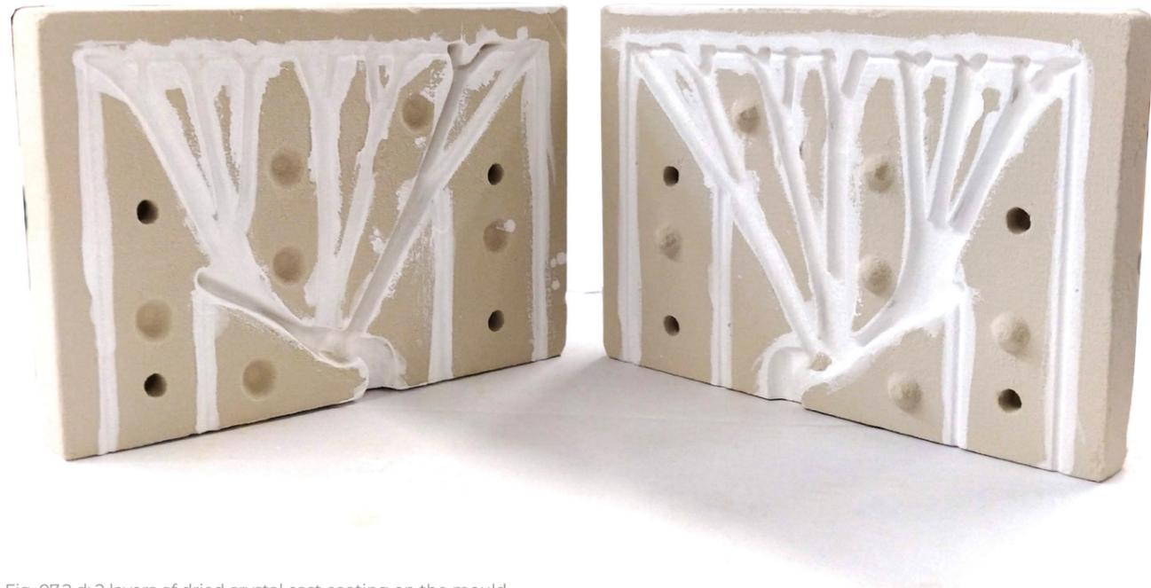
Fig. 07.2 d: 2 layers of dried crystal cast coating on the mould
