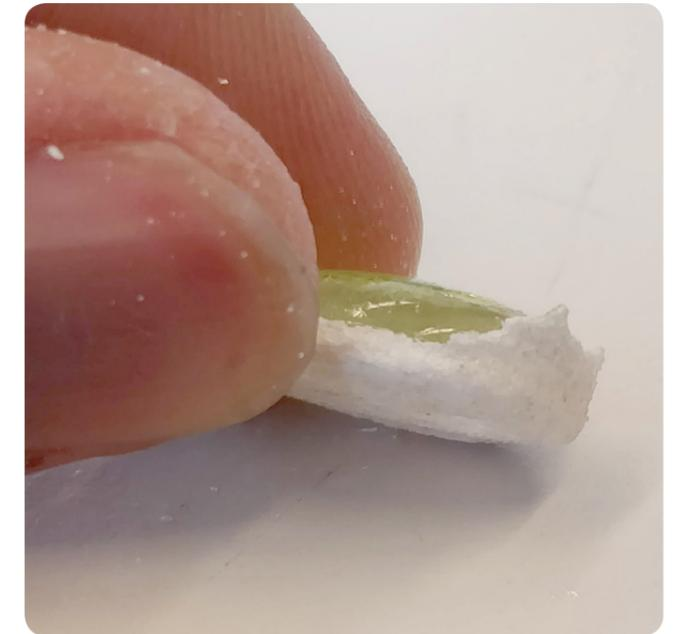
Fig. 06.7 f: Mold mix 6 coating being stuck to the glass piece
