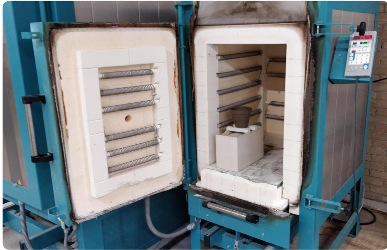
Fig. 07.2 l: Specimen being put inside the kiln- Helmut Rohde (model no. ELS 200 S)
