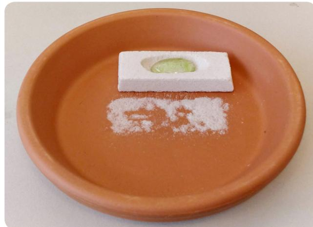
Fig. 06.5 f: Binder disintegration at the bottom of the CHP mould
