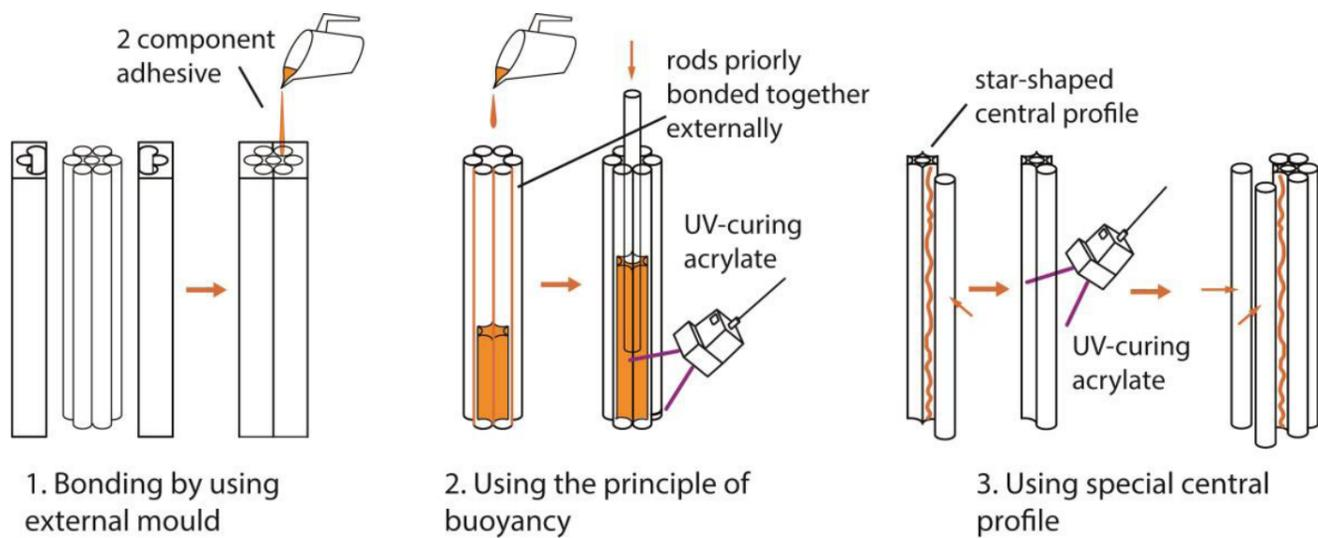
Fig. 03.3 n: Explored techniques for bonding rods together
