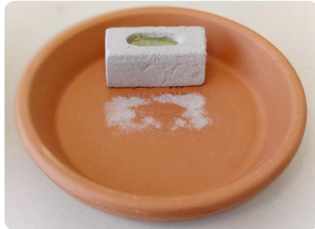
Fig. 06.5 e: Binder disintegration at the bottom of the Anorganik mould
