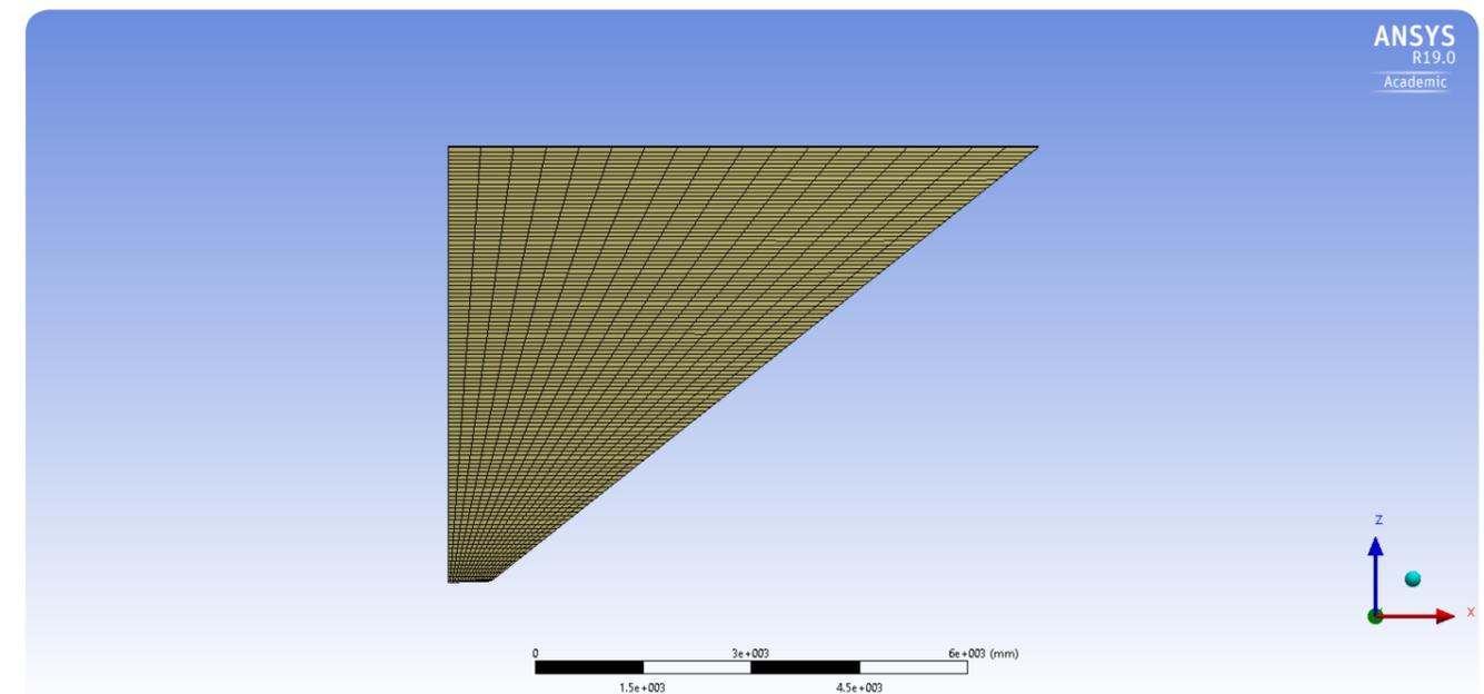
Fig. 05.2 g: Mesh size and distribution of the geometry
