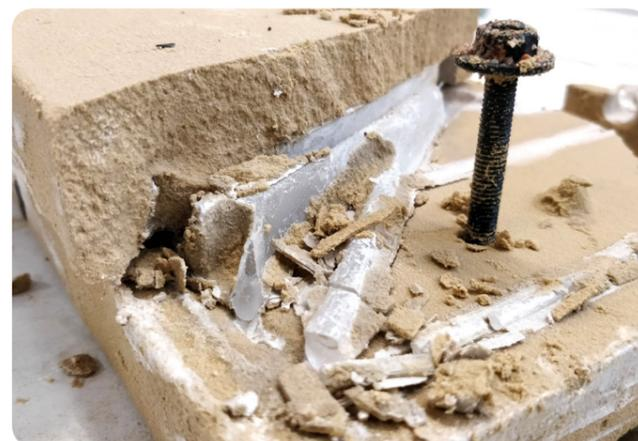
Fig. 07.3 c: On breaking the mould, half casted pieces of glass can be observed. Also, nuts &amp; bolts are burnt and are fused together.
