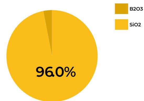
96% silica is very similar to fused silica except 3% of boron oxide is added as stabilizer.
