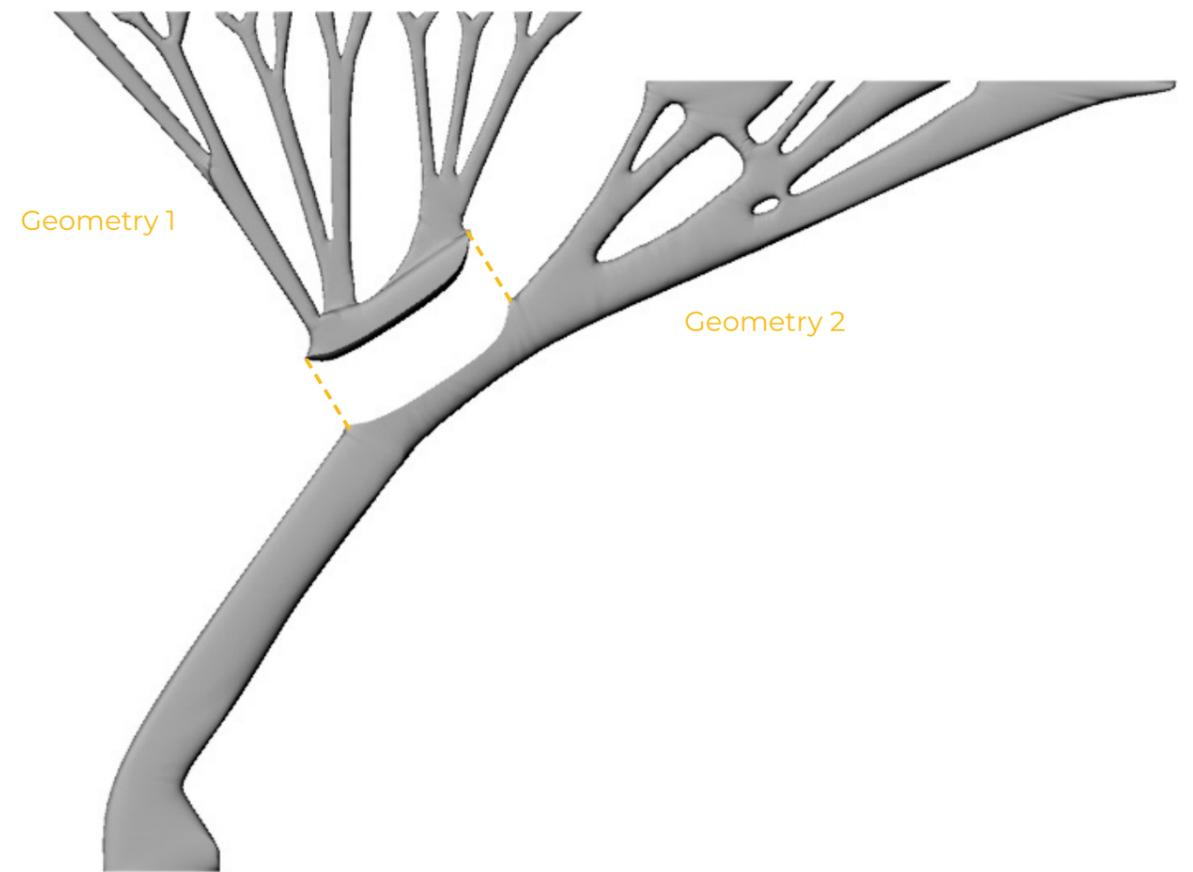
Fig. 05.2 ze: Final splitted Geometry for fabrication
