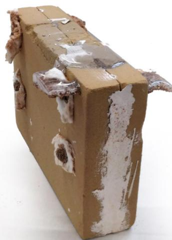
Fig. 07.3 b: Sand mould upon removal from the setup could still sustain its own weight along with the casted glass piece
