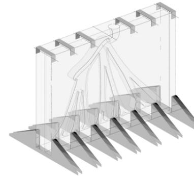
Fig. 08.1 f: Clamping moulds together using steel clamps
