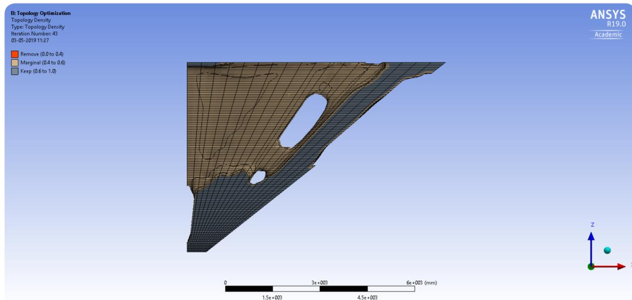
Fig. 05.2 h: Front view of the Optimized Geometry
