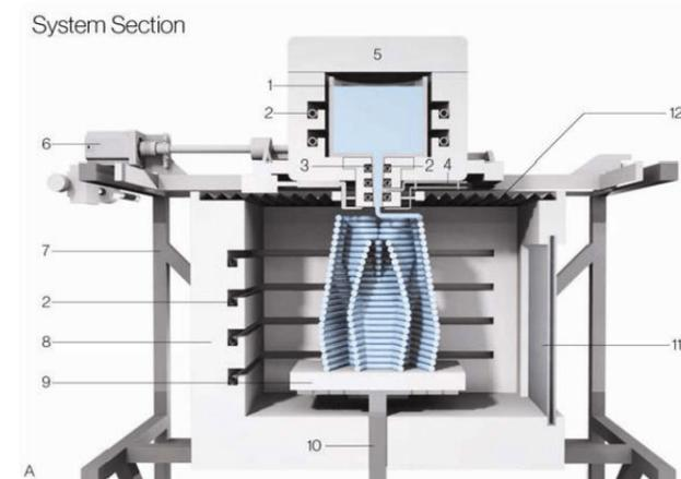
Fig. 03.2 h: G3DP dual heated chamber Glass printer by MIT 1. crucible, 2. heating elements, 3. nozzle, 4. thermocouple, 5. removable feed access lid, 6. stepper motors, 7. printer frame, 8. print annealer, 9. ceramic print plate, 10. z-driven train, 11. ceramic viewing window, & 12. insulating skirt
