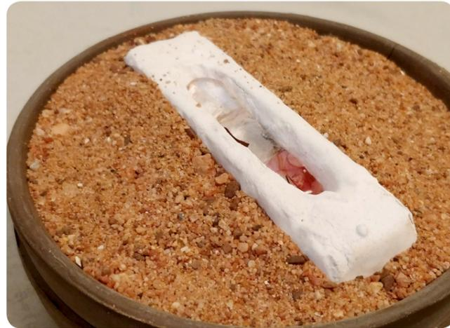
Fig. 06.3 g: Casted glass piece in specimen 2
