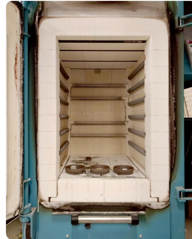
Fig. 06.4 b: Helmut Rohde kiln used for the experiment
