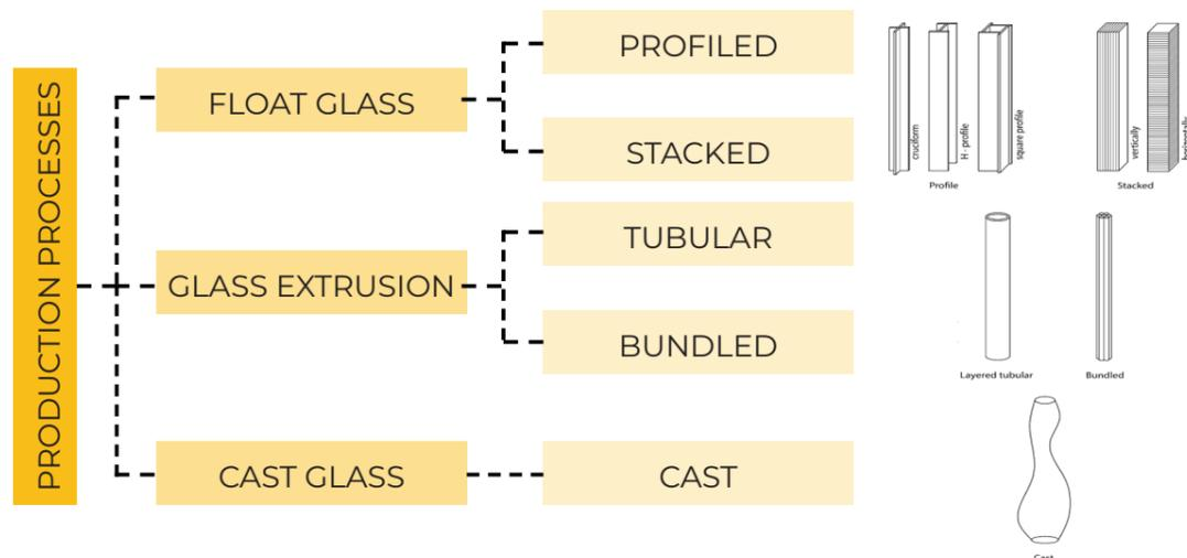
Fig. 03.3 f: Classification of columns based on production process
