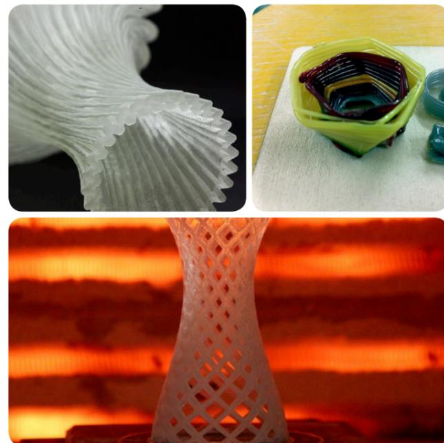
Fig. 03.2 g: 3D printed Glass prototypes by Micron 3DP (Micron3dp 2019) (Simon 2015)
