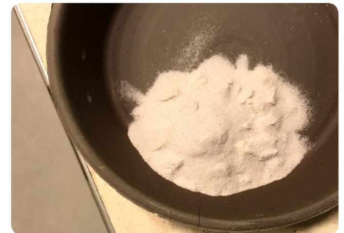
Fig. 06.2 d: Total disintegration of binder leaving a heap of sand
