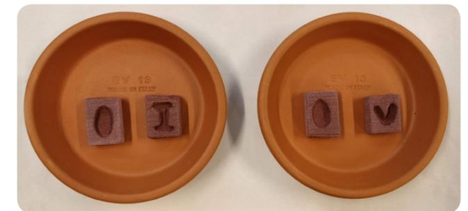
Fig. 06.6 b: Manually carved impressions in CHP binded sand mould
