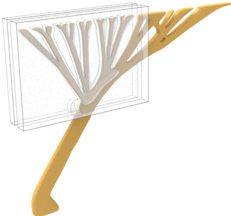
Fig. 07.1 b: Mould design with respect to geometry.
