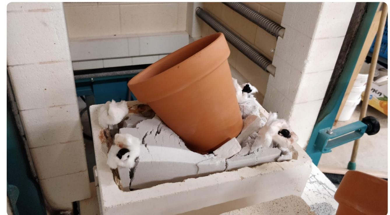
Fig. 07.3 e: Failure of the mould due to weight of the earthen pot and glass
