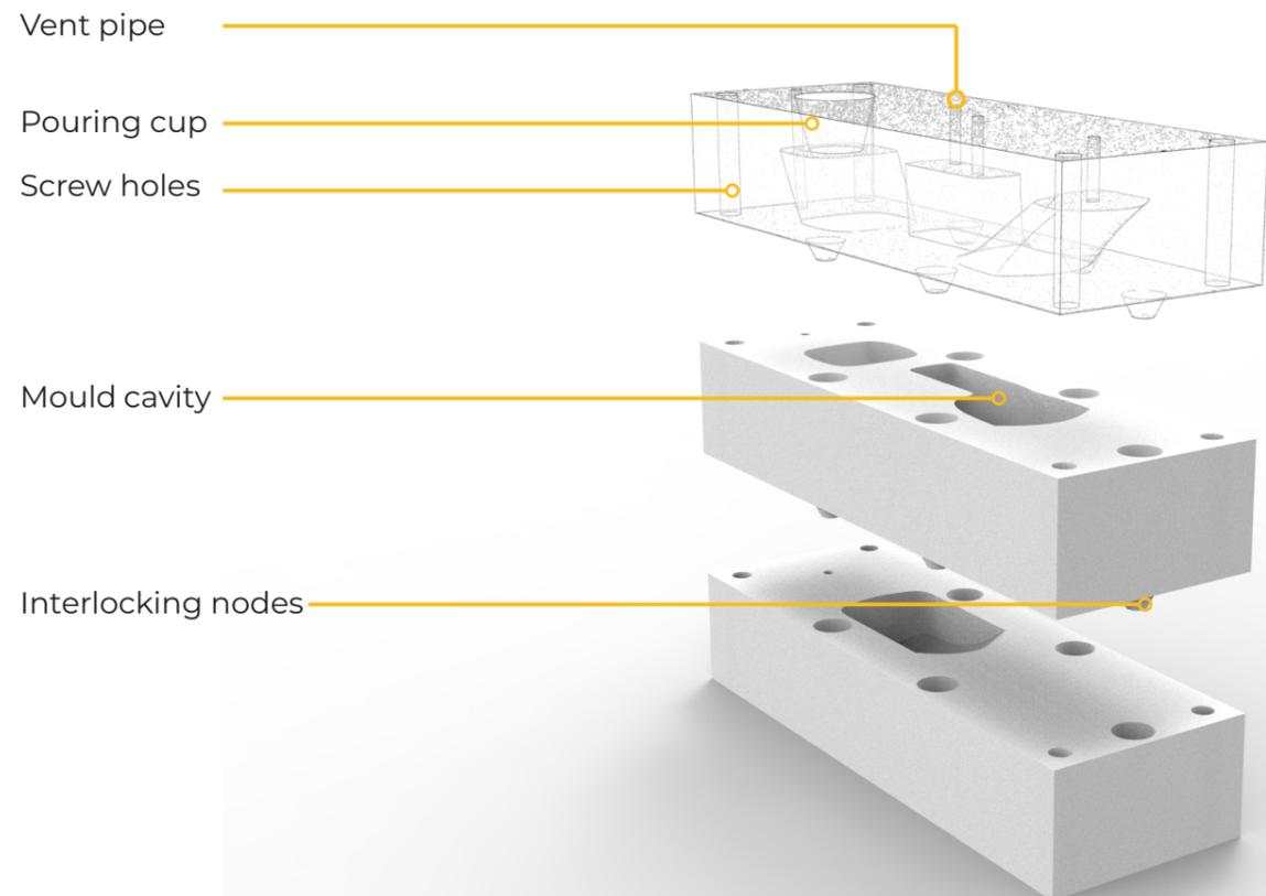
Fig. 07.1 i: Final mould design for prototyping
