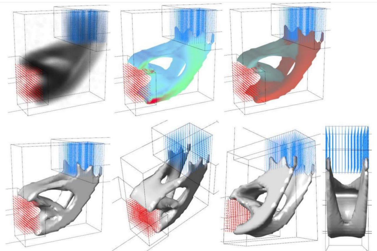
Fig. 03.7 c 3 Dimensional topology optimization using millipede (Michalatos & Kajijima, n.d.)
