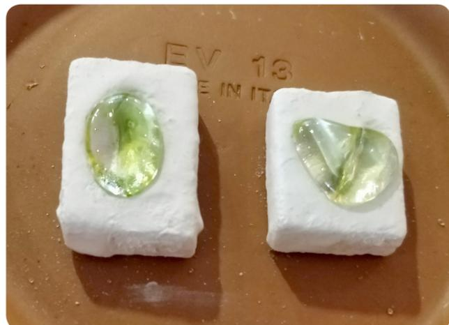
Fig. 06.6 e : Casted glass piece in crystal cast coated moulds
