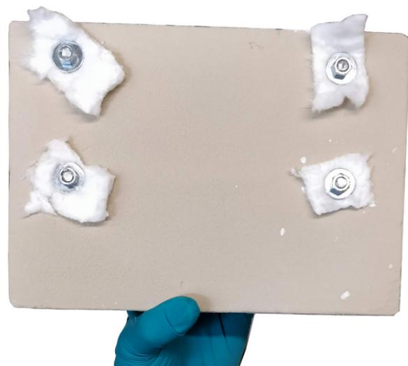
Fig. 07.2 h: putting blanket around screws to avoid sticking of glass around screws during breakage of mould or overflow of glass.
