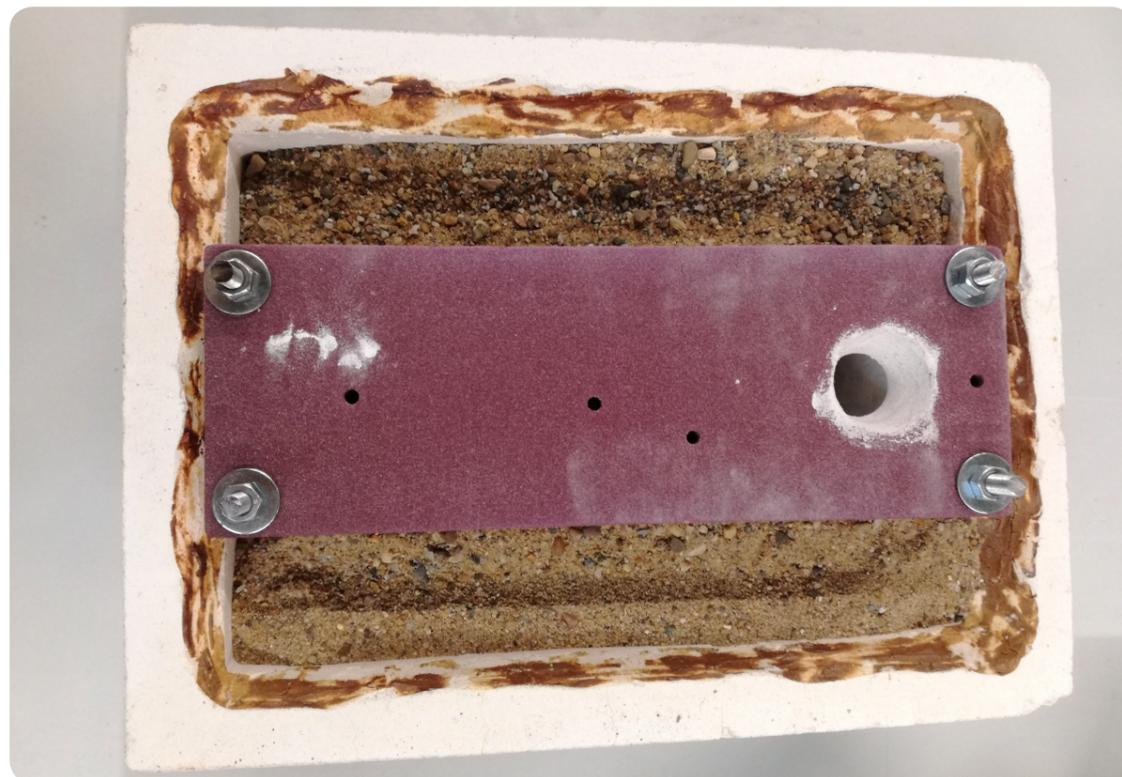
Fig. 07.2 u: Crystal cast coated mould prepared for casting inside the kiln
