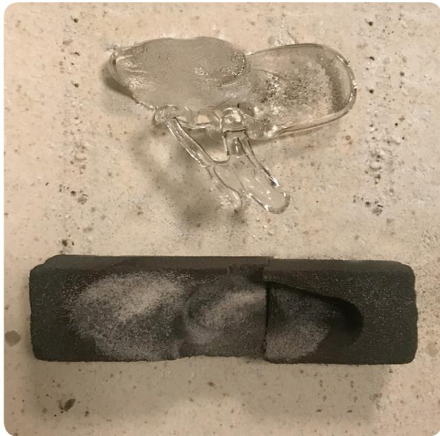
Fig. 06.1 i: Surface chills observed on the contact area
