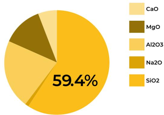
Aluminosilicate glasses have alumina (Al<sub>2</sub>O<sub>3</sub>) in their composition. This type of glass is very similar to Borosilicate type but offer better resistance to temperature fluctuations and chemicals.
