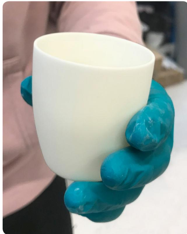
Fig. 06.1 c: High alumina crucible
