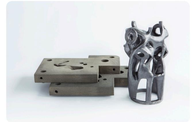
Fig. 03.6 c: Metal casted node in a 3D printed sand mould designed by Arup (Galjaard 2017)
