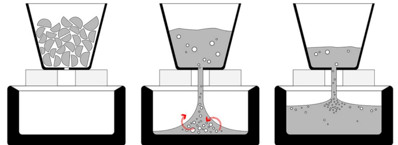
Fig. 03.2 o: Process of Kiln Casting using terracotta pots for melting the broken glass pieces which pours down in the mould
