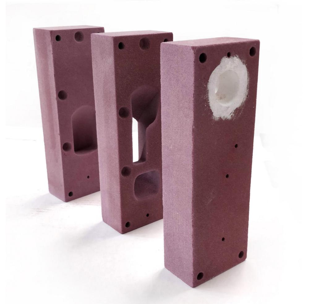
Fig. 07.2 s: 3D printed mould at 1:3 scale for prototyping
