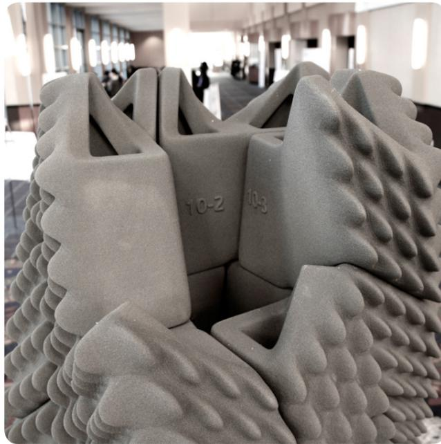
Fig. 03.6 g: Hollow inter lockable sand printed pieces for dry assembly (Rael 2018)
