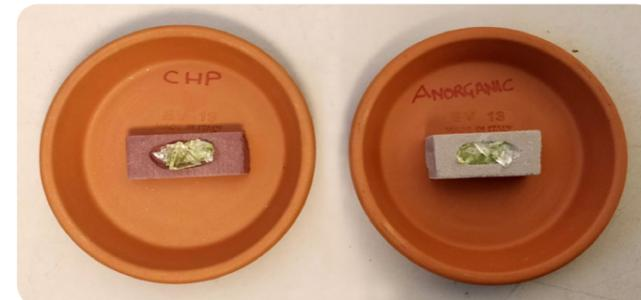
Fig. 06.5 a: Kiln casting of glass piece in manually carved impression in sand mould
