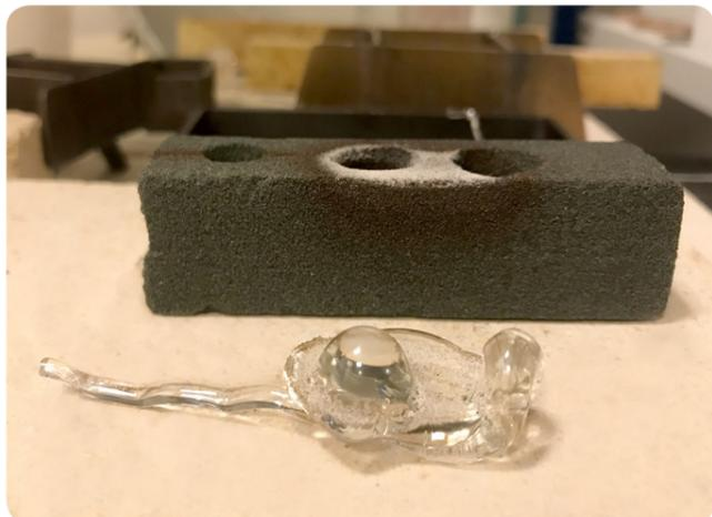
Fig. 06.1 j: Casted glass piece, specimen 2
