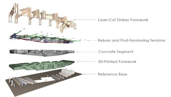
Fig. 03.6 j: Framework for casting concrete slab segment with provision for post-tensioning tendons.(The Smart Slab n.d.)
