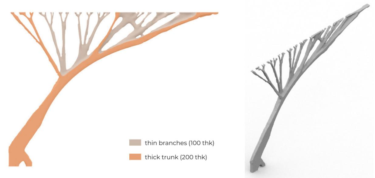
Fig. 05.2 zc: Generalization of thickness of the optimized geometry
