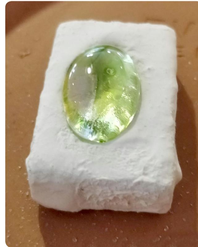
Fig. 06.6 h: Clear optical quality of glass in crystal cast coated mould
