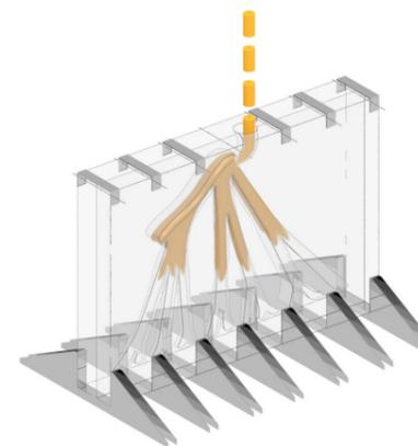
Fig. 08.1 g: Pouring of molten glass in preheated mould
