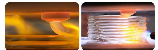
Fig. 03.2 j: View of the Kiln chamber while printing in G3DP. (Simon 2015)
