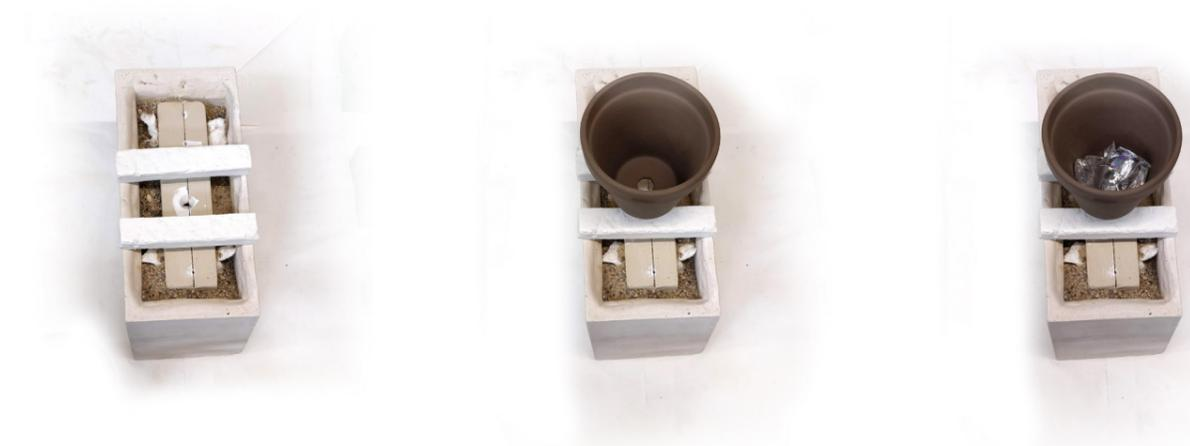
Fig. 07.2 k: Placing an earthen pot on top of mould to allow glass to melt in the pot and flow inside the sand mould.
