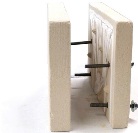
Fig. 07.2 e: clamping on moulds together using M8 bolt & nut
