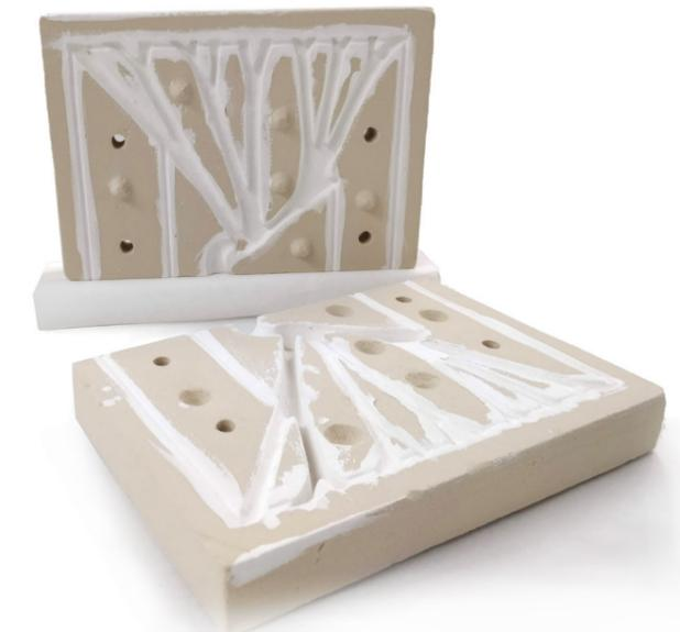
Fig. 07.2 c: 2 layers of dried crystal cast coating on the mould
