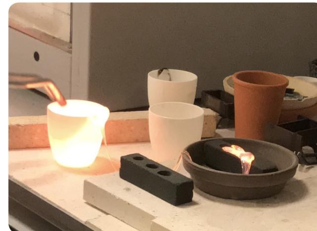
Fig. 06.1 f: Glass hot poured in the cavity of first specimen
