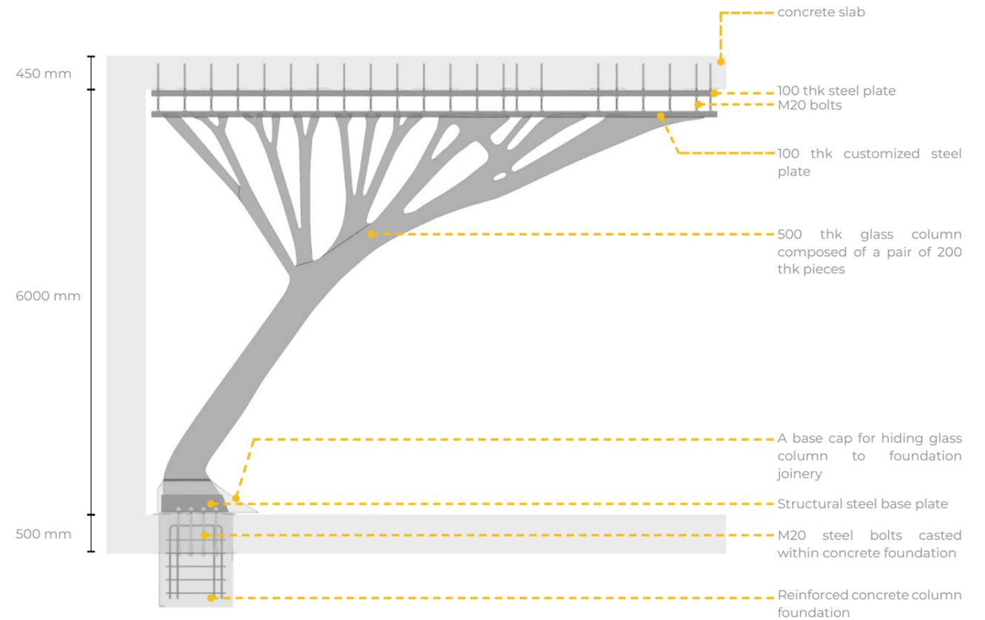
Fig. 08 b: Final assembly of Glass Column
