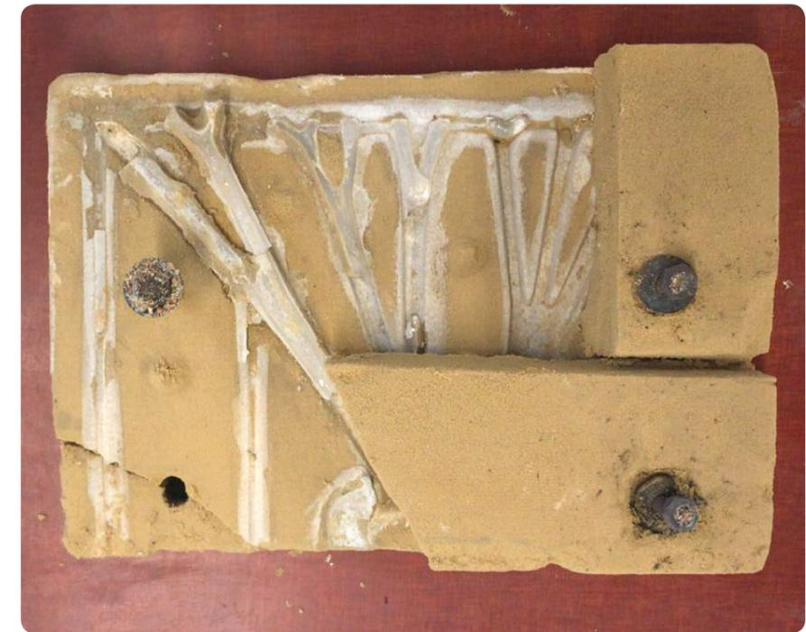
Fig. 07.3 i: Anorganik binder system with artificial sand as mould showcasing the small casted glass pieces inside the mould
