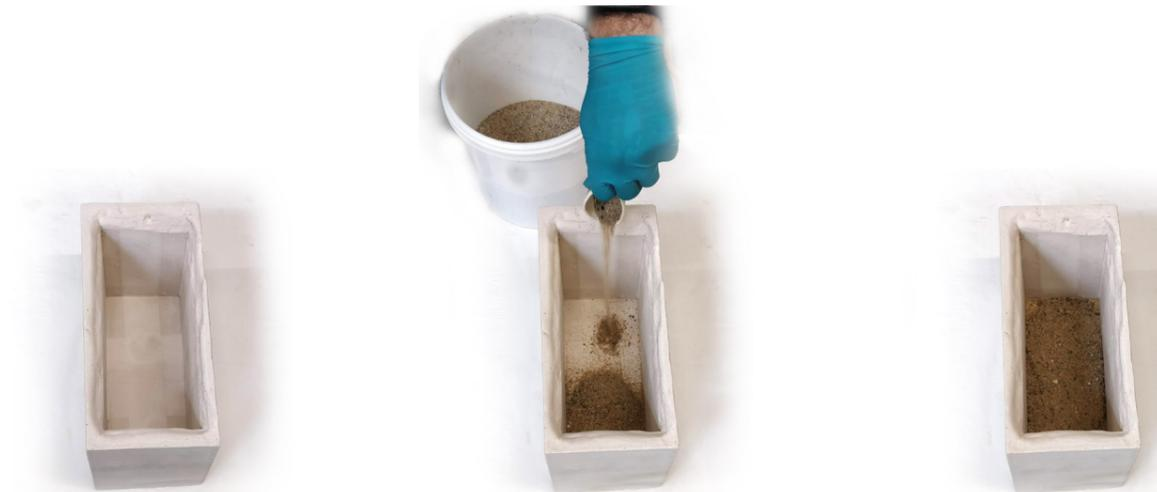
Fig. 07.2 i: setting up a bed of coarse sand before placing sand mould inside crystal cast mould.
