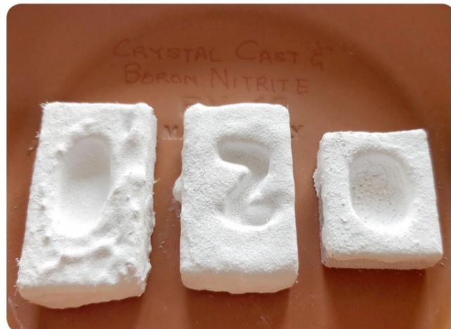
Fig. 06.7 c: Specimens coated with crystal cast and then boron nitride
