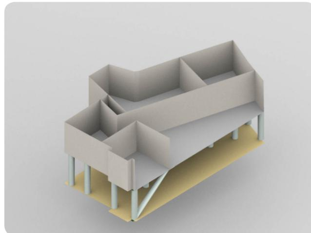
Fig. 05.2 d: Slanted column transferring the load to the periphery
