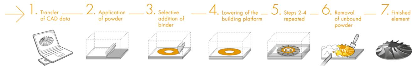
Fig. 03.6 a: Illustration of step by step procedure of sand casting of metal by (Voxeljet 2018).
