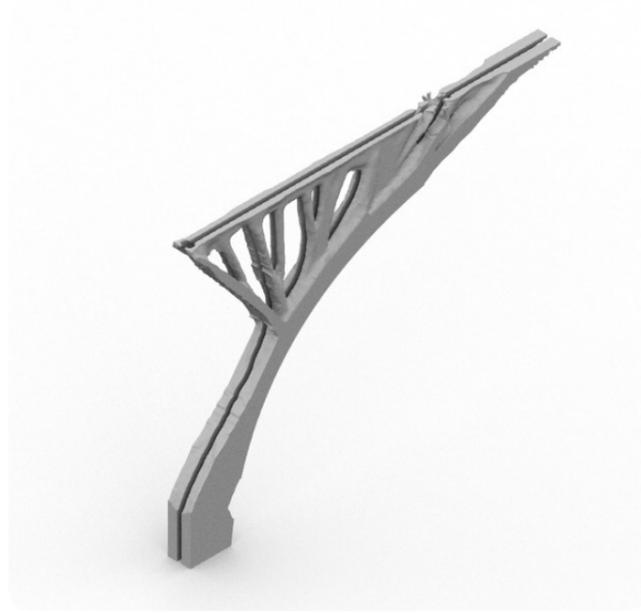
Fig. 05.2 w: Second Optimization of split geometry
