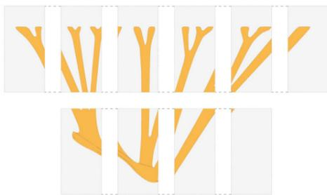
Fig. 08.1 b: Division of geometry on basis of printer bed size
