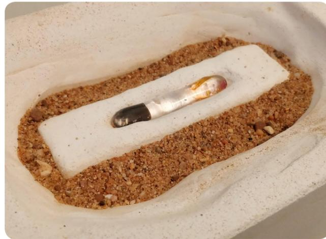
Fig. 06.3 f: Casted glass piece in specimen 1
