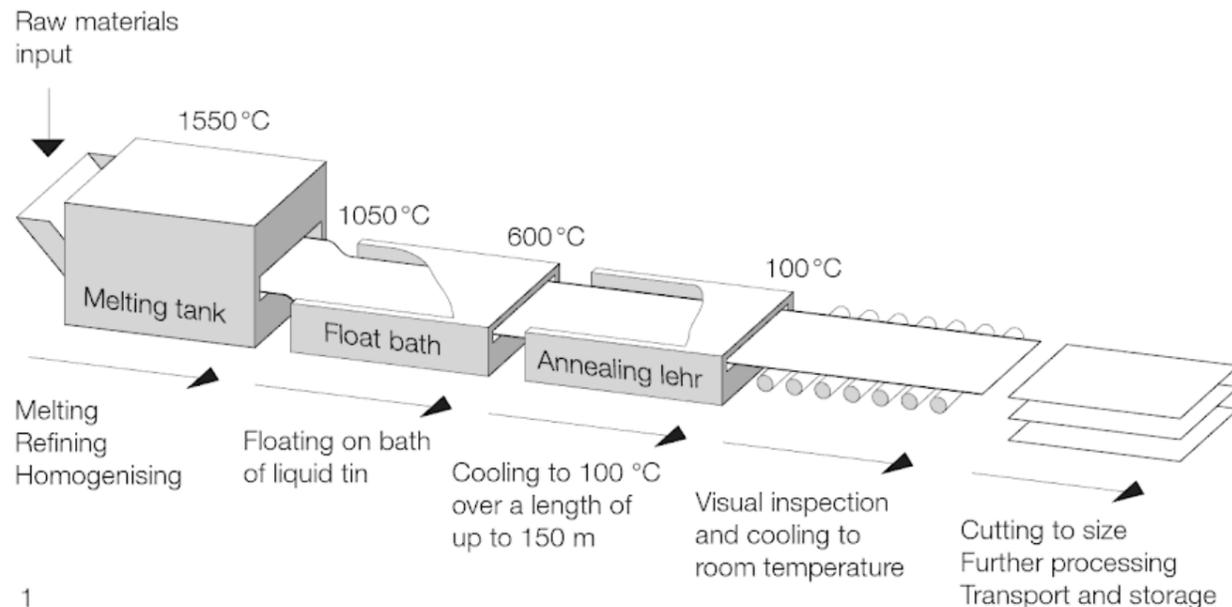
Fig 03.2 b : Float Glass Process from Melting to Annealing and finally post processing
