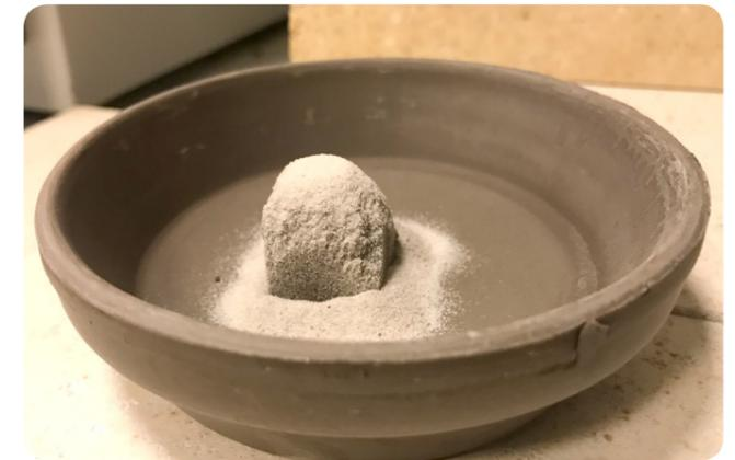
Fig. 06.2 c: Disintegration of binder resulting in loose sand around
