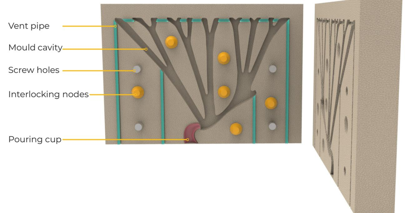
Fig. 07.1 d: Final mould design for prototyping
