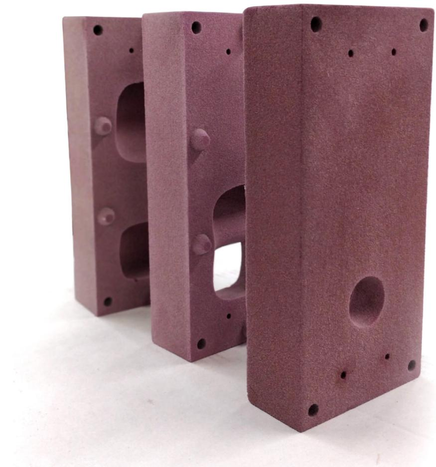
Fig. 07.2 o: 3D printed mould at 1:3 scale for prototyping
