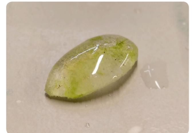
Fig. 06.5 j: Casted glass piece in CHP binder system
