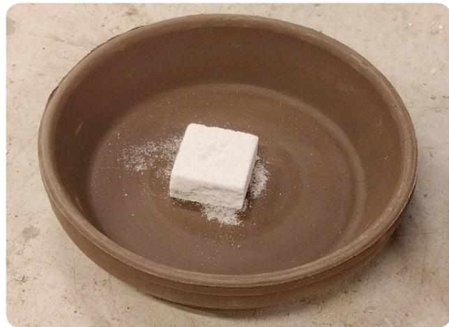
Fig. 06.4 d: CHP binder system after exposure to heat at 900 degree
