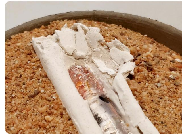
Fig. 06.3 i: Lose of strength by the mould after casting process
