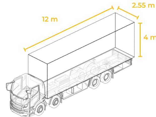
Fig. 05.1 a: Maximum permissible dimension of a truck on German roads
