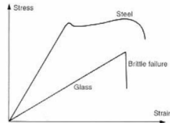
Fig 03.1 f: Stress and Strain curve of Glass V/S Steel (sahol hamid 2007)
