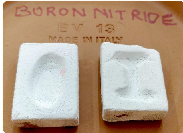
Fig. 06.6 f: Boron nitride coated moulds before experiment
