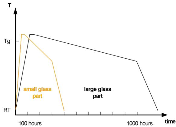
Fig. 03.4 b: Small v/s Large glass piece in regards to annealing time (SchottAG 2004)
