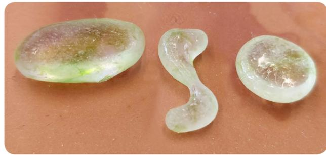
Fig. 06.7 h: Casted glass pieces with crystal cast and boron nitride coating
