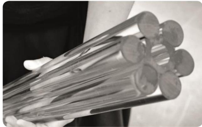
Fig. 03.3 m: Final prototype of bundled glass column
