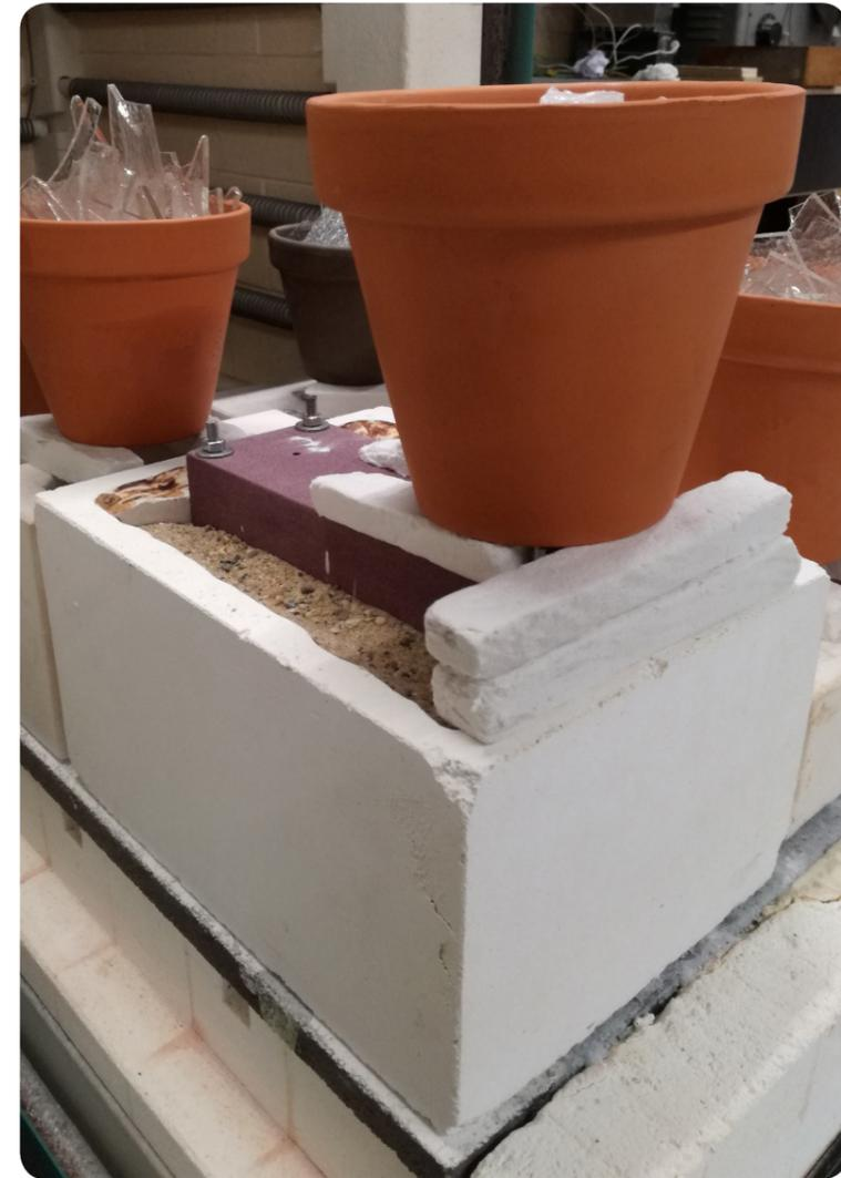
Fig. 07.2 v: Crystal cast coated mould prepared for casting inside the kiln
