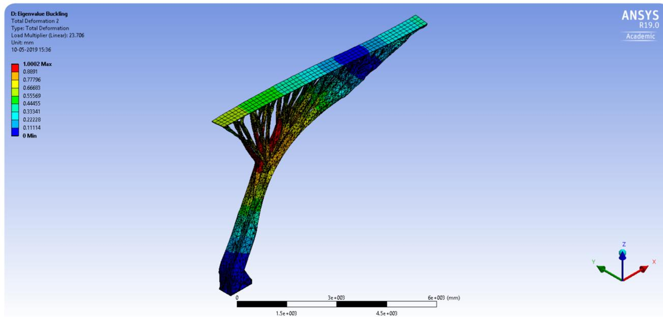
Fig. 05.2 zb: Buckling Analysis along x axis.
