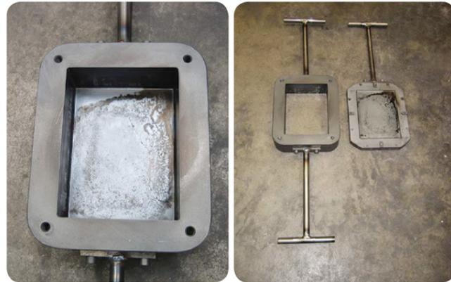
Fig. 03.2 l: Reusable Steel moulds for casting glass by Poesia Company
