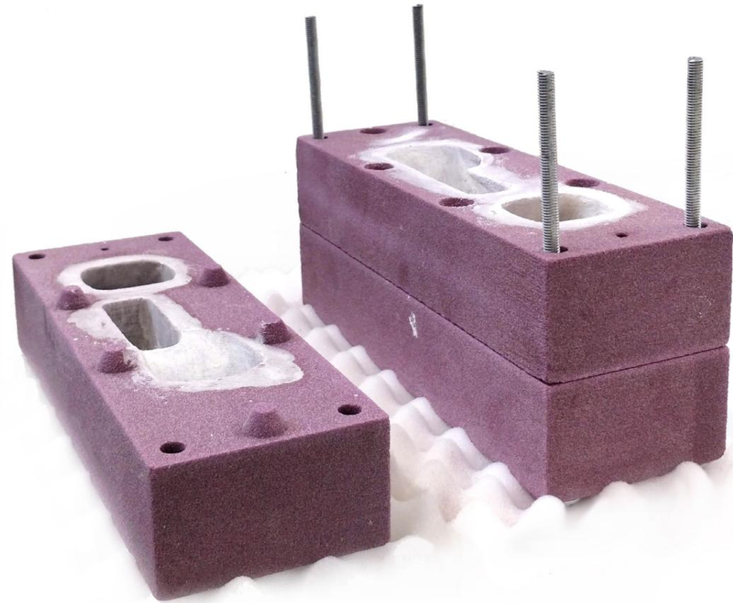
Fig. 07.2 t: Crystal cast coated mould prepared for casting inside the kiln
