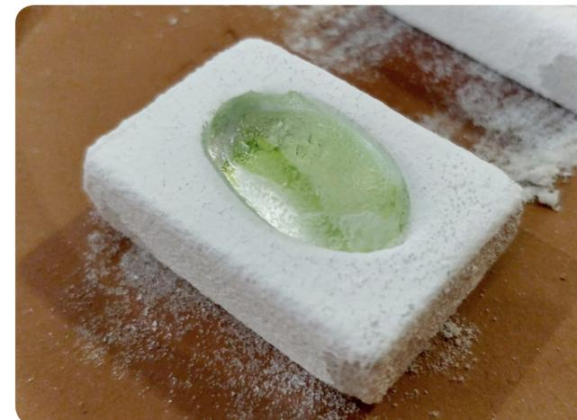
Fig. 06.6 i: Dusky optical quality of glass in boron nitride coated mould
