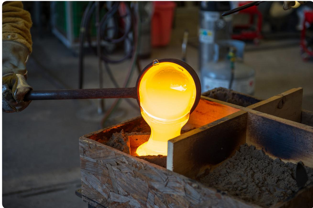
Fig. 03.2 m: Casting of molten Glass in a steel mould surrounded by sand to avoid expansion of mould due to pressure
