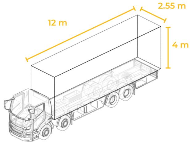
Fig. 08.2 a: Maximum permissible dimension of a truck on German roads
