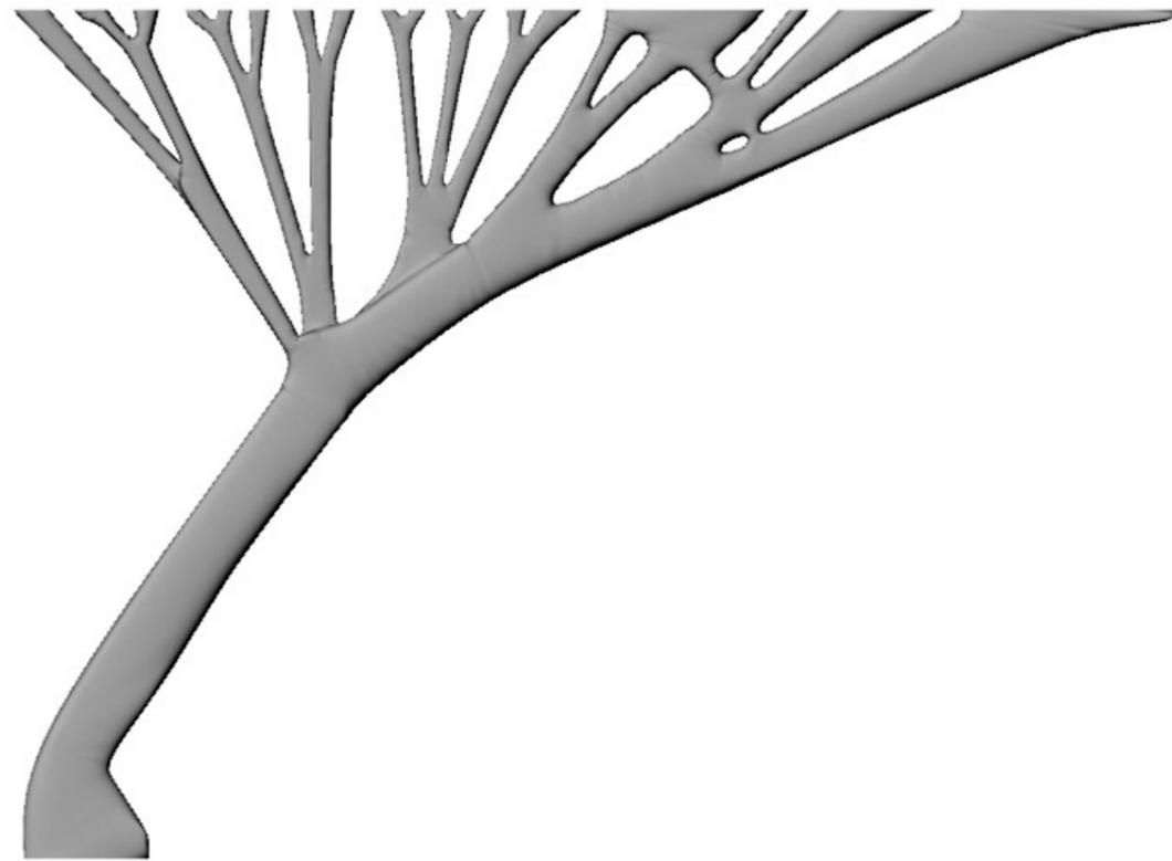
Fig. 05.2 zd: Final Optimized Geometry for fabrication
