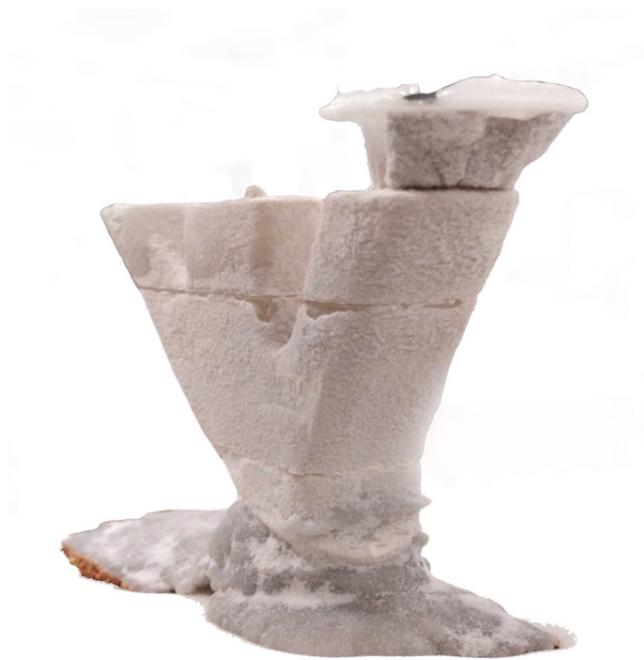
Fig. 07.3 g: Casted geometry after removal from sand mould
