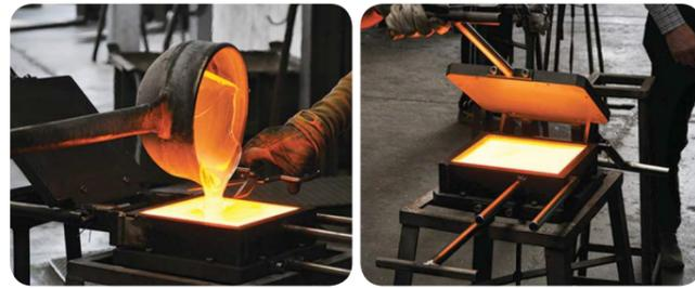
Fig. 03.2 k: Casting of Soda-lime glass bricks by Poesia Company
