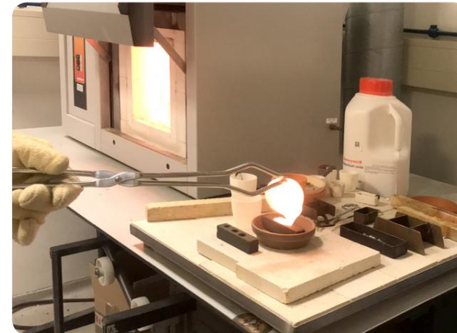
Fig. 06.1 e: Hot pouring of glass on top of first specimen
