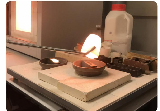
Fig. 06.1 g: Hot pouring of glass for second specimen
