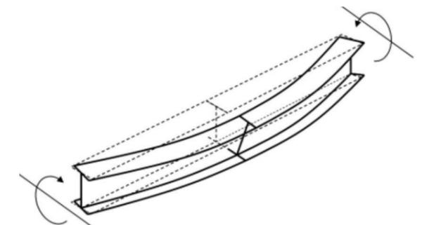
Fig. 03.3 d: Torsional Buckling of a column
