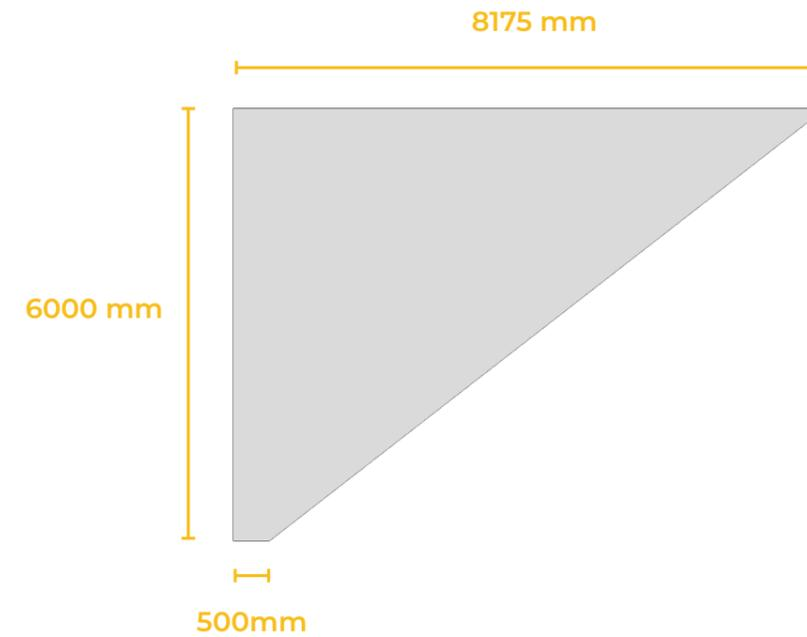
Fig. 05.2 f: Dimension of the new column to be optimized
