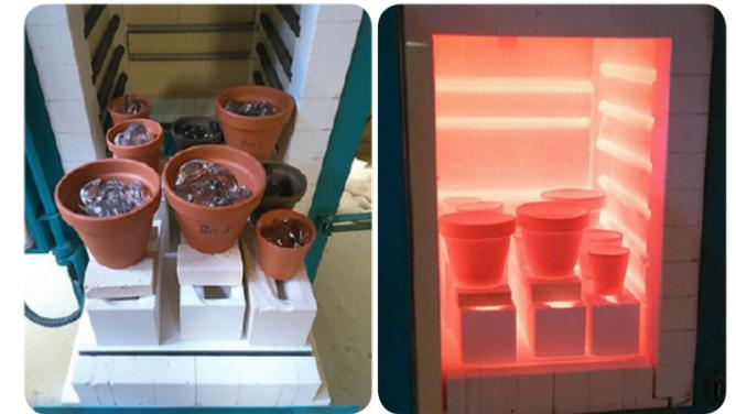
Fig. 03.2 n: Kiln casting of glass objects at TU Delft glass lab
