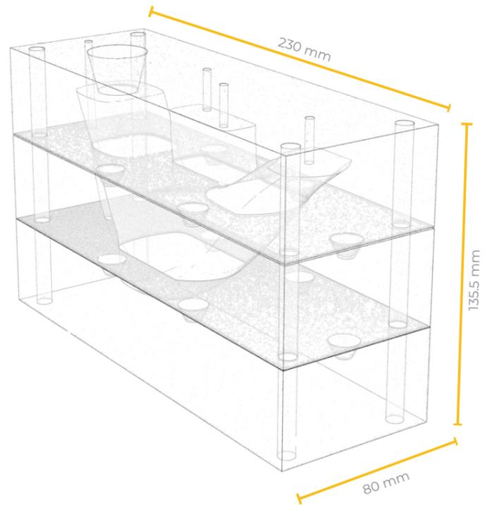
Fig. 07.1 h: Mould of Geometry 3 at scale 1:5
