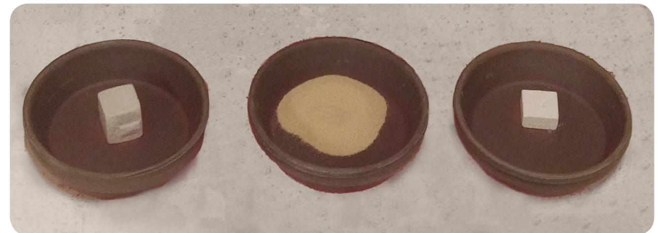
Fig. 06.4 c: Specimens behavior on exposure to heat at 500 degree Celsius
