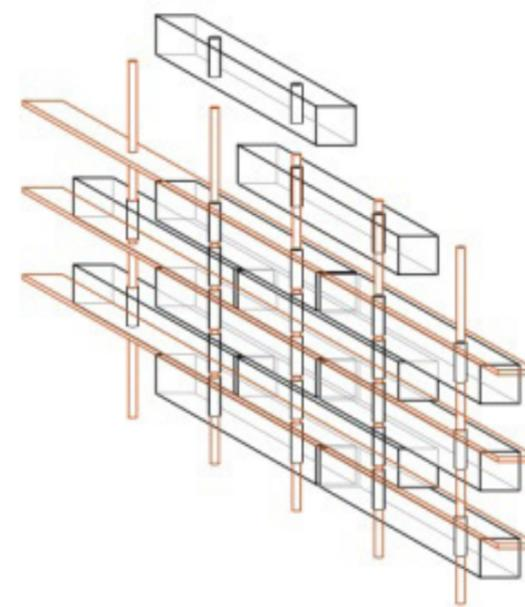
Fig. 03.8 a Optical House facade illustration showing the substructure (F. Oikonomopoulou, T. Bristogianni, et al., Interlocking cast glass components, Exploring a demountable dry-assembly structural glass system 2018)
