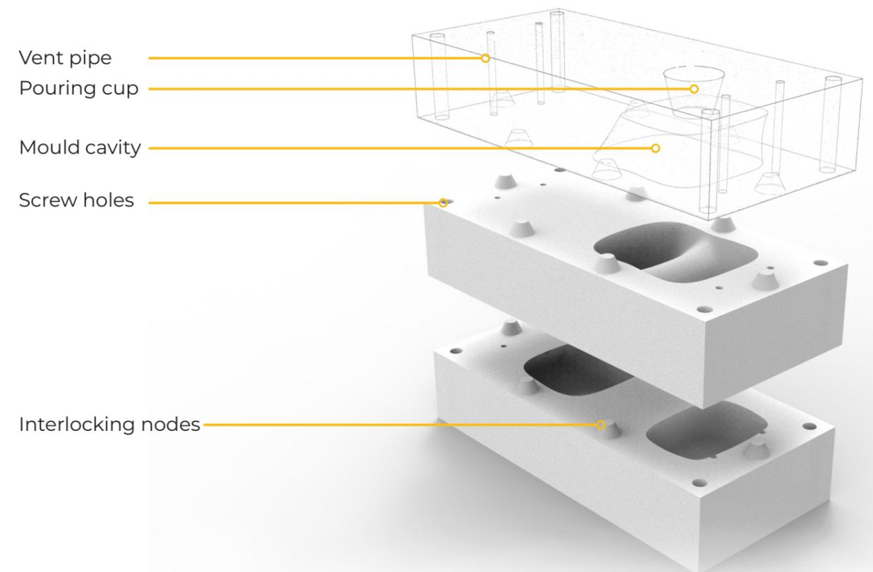
Fig. 07.1 g: Final mould design for prototyping
