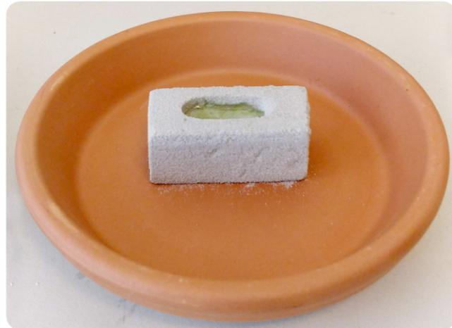
Fig. 06.5 c: Casted glass piece inside Anorganik binder system
