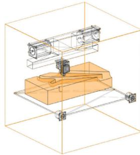
Fig. 08.1 c: Printing of sand mould
