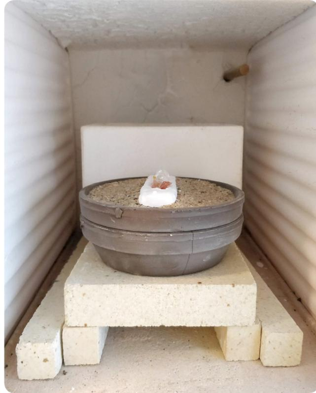
Fig. 06.3 d: Setting up of specimens inside the oven
