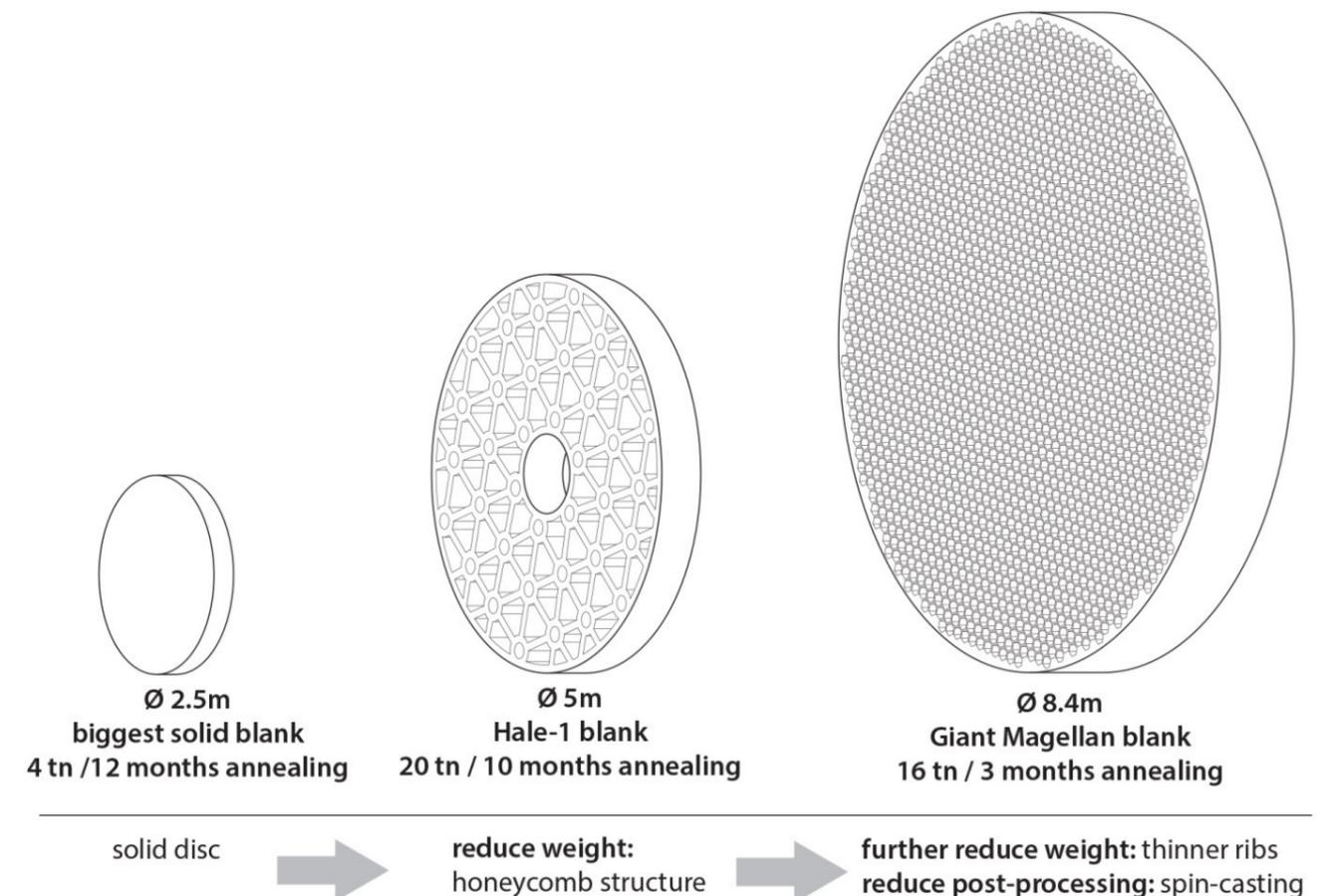
Fig. 03.4 d: Evolution of the cast mirror blanks in size due to smart geometry and manufacturing process (F. Oikonomopoulou, et al. 2018)
