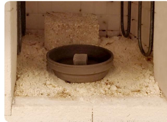
Fig. 06.2 a: Specimen tested for direct exposure to heat
