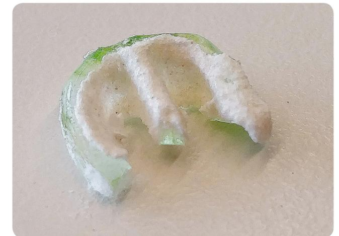
Fig. 06.7 g: Mold mix 6 coating being stuck to the glass piece
