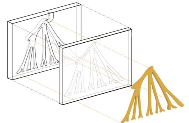
Fig. 08.1 i: Demoulding the casted glass geometry
