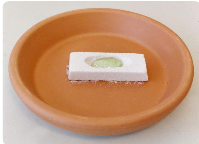
Fig. 06.5 d: Casted glass piece inside CHP binder system
