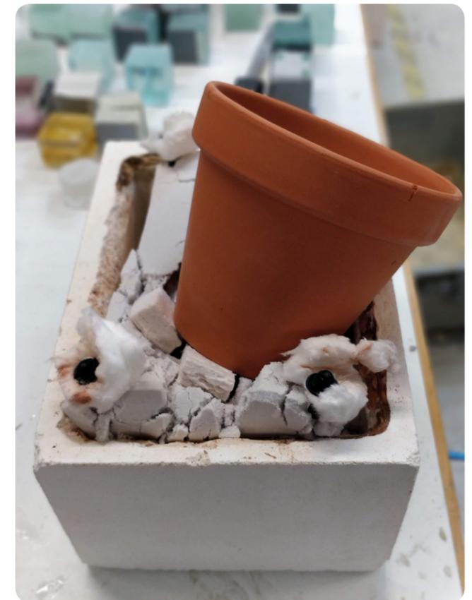
Fig. 07.3 d: Failure of the sand mould during the casting process
