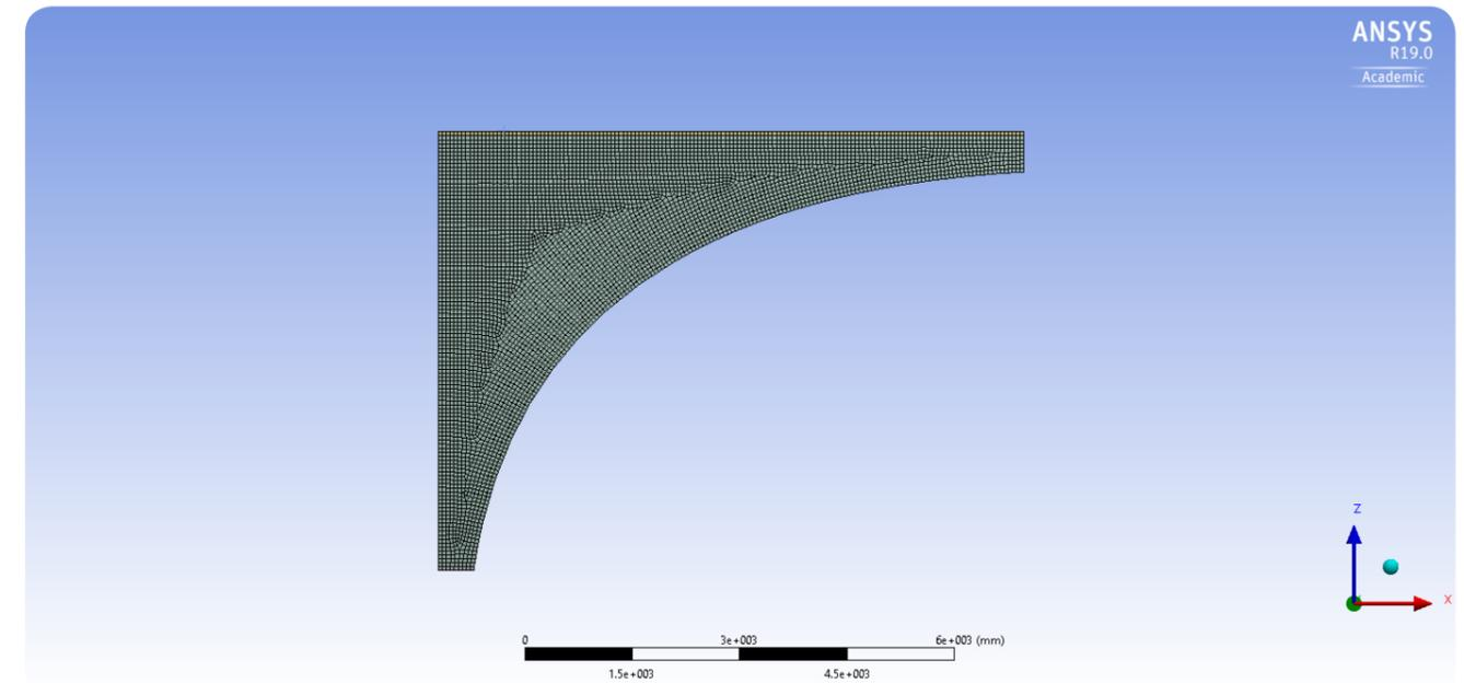
Fig. 05.2 n: Mesh size and distribution of the geometry
