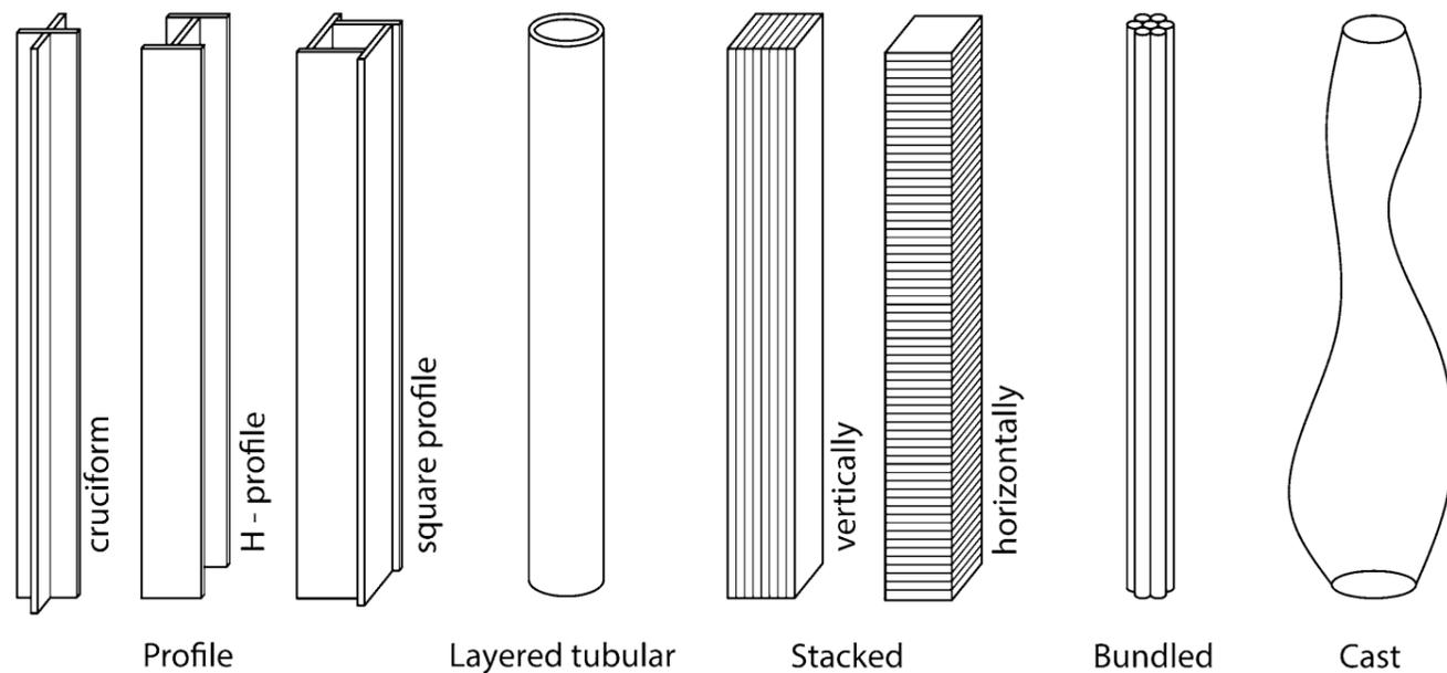
Fig. 03.3 e: 5 different types of columns defined by R. Nijse & E. ten Brincke
