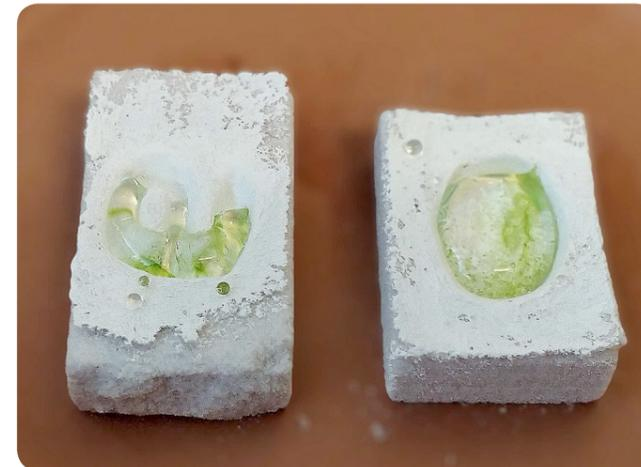
Fig. 06.7 d: Result of glass casted in mold mix 6 coated moulds
