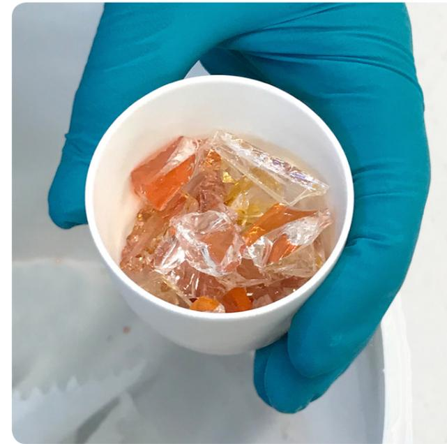
Fig. 06.1 d: Broken pieces of glass in crucible
