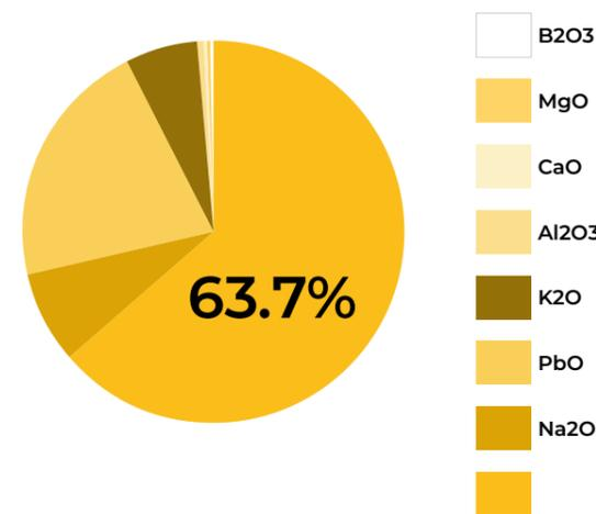
Borosilicate glass, also known as Pyrex, was invented by Corning Glass Works in 1915. It was developed to withstand high thermal shocks. The material has low thermal expansion coefficient. This makes it less prone to internal stress, hence would not fracture easily.
