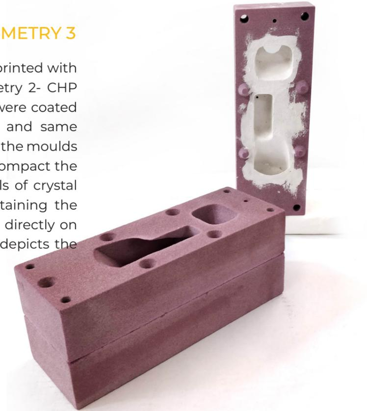
Fig. 07.2 r: 3D printed mould at 1:3 scale for prototyping
