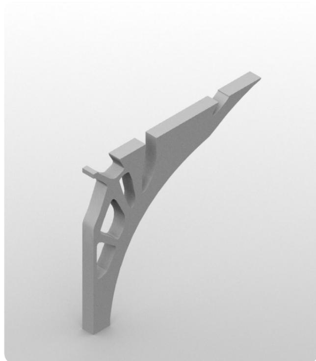
Fig. 05.2 p: Extrusion of silhouette of 1st optimized geometry
