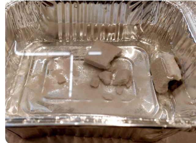
Fig. 06.5 g: Easy disintegration of CHP binder inside water
