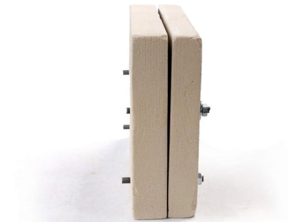
Fig. 07.2 f: clamping of mould together using M8 bolt & nut
