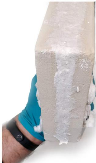
Fig. 07.2 g: sealing the seam between the mould pieces to avoid leakage of glass
