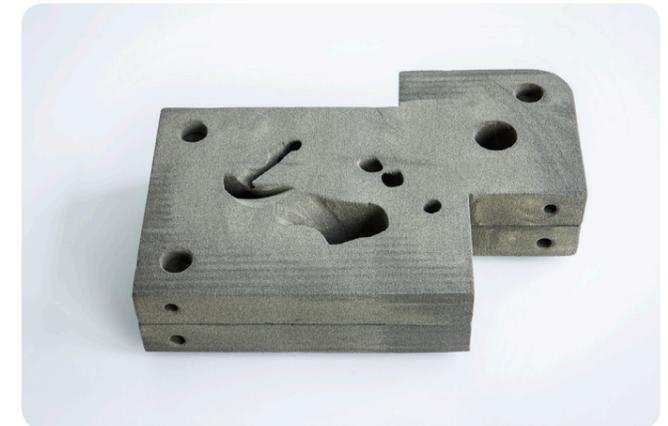
Fig. 03.6 d: 3D printed sand mould designed and fabricated by 3Dealise for casting a metal node (Galjaard 2017)
