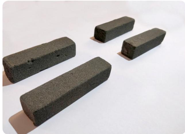
Fig. 06.1 a: 3D printed sand mould with furan binder system
