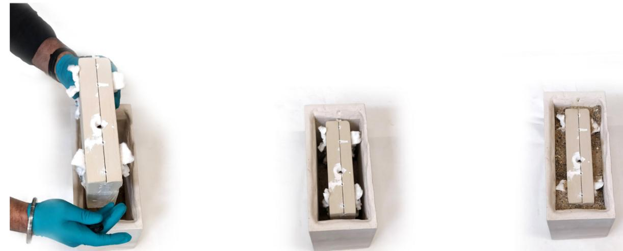
Fig. 07.2 j: placing sand mould inside the crystal cast mould and filling the remaining cavity with coarse sand.
