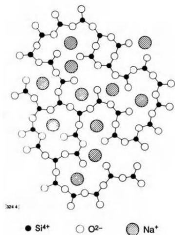
Fig 03.1 g: Molecular arrangement of Sodium Silicate Glass
