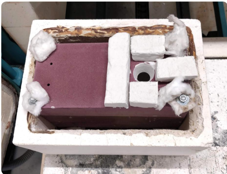
Fig. 07.2 q: Final setup of mould inside the furnace
