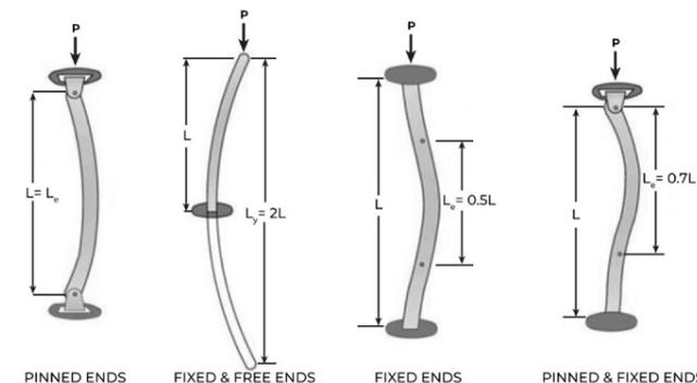
Fig. 03.3 c: Buckling of a column based on end supports (Charpedia n.d.)
