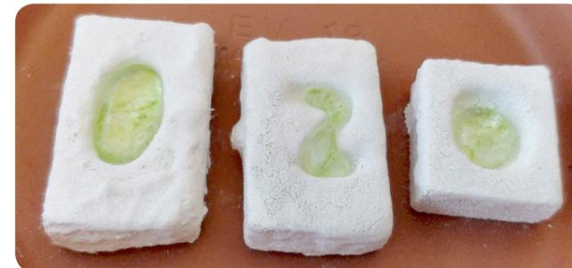
Fig. 06.7 e: Result of glass casted in dual layered coating of crystal cast and boron nitride
