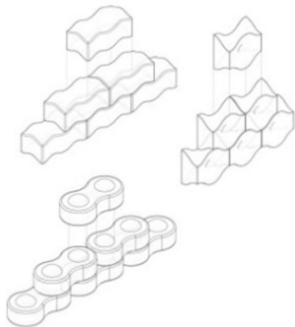
Fig. 03.8 c Interlocking geometries
