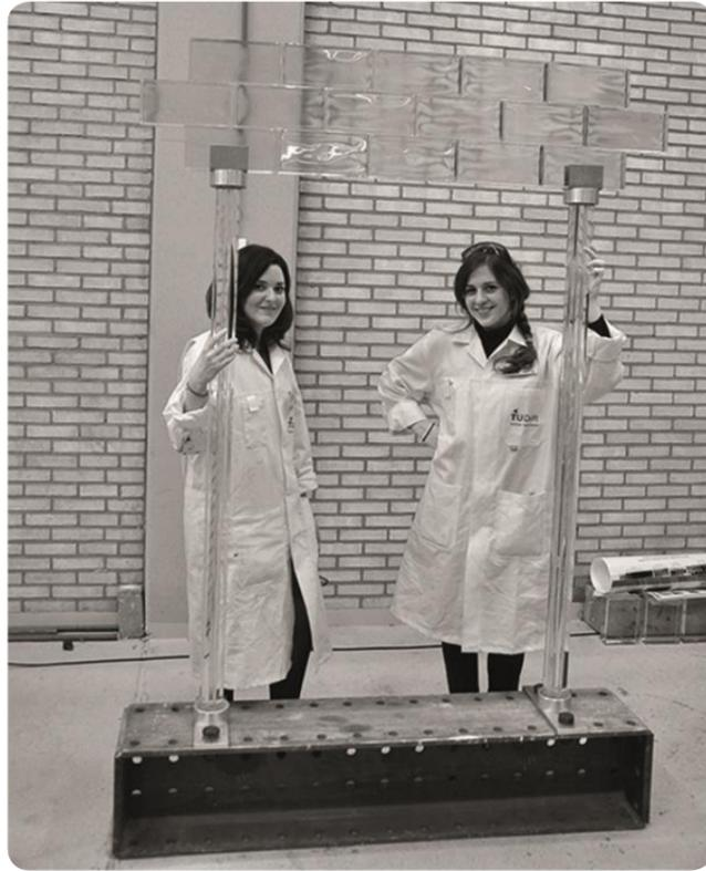
Fig. 03.3 o: 1.5 m high column prototype
