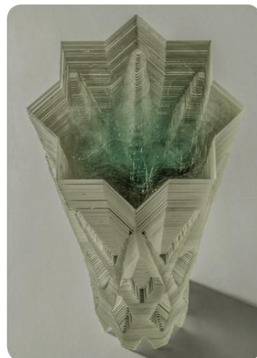
Fig. 03.3 j: Vertically Stacked glass column
