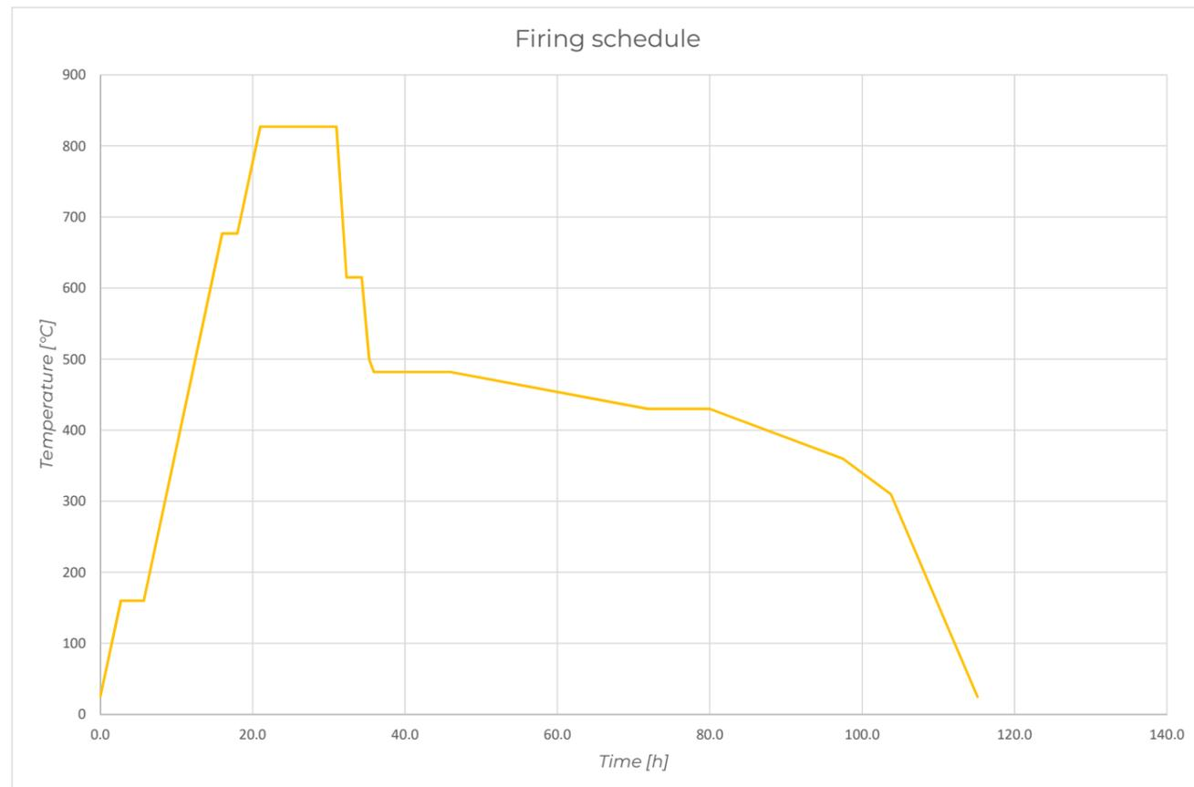
Fig. 07.2 m: Firing schedule of the kiln temperature v/s time
