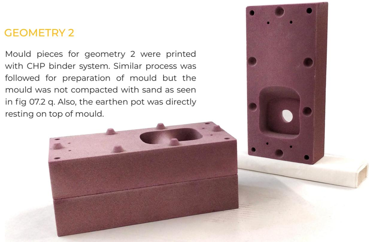
Fig. 07.2 n: 3D printed mould at 1:3 scale for prototyping
