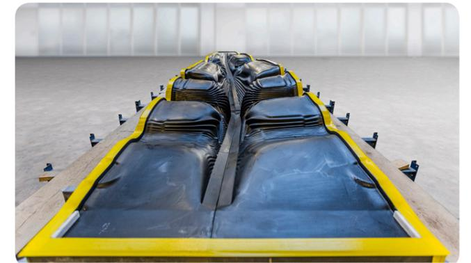
Fig. 03.6 k: Segments of 3D printed moulds stuck together to cast concrete slab and coated for finished surface and easy removal.(The Smart Slab n.d.)
