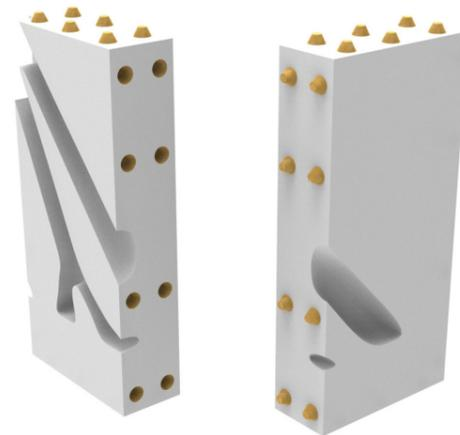
Fig. 08.1 e: Interlocking mechanism of the moulds
