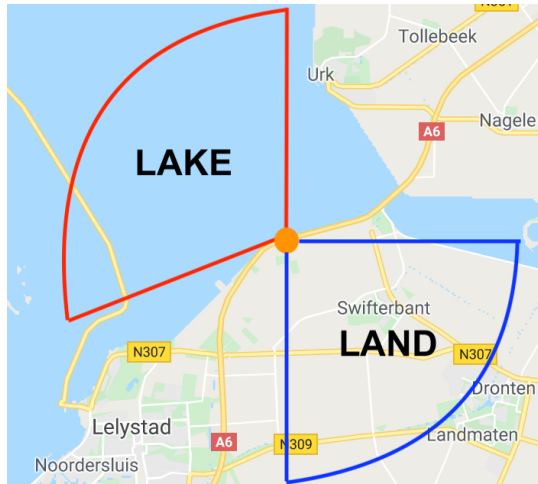
Figure 5.13: Lake and land wind direction sectors for LiDAR 1, indicated by the orange dot
