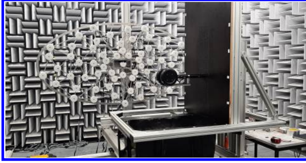
Fig. 2 Experimental setup conducted at TUD's A-Tunnel with the outlet nozzle Delft 40x70 [13] blowing in top wise direction. The landing gear shown features the installed fairing, whereas the microphone array is positioned sideline. On the right hand side the setup during image acquisition is shown.
