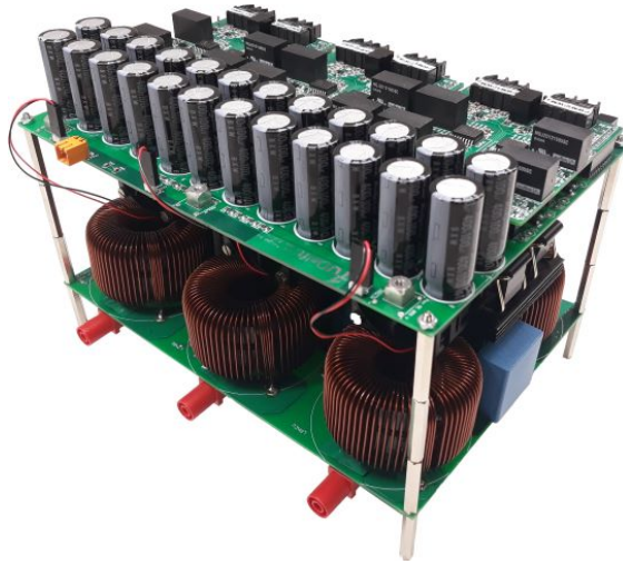
Figure B.4: Prototype of the 10kW 2L-VSC used for the efficiency testing of the mcHyS with LCL filter in the bottom.
