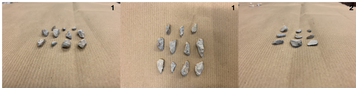
Figure 5.3: Flakiness and shape index particles [1/2]
