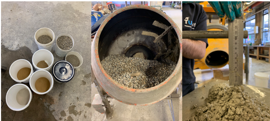
Figure E.3: Material selection (left), mixing (middle) and slump test (right)
