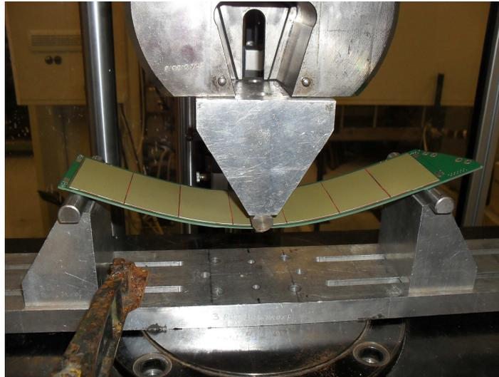
**Figure 3-1: Test set-up three point bending**
