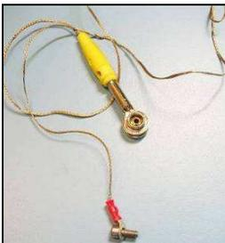
To ensure comparable test conditions at different locations and to avoid short-circuits the satellite needs to be electrically grounded. Delfi-C<sup>3</sup> made use of a clip for grounding. Delfi-n3Xt will make use of bolts for grounding as shown on Figure 11-12. A hole for grounding has been implemented in the BOP.
