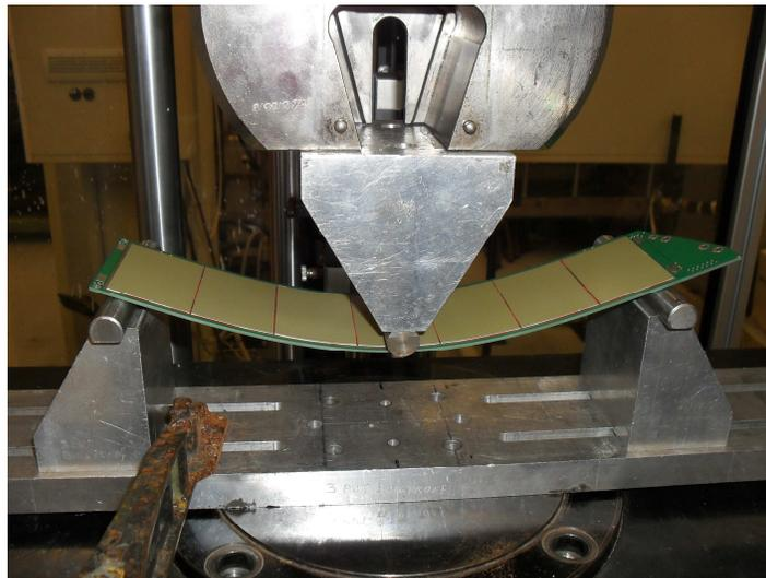
**Figure 3-2:** Bending test on solar panel PCB with dummy solar cells
