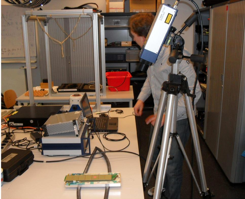
**Figure 6-7:** Frequency test set-up with dummy panel
