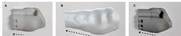
Figure G.13: Difference in tapered extrusion; (a) first design; (b) 3D-model of vaginal cavity; (c) tapered extrusion based on 3D-model of vaginal cavity.
