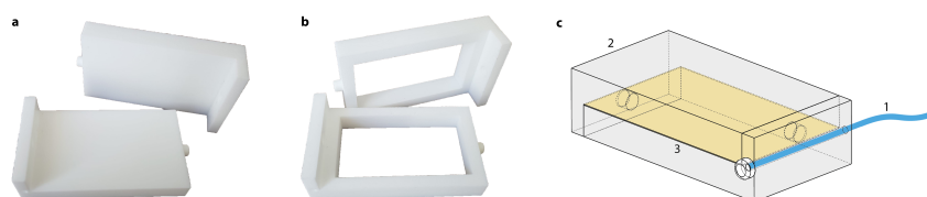
Figure 6.1: The two test boxes used during the experiment; (a) test box 1 with closed surface; (b) test box 2 with open surface; (c) schematic illustration of test box 1 with placed GaFchromic film segment and flexible implant tube inserted in the needle channel: 1. Flexible implant tube; 2. Test box 1; 3. GaFchromic film segment.
