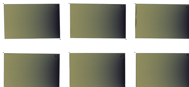
Figure 6.3: Scans of the six irradiated film segments. Upper row: film segments 1, 2 and 3 (irradiated in test box 1: closed surface); lower row: film segments 4, 5 and 6 (irradiated in test box 2: open surface).
