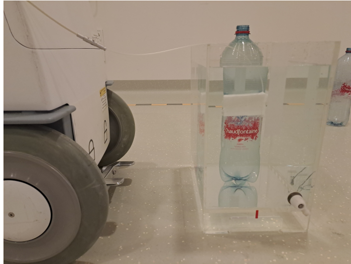
Figure H.4: Experimental set up. Side view of the Flexitron afterloader (left), water tank and plastic bottle with test box 1 taped to it. The flexible implant tube is inserted in the test box and connected to the afterloader.
