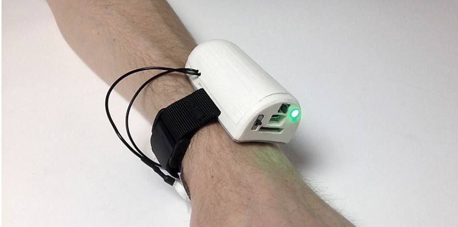
Figure 7. Second version of the open design EDA sensor unit.
