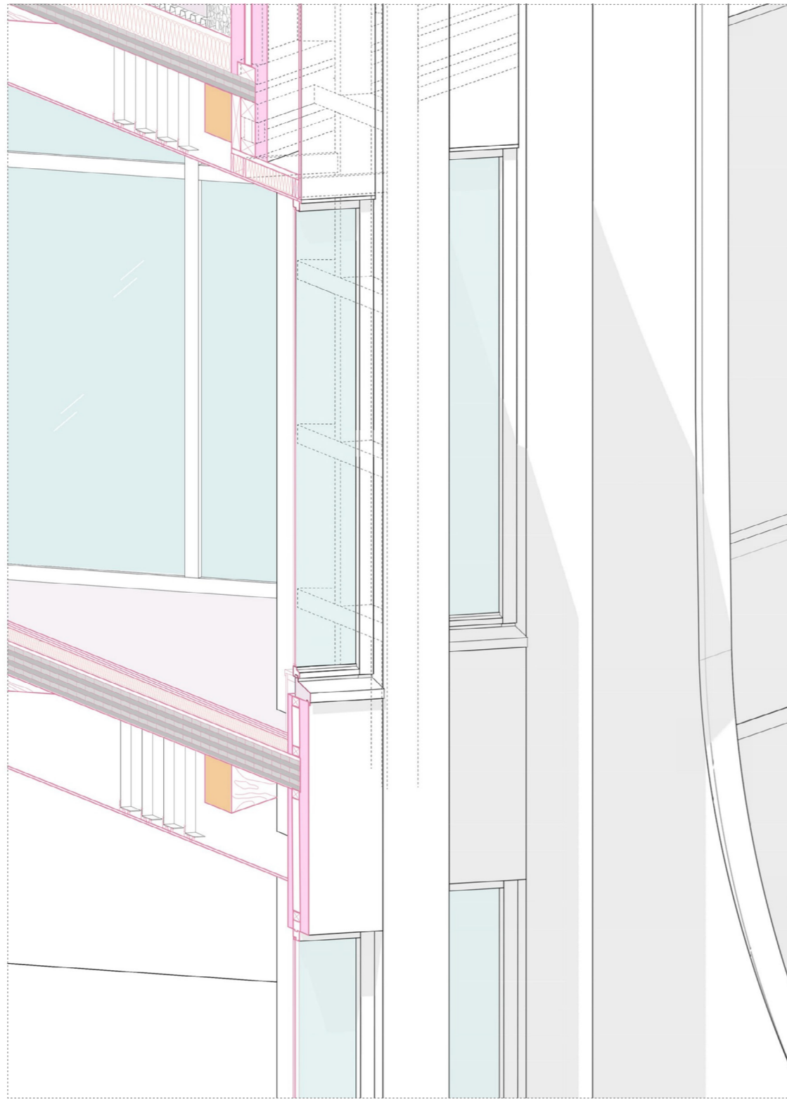
Figure 36: Axonometric detail of vertical louvre-like hempcrete forms as part of the Docking Station façade exploration.
