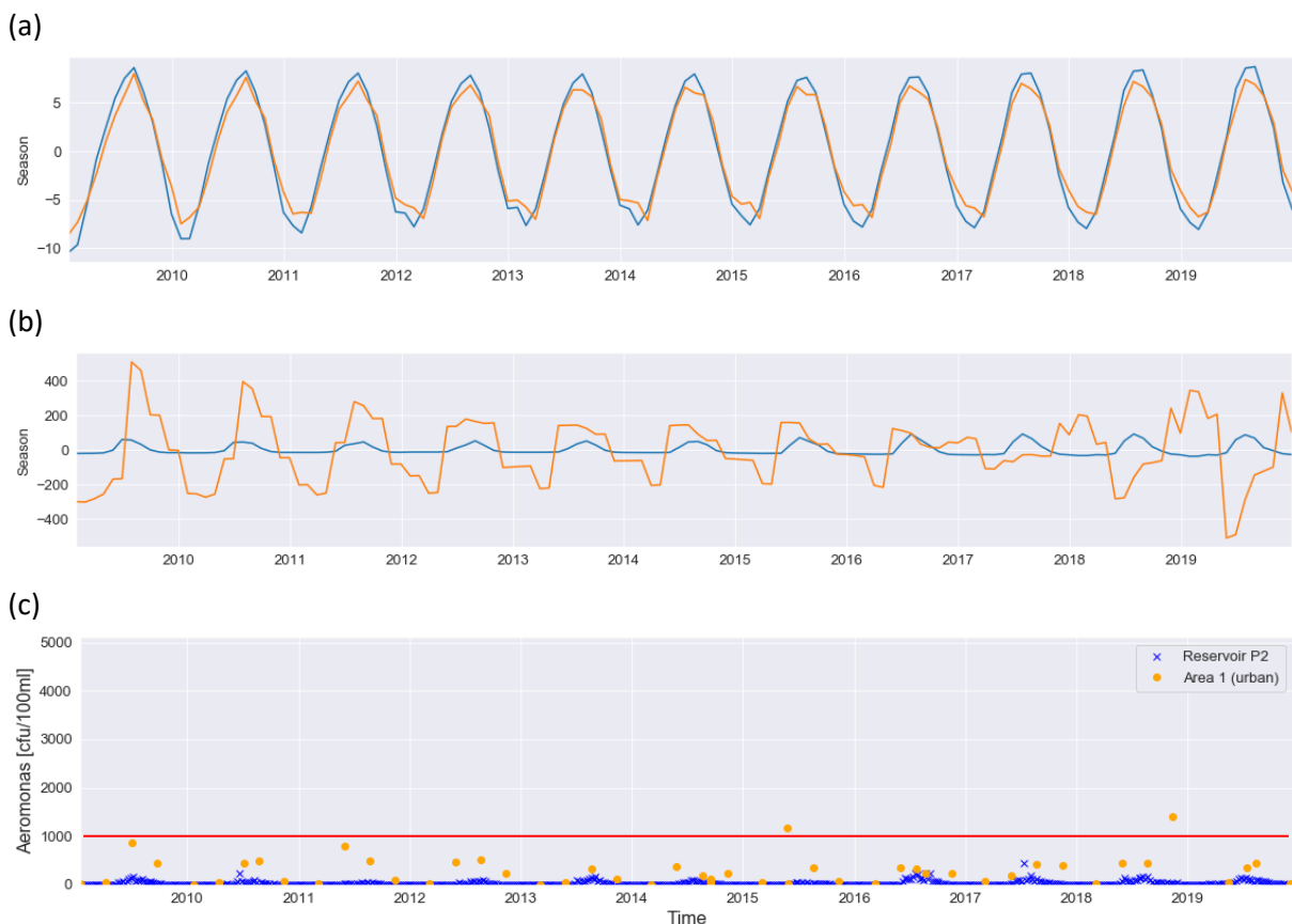
Figure 24 - Area 1 (urban) with Seasonal pattern of absolute sample temperature ( ^{\circ}\text{C} ) (a) and seasonal pattern of Aeromonas samples (cfu/100ml) (b). Aeromonas sample values (cfu/100ml) for Area 1 (orange), reservoir P2 (blue) and drinking water standard (red) (c).
