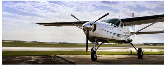
Figure 2.1: Example of a modern strut-braced wing aircraft (Cessna Caravan)
