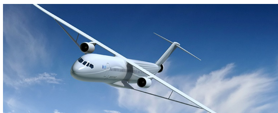
Figure 2.3: Example of strut-braced wing aircraft concept developed by Boeing (SUGAR research)
