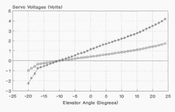
input voltage (up) -\* output voltage(up)
