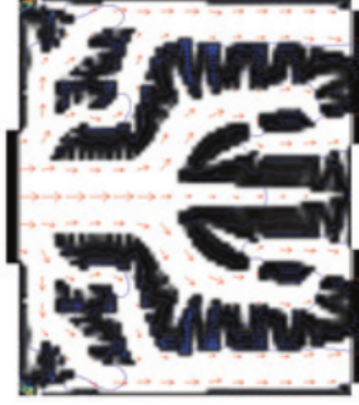
Figure 3.6: Optimised design showing root like structure[27]. The black regions are regions of highly conductive solid material, and the white regions of fluid material. The fluid enters the system from the left boundary and exits from the right one. Heat is generated throughout the domain.
