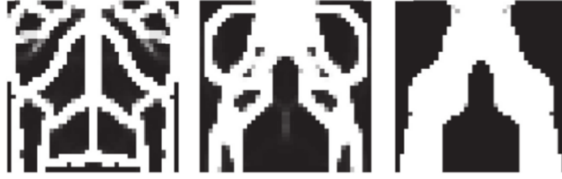
Figure 3.5: Optimised design for varied pressure drop[10]. The black regions are regions of highly conductive solid material, and the white regions of fluid material. The fluid enters the system from the top boundary and exits from the bottom one. Heat is generated throughout the domain.
