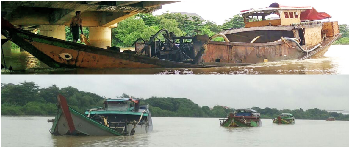
Figure D.1: During high tide several barges were observed carrying a mixture of fine sediment and water upstream. They raced against the rising water to make it past certain bridges. In the upper picture: a sailing barge just in time to pass under the bridge. Four more barges after this followed, approaching in the lower picture. Both pictures were taken shortly after each other, 17 km upstream of the mouth of the Pazundaung Creek
