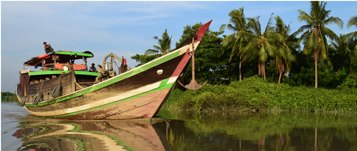
Figure D.4: An unloaded barge is making its way back downstream, note the difference in draught of about 1 m, compared to a loaded barge.
