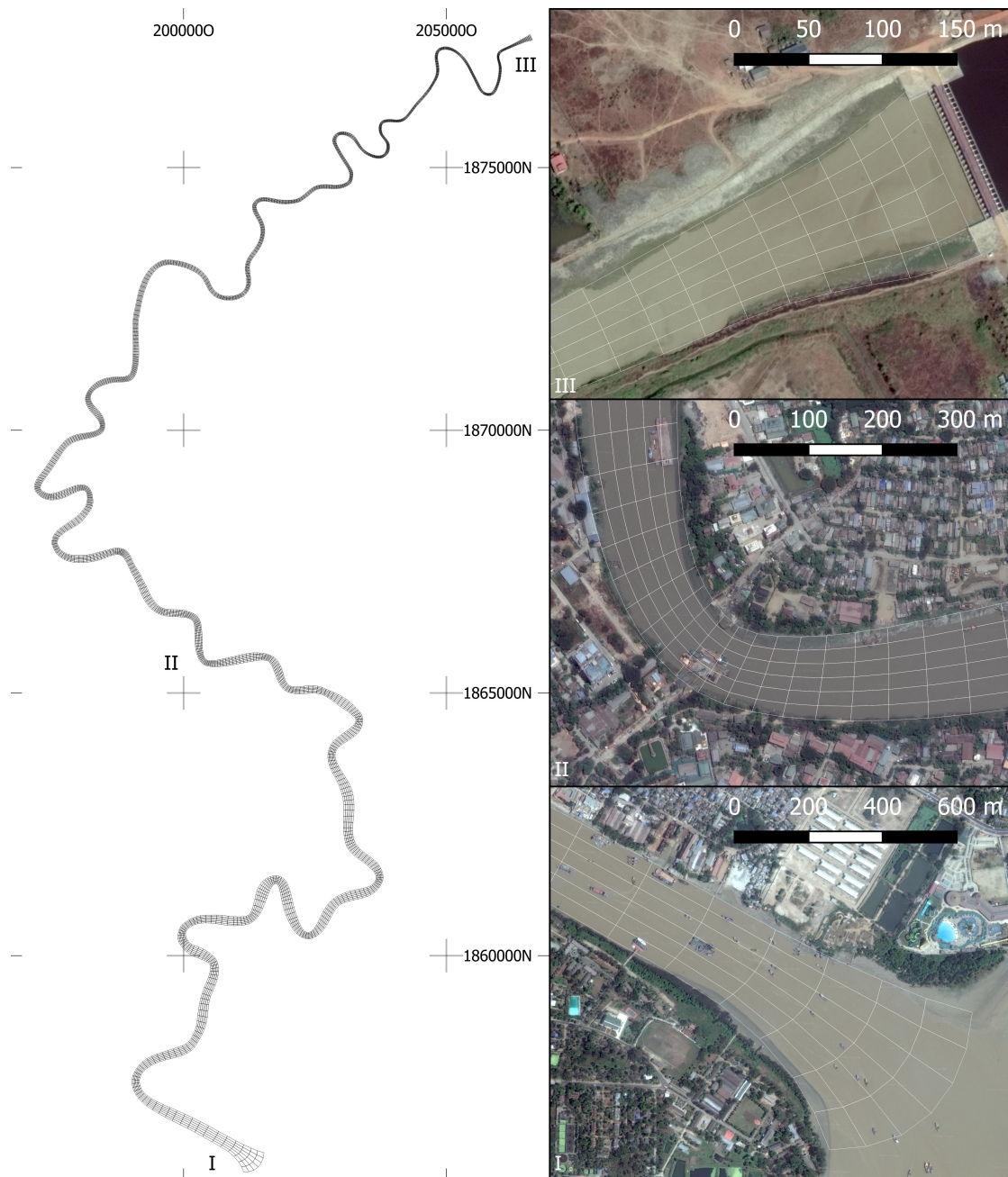
Figure 3.5: The computational grid is generated based on Google Earth satellite imagery and consists of 6 by 840 grid cells
