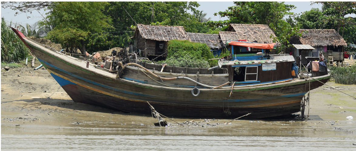
Figure D.5: A barge on the river bank, during low water. From this and the above pictures assumptions for the draught of a loaded (2 m) and unloaded barge (1 m) are made
