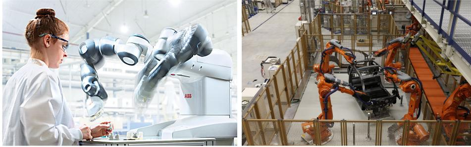
(a) Collaboration between a robot and its operator<sup>1</sup> (b) High performance robot manipulators working in an enclosed perimeter<sup>2</sup>
