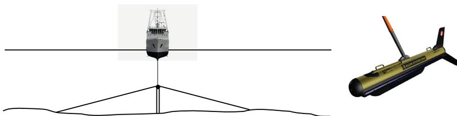
**Figure 2.1:** Schematic of a survey with a side-scan sonar (left) and illustration of a Klein 5900 side-scan sonar (right, <http://www.1-3klein.com/>).
