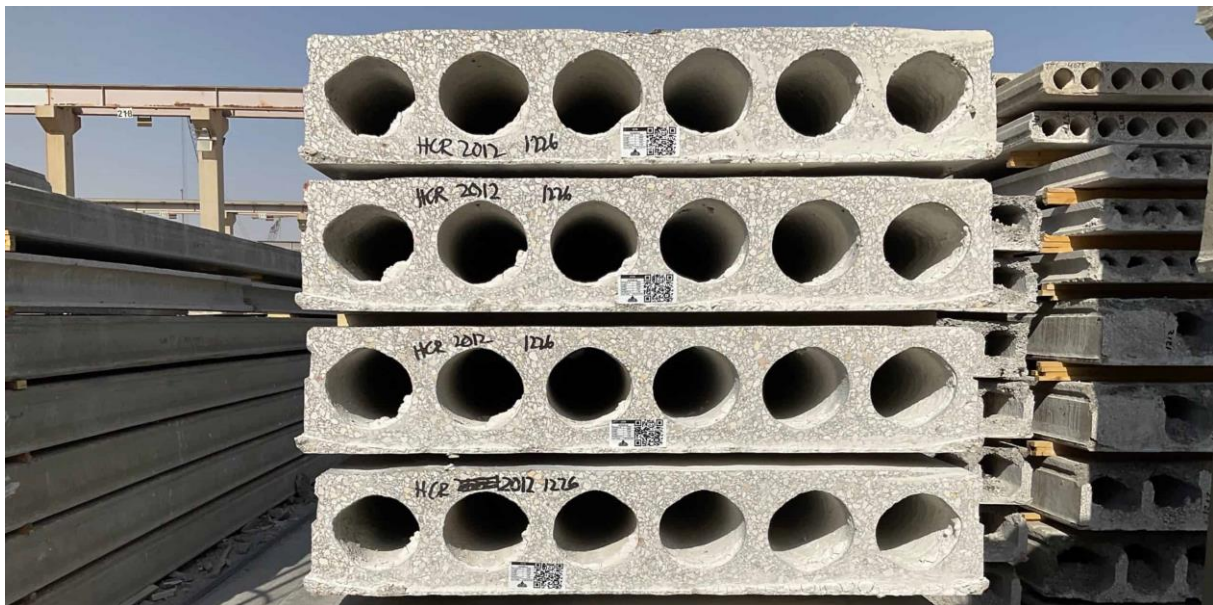
Figure 10 Prefab Slab Elements Prepared for Digital Traceability
