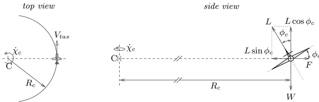
(a) geometry of a stationary horizontal turn ( $\beta=0$ )
