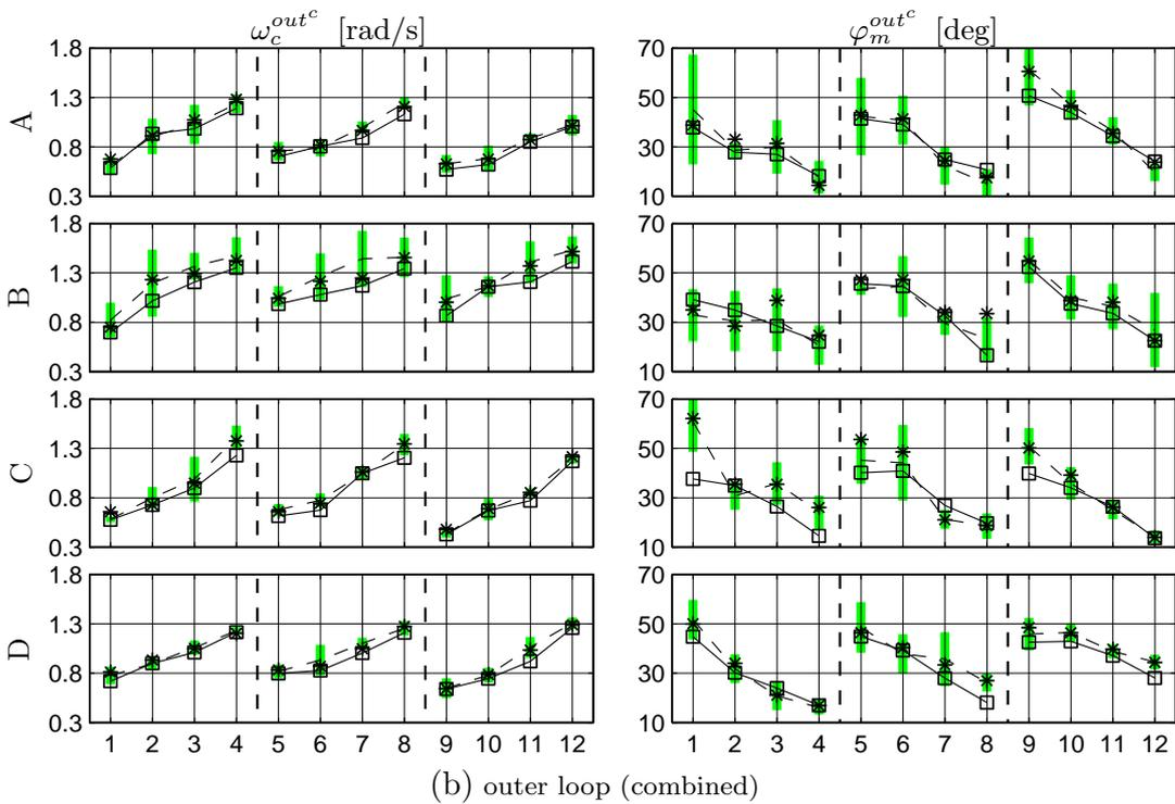
**Figure 5.9:** Crossover frequencies and phase margins (all subjects, all conditions). The shaded areas show the uncertainty regions of the *raw* frequency response data, their averages connected with the dashed line. The ‘\*’-symbols show the quantities for the *averaged* frequency responses, whereas the squares show them for to the MLMs.
