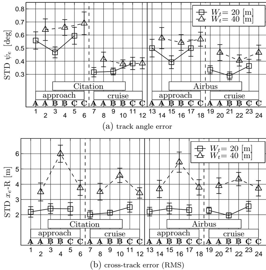
**Figure 10.18:** The means and 95% confidence limits of the STDs of the dependent measures (all subjects).
