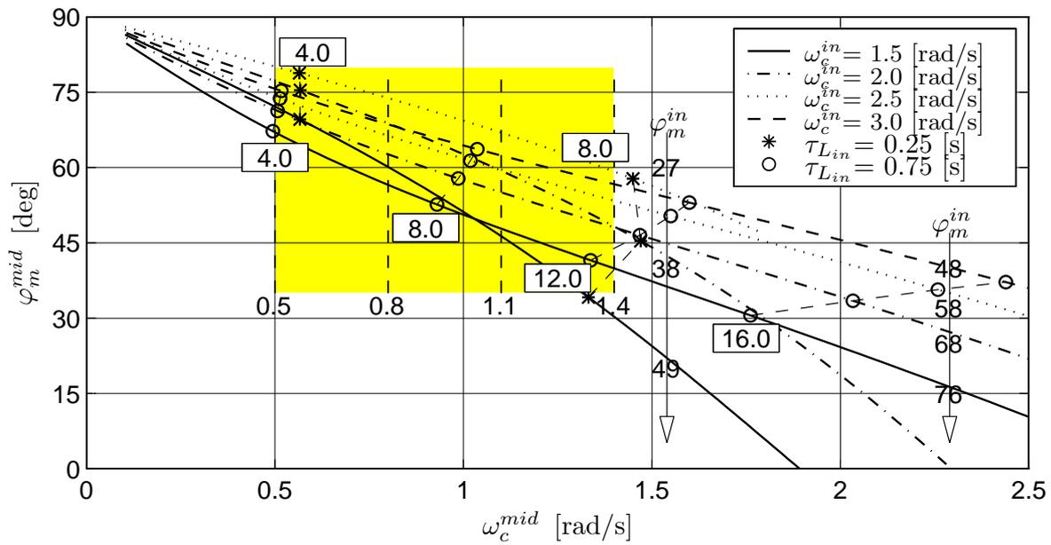
**Figure E.4:** The middle loop crossover frequency and phase margin as a function of the middle loop pilot gain  $K_{p_{mid}}$  for four levels of the inner loop crossover frequency  $\omega_c^{in}$  and two values of the inner loop pilot lead  $\tau_{L_{in}}$ . The values of  $K_{p_{mid}}$  are shown in the upper and lower insets for the lead times  $\tau_{L_{in}}=0.25$  [s] and  $\tau_{L_{in}}=0.75$  [s], respectively. The arrows show the inner loop phase margins for both the conditions.
