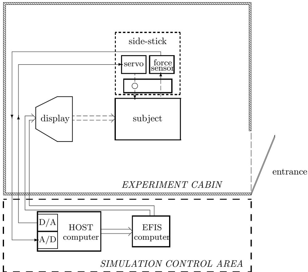
**Figure A.1:** Lay-out of the laboratory and a pictorial representation of the elementary information flow in the simulation environment.
