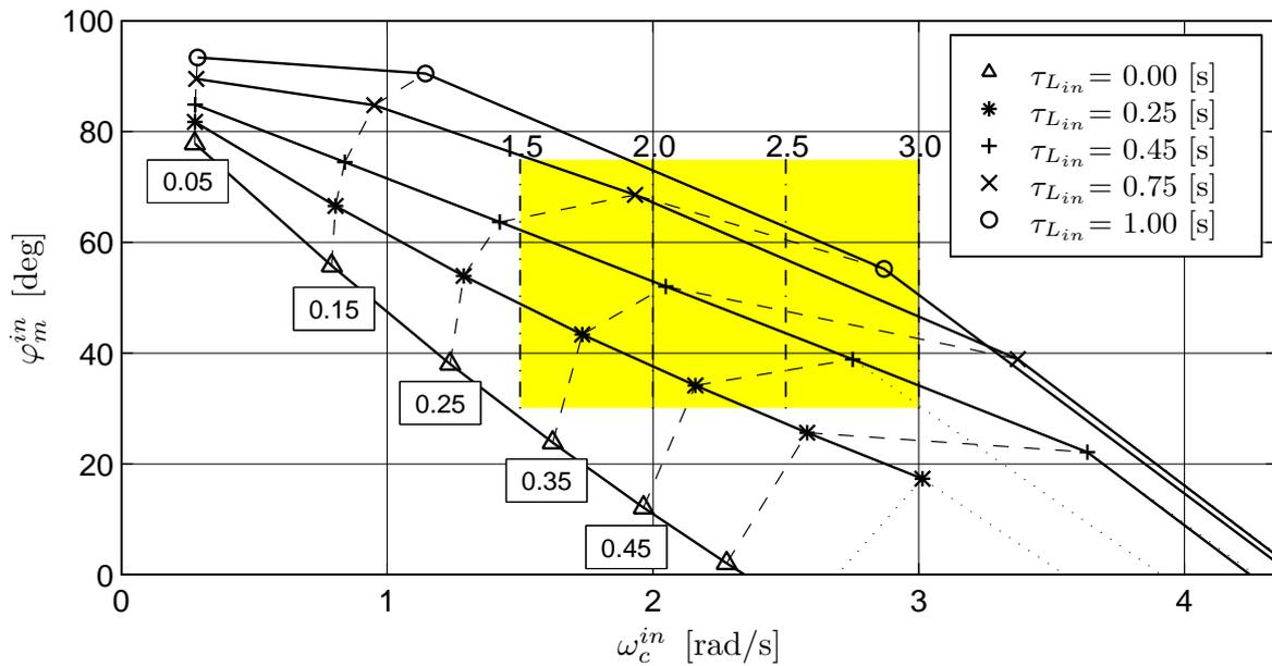
**Figure E.3:** The inner loop crossover frequency and phase margin as a function of the inner loop pilot gain  $K_{p_{in}}$  for five levels of the pilot lead  $\tau_{L_{in}}$ . The dashed lines represent iso- $K_{p_{in}}$  lines (with levels marked in the insets) Here, and in the following, the filled rectangle contains approx. 90% of the values found in the experiments.
