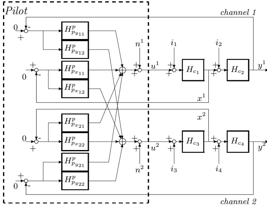
**Figure F.5:** The general situation of a *parallel* pilot model with four input signals and two output signals in a two-axis disturbance task. Two control channels can be distinguished that are controlled with two ( $2 \times 1$ ) parallel sub-models. The interference between both the channels is represented by the four cross-feeds.
