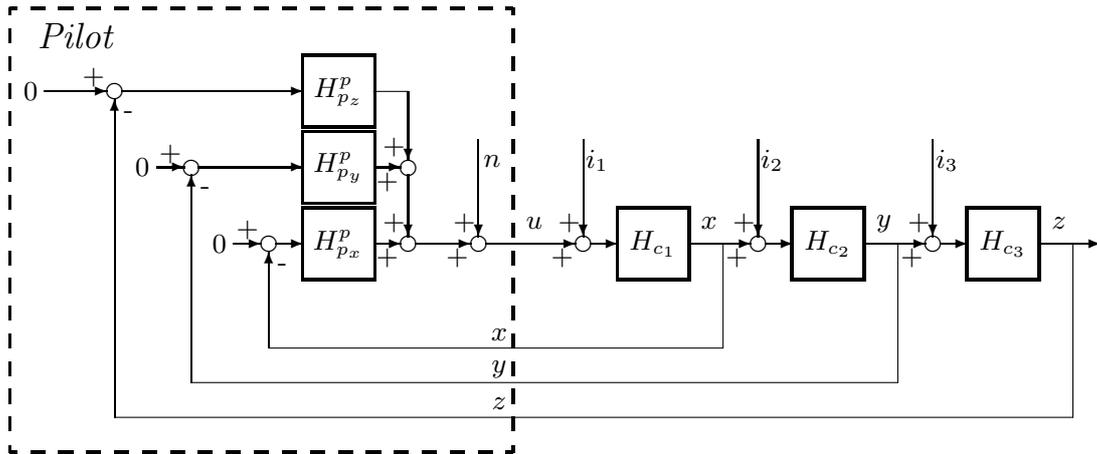
**Figure F.4:** The general situation of a *parallel* pilot model with three input signals and one output signal in a disturbance task.
