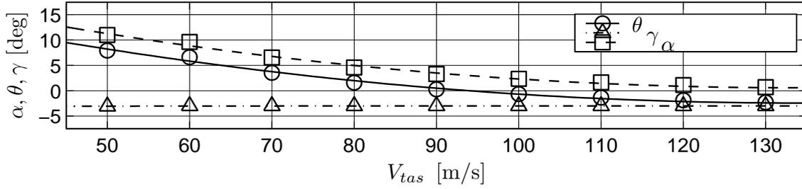
**Figure C.3:** The initial conditions of the aircraft angle of attack  $\alpha$ , angle of climb  $\gamma$  and pitch attitude  $\theta$  as a function of the velocity  $V_{tas}$  (Cessna Citation 500 – DASMAT).
