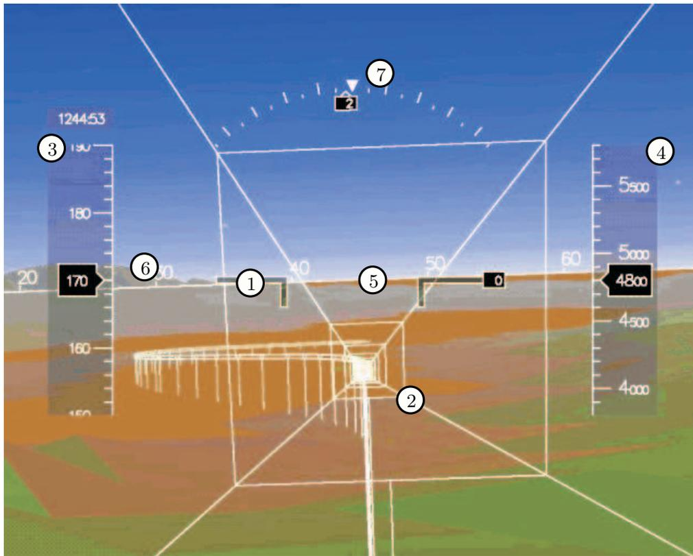
**Figure 1.6:** The Tunnel-in-the-Sky display. In this figure, ① depicts the aircraft symbol, ② the tunnel geometry, ③ the aircraft velocity (in [knots]), ④ the aircraft altitude (in [ft]), ⑤ the horizon line, ⑥ the heading angle indicators and ⑦ the bank angle indicator.
