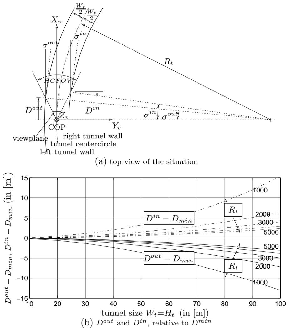
**Figure D.3:** The minimum viewing distances of the outer curve wall,  $D^{out}$ , and inner curve wall,  $D^{in}$ , shown with respect to the minimum viewing distance for a straight trajectory,  $D^{min}$ , as a function of the tunnel size  $W_t$  and the curve radius  $R_t$  (in [m]). The aircraft Body axes are aligned with the tunnel centercircle.
