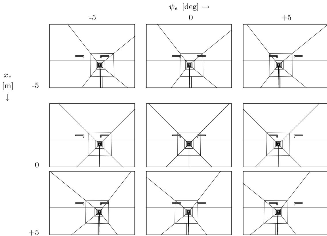
**Figure 2.11:** Distortion of the symmetry in the geometry of a generic tunnel-in-the-sky display.  $x_e$  and  $\psi_e$  represent the lateral position error and the heading angle error with respect to the trajectory, respectively.
