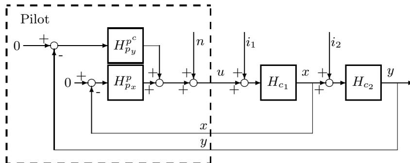
(a) estimation of the combined outer loop using the middle loop signal
