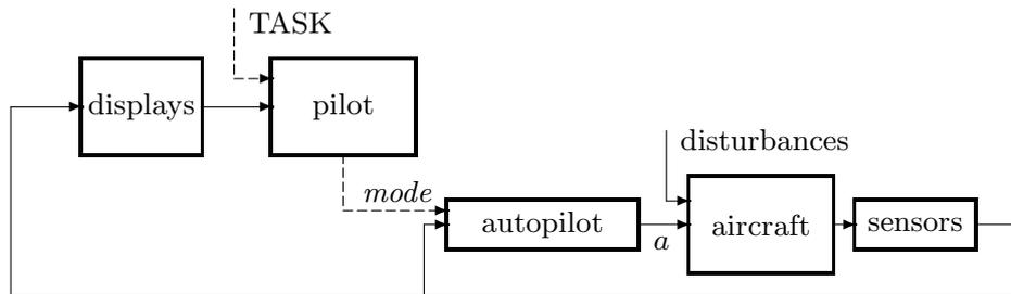
(b) supervisory control, *control augmentation*
