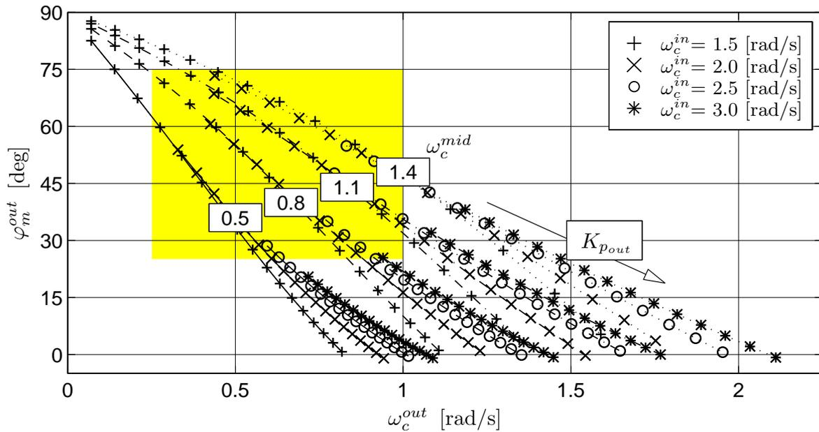
**Figure E.5:** The outer loop crossover frequency and phase margin as a function of the outer loop pilot gain  $K_{p_{out}}$  for four levels of the inner loop crossover frequency (legend) and four values of the middle loop crossover frequency (insets). The diagonal arrow shows the direction of increasing  $K_{p_{out}}$ .
