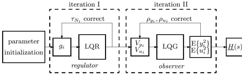
**Figure E.7:** Computation flow of the Optimal Control Model.
