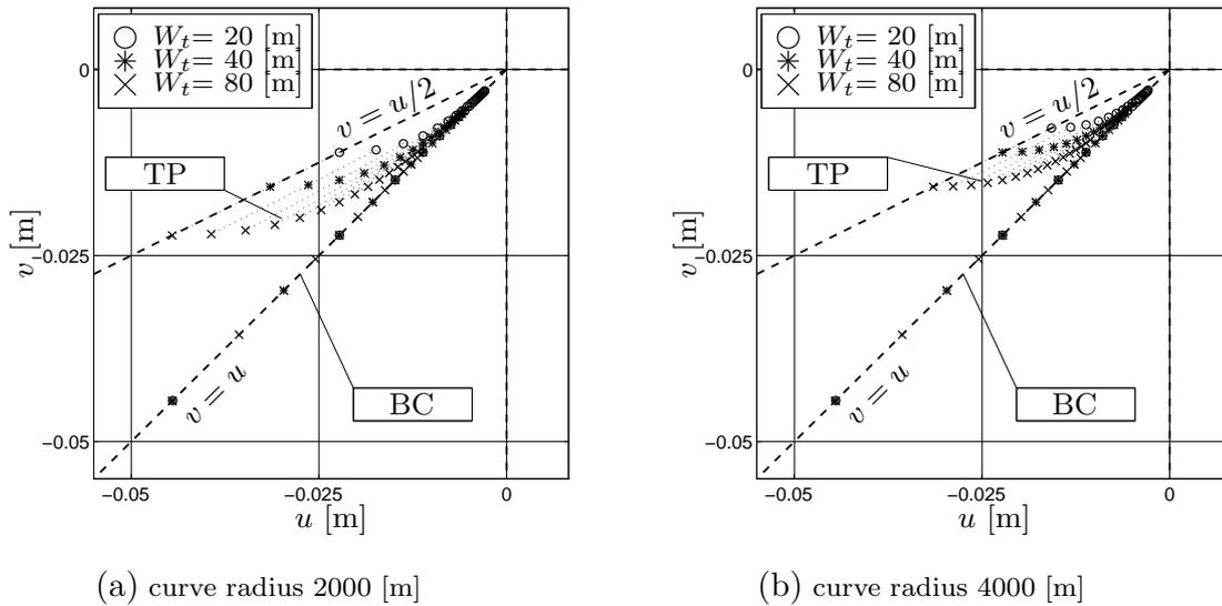
**Figure 10.10:** Successive projections of the tangent point (TP) and the point marking the beginning of the curve (BC). The curve is approached from an initial distance of 750 [m] to the start of the curve in steps of 75 [m]. Only the lower-left corner of the display is shown; the screen center is marked by the dashed lines ( $u = v = 0$ ).
