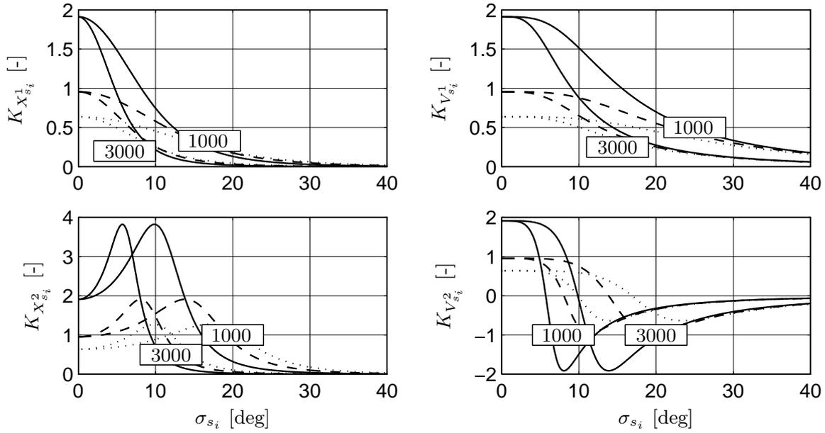
**Figure D.1:** Splay angle gains of the outer curve wall (top) and the inner curve wall (bottom) as a function of the viewing distance  $\sigma_{s_i}$ . It is assumed that the square tunnel ( $H_t=W_t$ ) is a perfect circle ( $\Delta\Psi=0$ ,  $\sigma_{s_i} = \sigma_{s_{i-1}}$ ). The lines represent the variables for two curve radii (1000 and 3000 [m]). The continuous, dashed and dotted lines represent tunnel sizes of 30, 60 and 90 [m], respectively.
