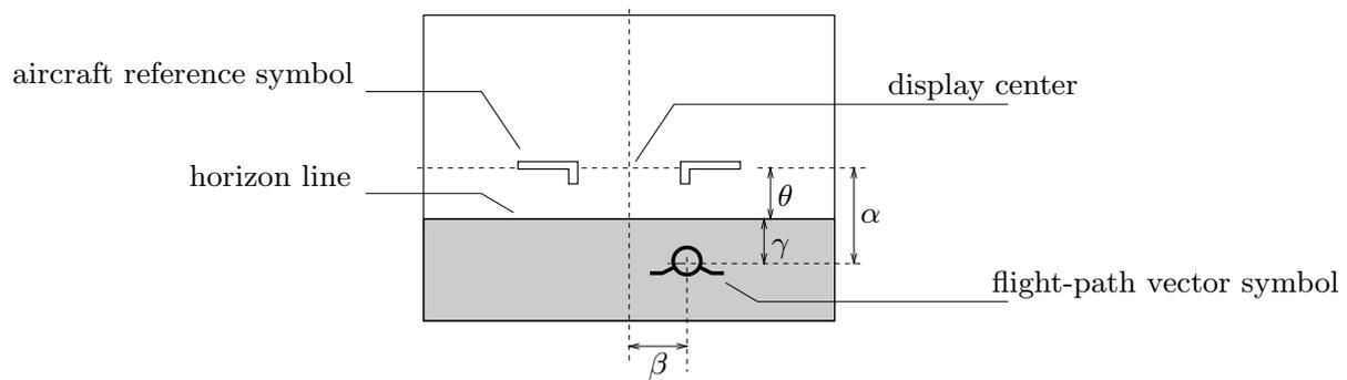
**Figure 9.1:** The flight-path vector: basics. The FPV shows the attitude  $(\alpha, \beta)$  of the aircraft velocity vector (the Aerodynamic reference frame  $\mathcal{F}^a$ ) with respect to the aircraft longitudinal axis (the Body reference frame  $\mathcal{F}^b$ ) depicted by the display center.
