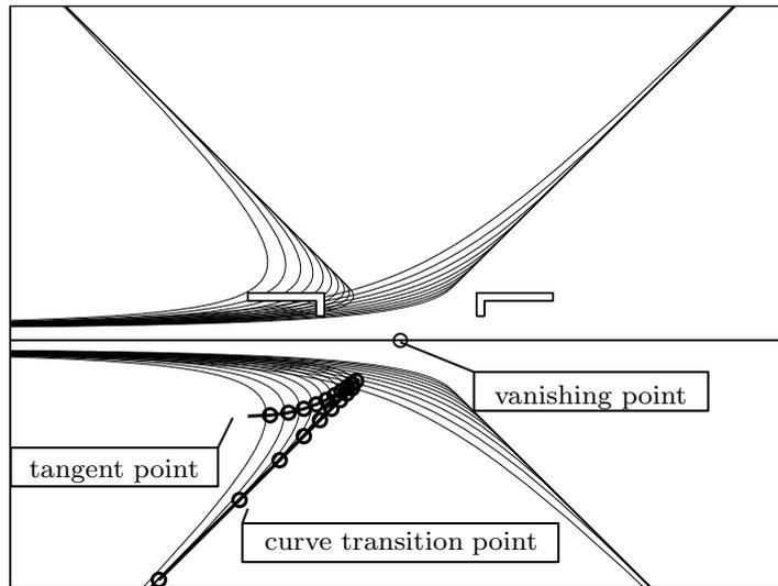
**Figure 10.8:** The frozen images of a 3-D *movie* showing the appearance of basic elements of the tunnel display when approaching a curve: tunnel-contour only. The movement of the tangent point (TP) is a cue for the approaching of the curve transition point (BC), which is less visible.
