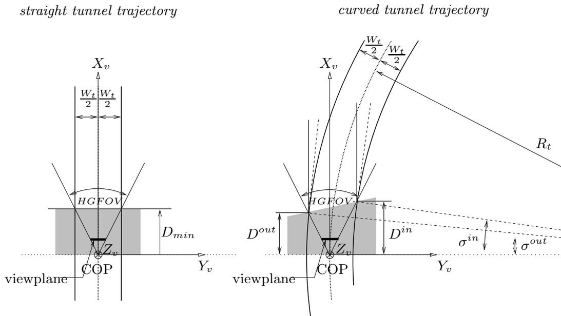
**Figure 8.3:** The effects of *not* showing the nearest part of the trajectory – due to the perspective projection method – for a straight (left) and curved (right) trajectory. The shaded areas indicate the part of the trajectory that is not visible for a pilot. The aircraft Body axes are positioned on and aligned with the tunnel centerline or centercircle.
