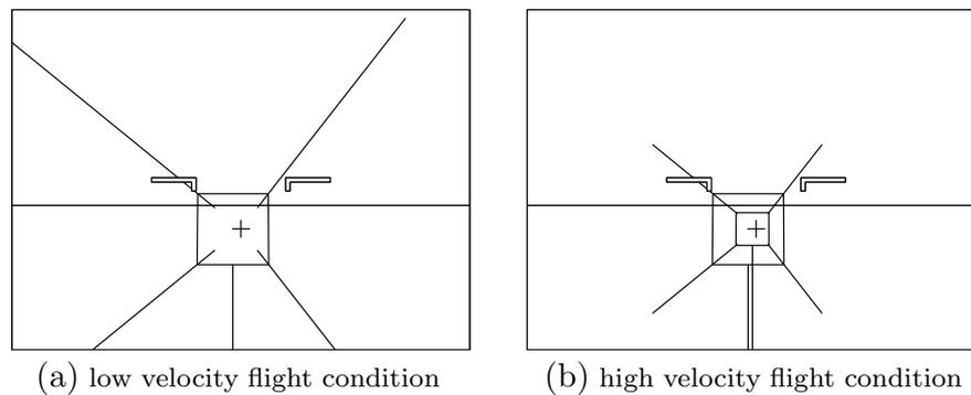
**Figure 6.13:** Tunnel images with a limited viewing volume for two velocity conditions. In these figures the cross symbol explicitly shows the *infinity point*, allowing pilots to directly perceive their heading with respect to the trajectory.
