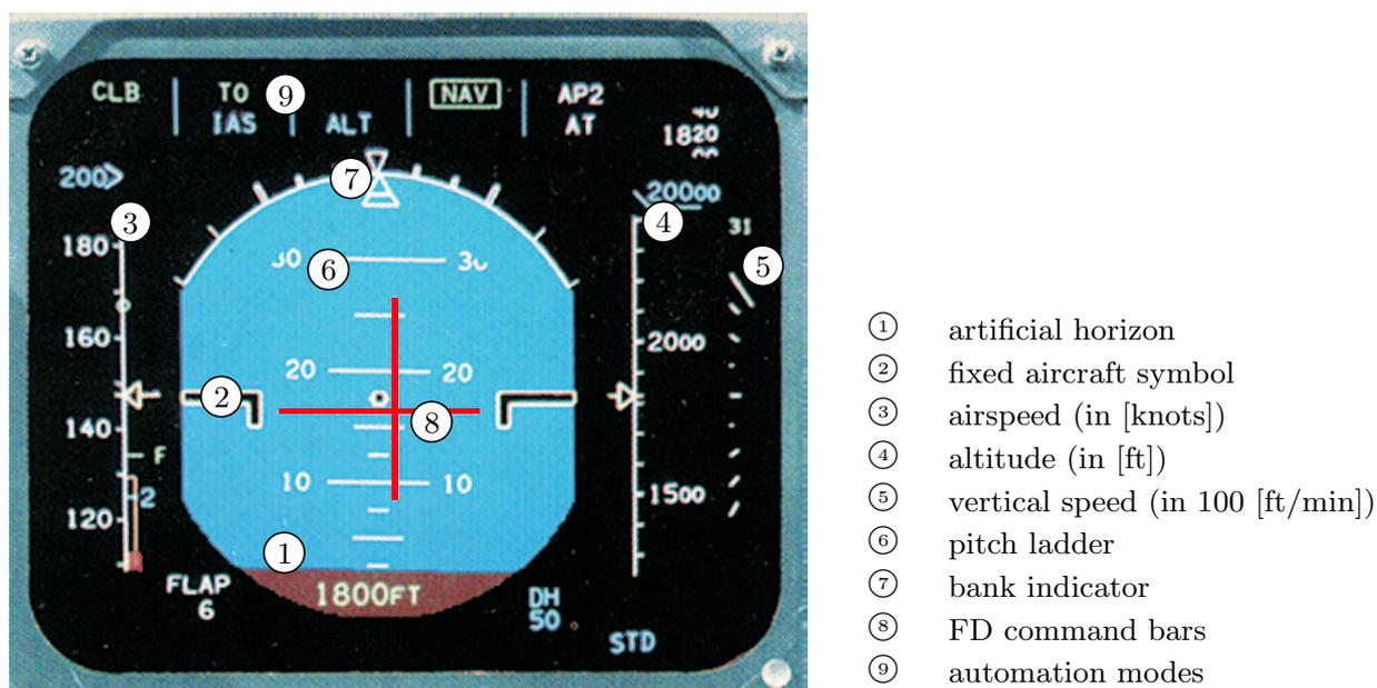
**Figure 1.4:** The Primary Flight Display (Fokker 100 version).
