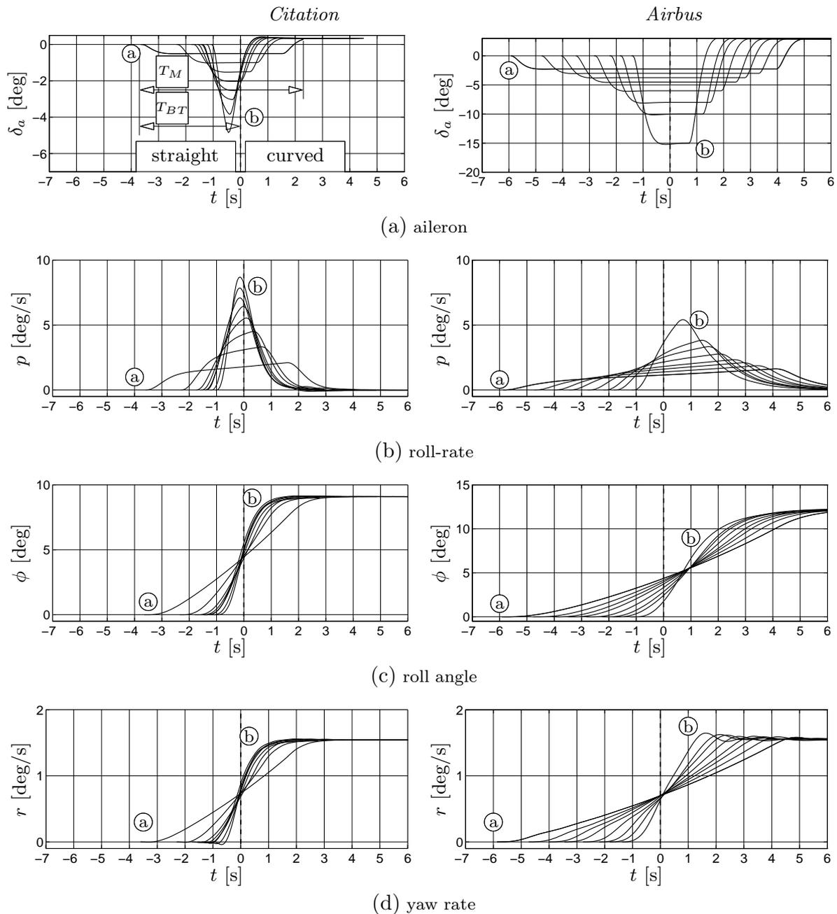
**Figure 10.4:** Time histories of the Cessna Citation 500 (left column) and the Airbus A300 (right column), plotted as a function of time relative to the start of the curve ( $t=0$ ) (van Oorschot, 1997b). In this figure, the ‘a’ and ‘b’ circles mark the *slow* and *fast* responses, respectively. Note that the steady-state value of  $\delta_a$  is non-zero and opposite to the initial deflection, a well-known idiosyncrasy of aircraft curve control.
