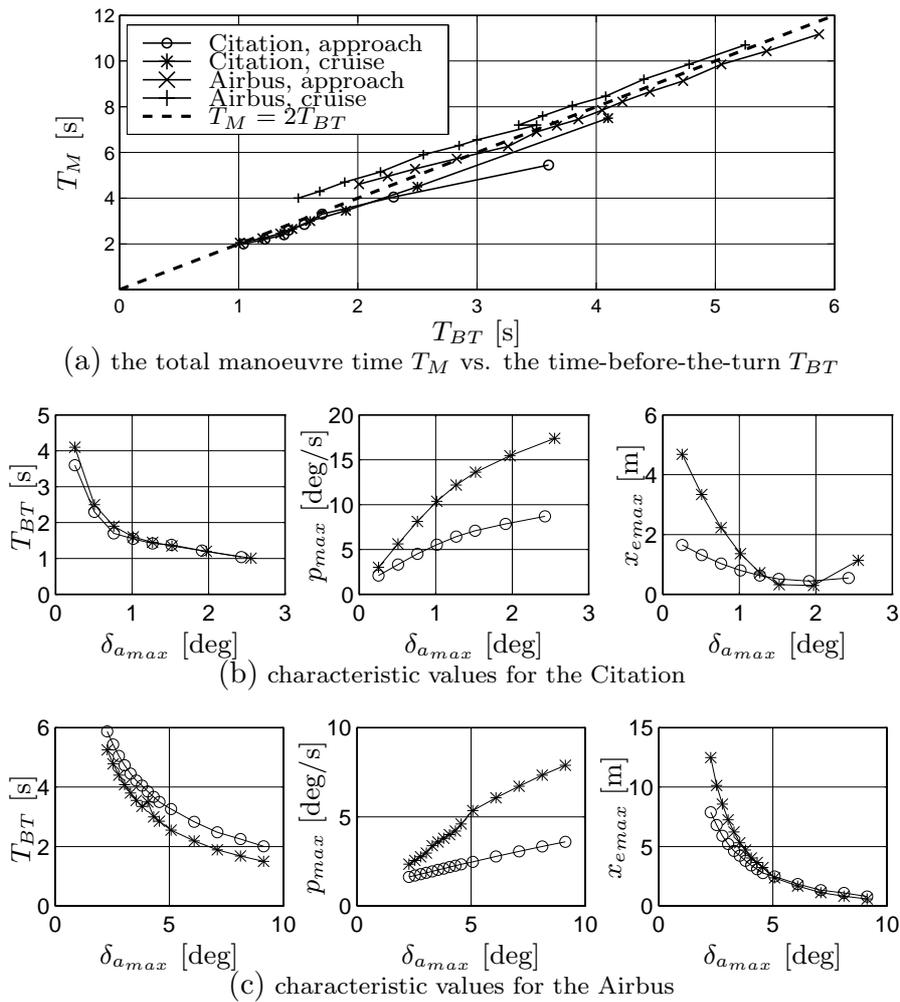
**Figure 10.5:** Characteristic values of the simulation study. The two bottom rows show the time-before-the-turn  $T_{BT}$ , the maximum roll-rate  $p_{max}$  and the maximum position error  $x_{e,max}$  as a function of the maximum aileron deflection  $\delta_{a,max}$ . The circles and asterixes represent the approach and cruise velocity conditions, respectively.
