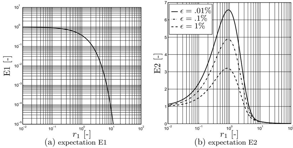
**Figure F.2:** The expectation quantities E1 and E2 as a function of the signal-to-noise ratio  $r_1$ . E2 is shown for three values of the probability variable  $\epsilon$  (Eq. F.14).
