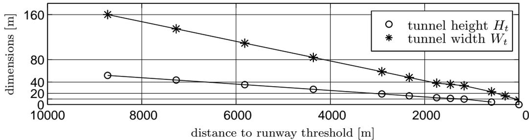
(b) inner tunnel dimensions for the RNP example in (a)
