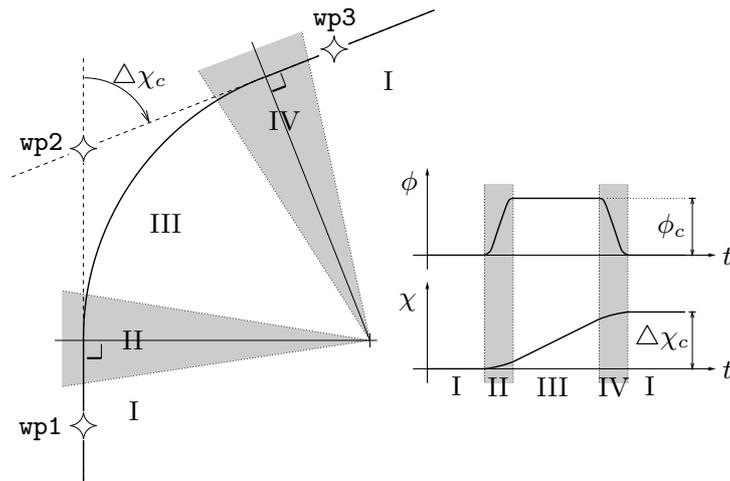
**Figure 2.8:** Analysis of the pilot's guidance task of following a FMS trajectory that is a concatenation of straight and circular segments (left). The right hand figure shows time histories of the aircraft roll angle  $\phi$  and the track angle  $\chi$ .
