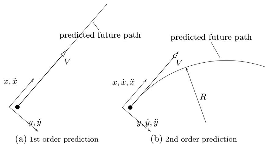
**Figure 9.2:** Two algorithms for predicting the aircraft future position. In this simplified figure,  $V$  represents the vehicle velocity and  $R$  the radius of the predicted circular future vehicle path. A first order algorithm (left) uses the aircraft position  $(x, y)$  and velocity  $(\dot{x}, \dot{y})$  in the inertial reference frame. A second order algorithm (right) extends the first order prediction by incorporating the vehicle accelerations  $(\ddot{x}, \ddot{y})$ .
