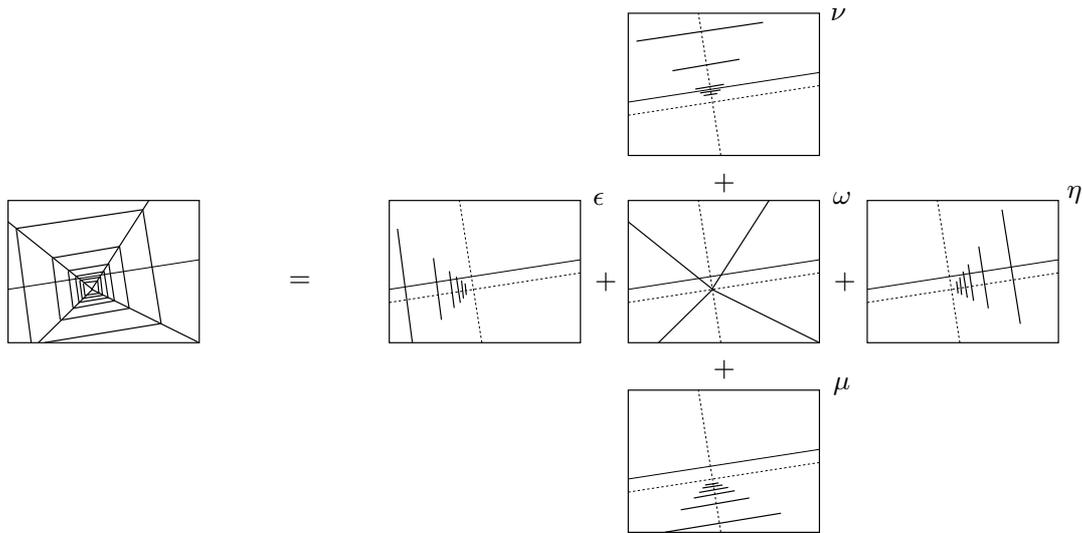
**Figure 7.1:** A generic tunnel (left) dissected in a number of entities (right), showing either optical splay –  $\omega$  – or optical density –  $\eta$ ,  $\epsilon$ ,  $\mu$ ,  $\nu$  – information. The dashed lines represent the horizontal and vertical pseudo-horizons through the infinity point.
