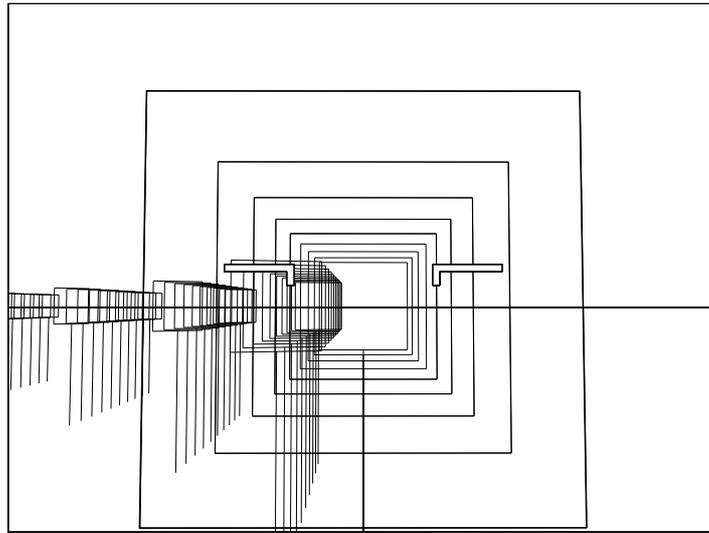
**Figure 10.7:** The frozen images of a 3-D *movie* showing the appearance of basic elements of the tunnel display when approaching a curve: tunnel-frames (and altitude poles) only.
