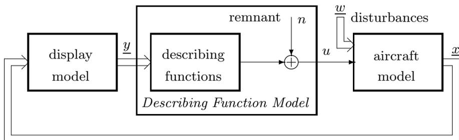
(c) the single-axis, multi-loop aircraft regulation task
