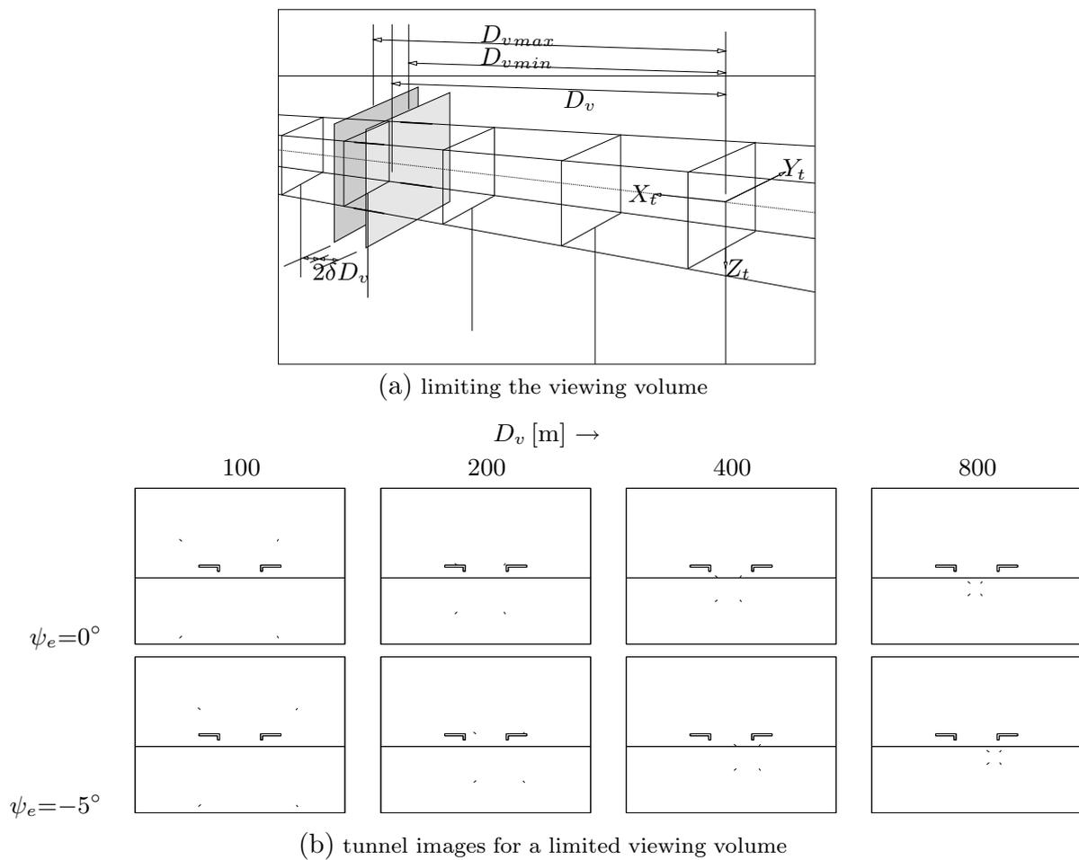
**Figure 6.1:** Limiting the viewing volume of the tunnel display to a small area around a viewing distance  $D_v$  (top). Defining the minimum and maximum viewplanes at a distance  $\delta D_v$  from  $D_v$  yields the projection on the viewplane of only the four line segments, resulting in the display images of the two bottom rows. The figures depict a situation for four viewing distances  $D_v$  ( $x_e=+5$  [m];  $\psi_e=0, -5$  [deg];  $W_t=H_t=40$  [m]).
