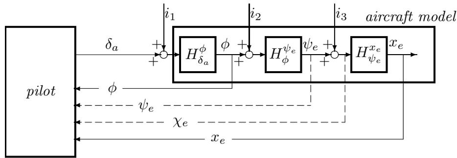
**Figure 9.5:** The composition of the three components of the aircraft dynamic model and the three disturbances inserted in the closed loop. This figure illustrates the fact that, dependent of the presence of the FPV symbol on the display, a pilot can close the middle loop using either  $\psi_e$  or  $\chi_e$ , where  $\chi_e = \psi_e + i_3$  and  $i_3 = \beta_g$ .
