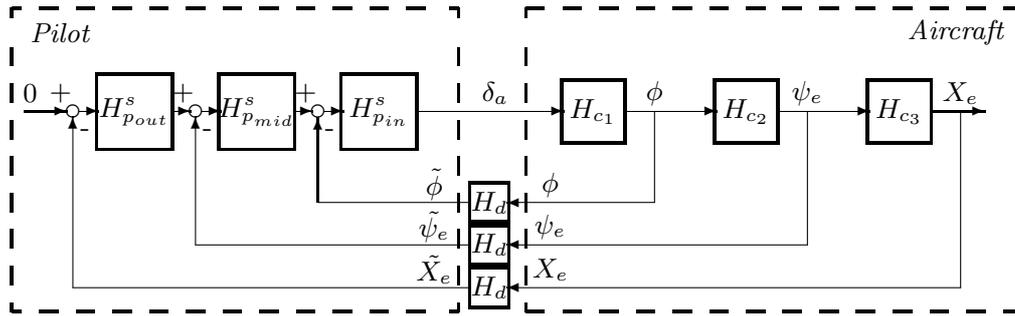
**Figure E.2:** Definition of the closed loop pilot/aircraft system of the sensitivity study. In this figure,  $H_{c1}$ ,  $H_{c2}$  and  $H_{c3}$  depict the aircraft inner, middle and outer loop dynamics.  $H_d$  indicates the simulation time delay that was present in the experiments of this thesis, see Appendix A.  $H_{p_{in}}^s$ ,  $H_{p_{mid}}^s$  and  $H_{p_{out}}^s$  are the pilot inner, middle and outer loop feedback characteristics, according to a *serial* model structure.
