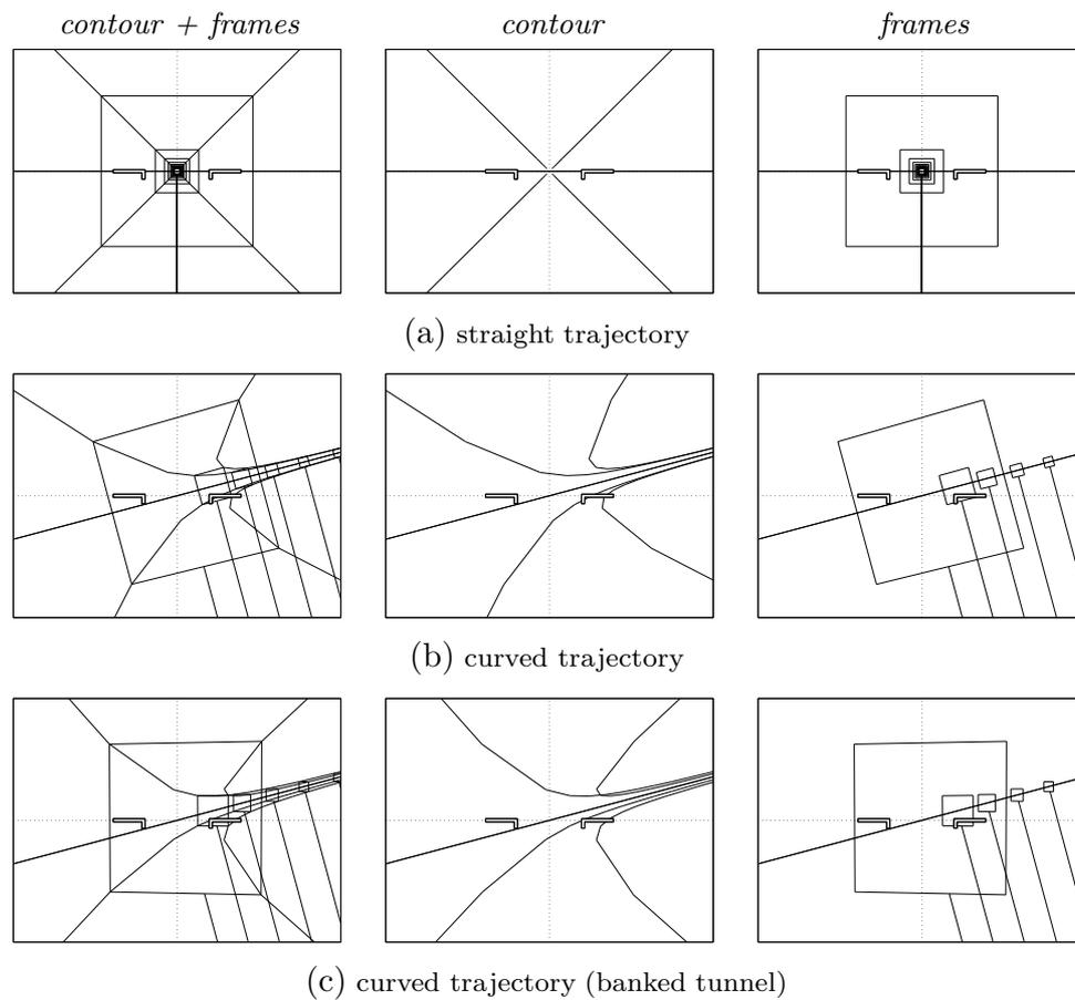
**Figure 8.2:** The tunnel display images corresponding to an aircraft recti-linear motion condition along a straight trajectory (top) and an aircraft curvi-linear motion condition along a circular trajectory (middle and bottom rows). The tunnel images are shown for the total display (left), the contour-only display (middle) and the frames-only display (right). The dotted lines represent the screen center. The aircraft attitude and position errors with respect to the trajectory are zero.
