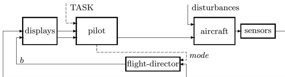
(c) manual control, *display augmentation***Figure 1.3:** Different types of flight guidance automation.
