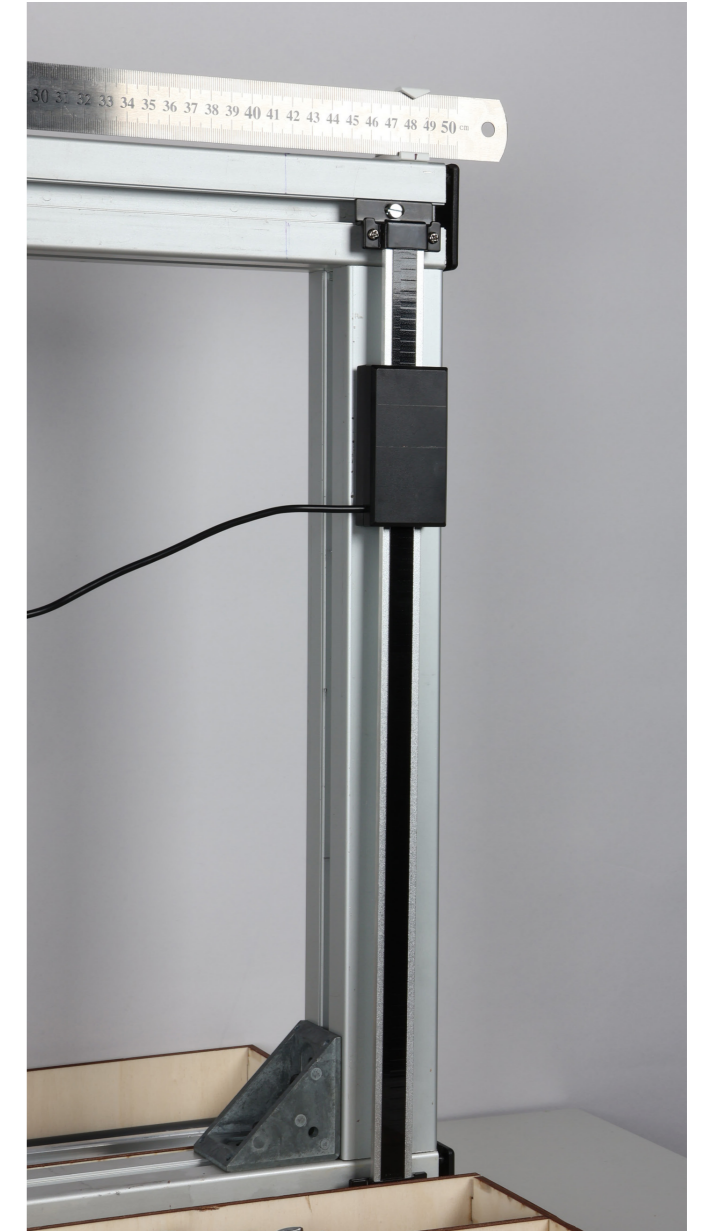
Figure 38: Digital ruler installed
