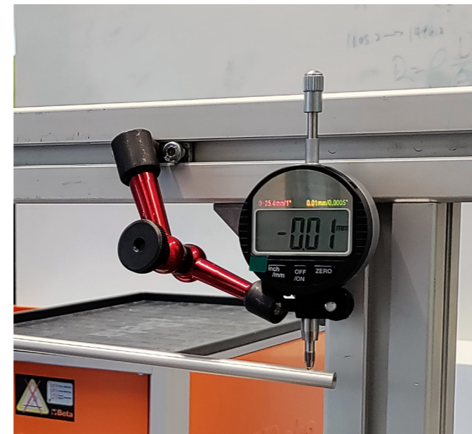
Figure 36: Digital dial gauge for deflection measurement
