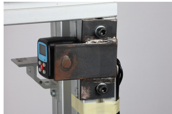
Figure 35: Custom steel holder
