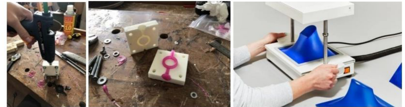
An example of a possible experiential machine to learn about injection molding [Gibbon, 2022] & FormBox: Vacuum Former
