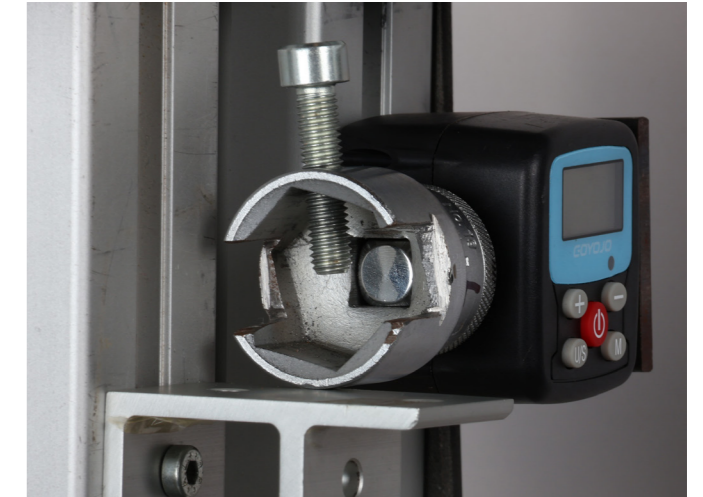
Figure 46: Large grip installed
