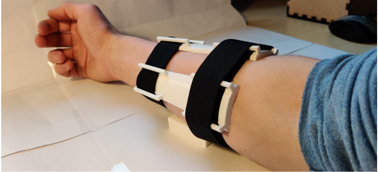
Figure L3. Forearm fixation concept 1 fastened around forearm (left).
