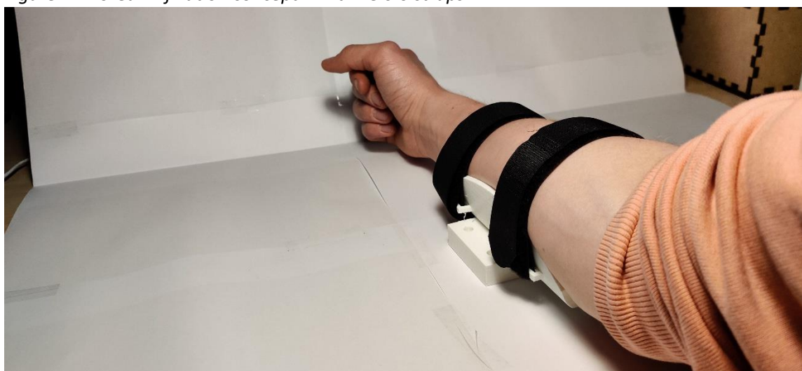
Figure L8. Forearm fixation concept 2 fastened around forearm (left).
