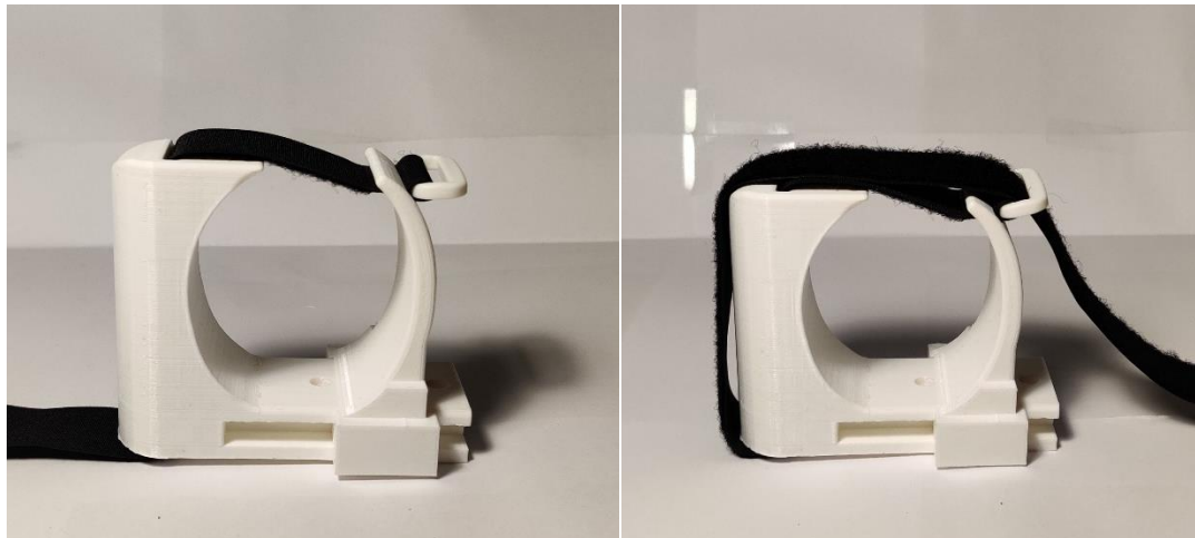
Figure H31. Concept 3 (V1 - elbow) prototype assembled with strap.
