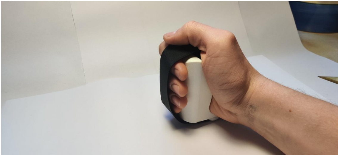
Figure P9. Hand fixation concept 2 with hand fastened and fingers underneath strap.
