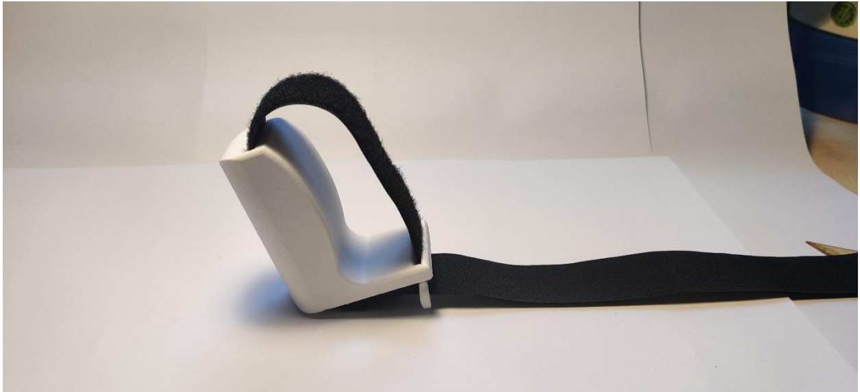
Figure P5. Hand fixation concept 2 with strap.
