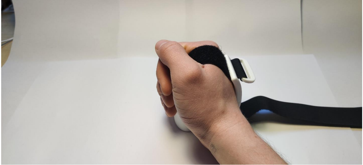
Figure P3. Hand fixation concept 1 with hand fastened and fingers around strap.
