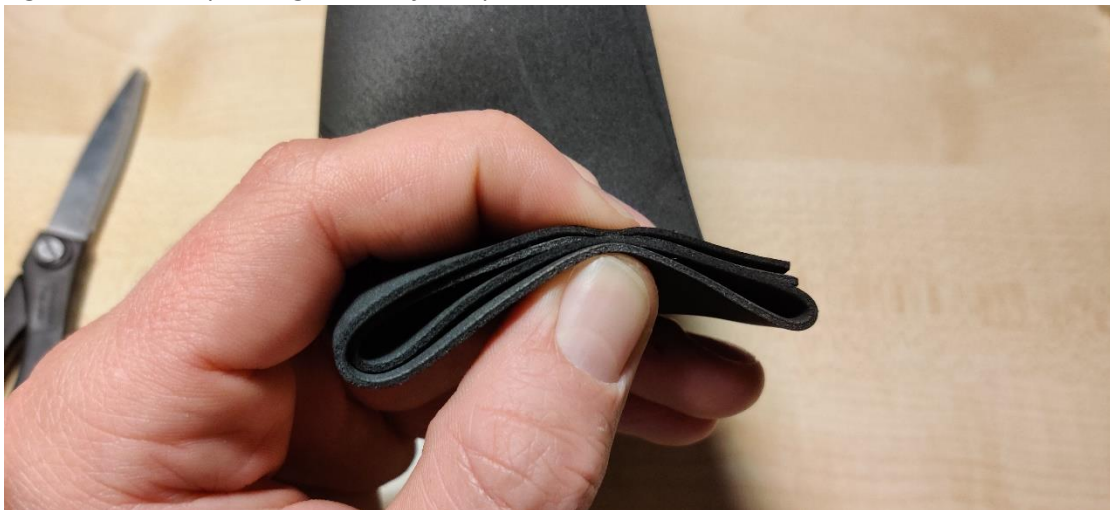
Figure FF17. Compressing multiple layers of EVA foam.
