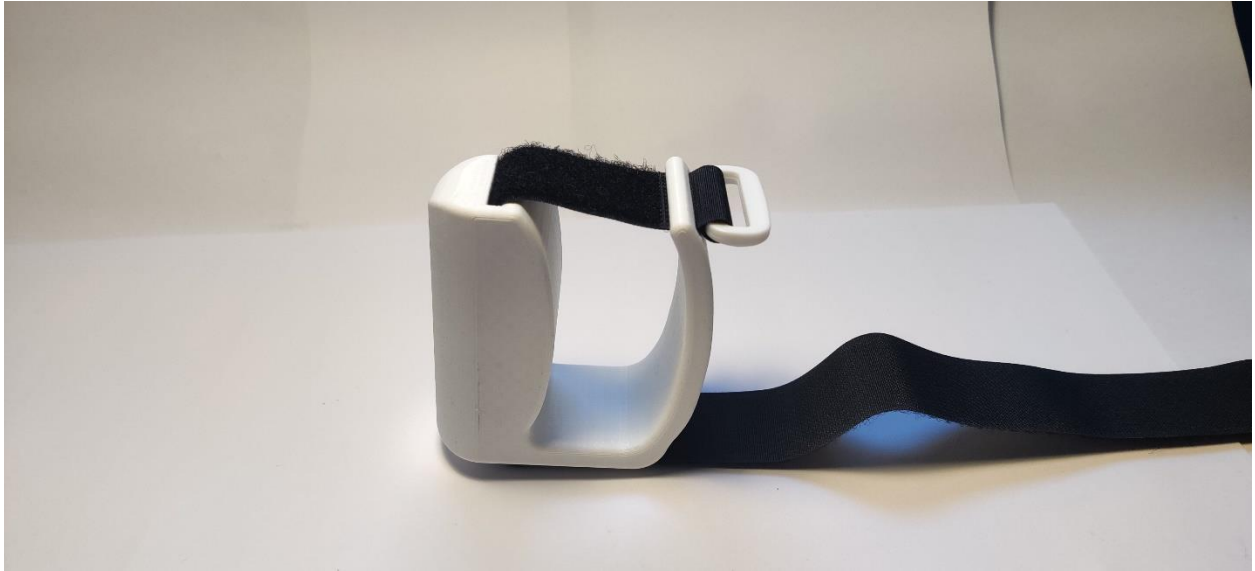
Figure P1. Hand fixation concept 1 with strap.
