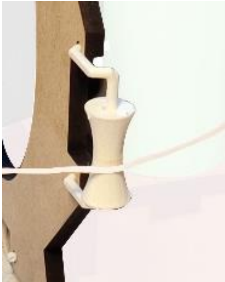
Figure H21. 3D-printed pulley and axis.
