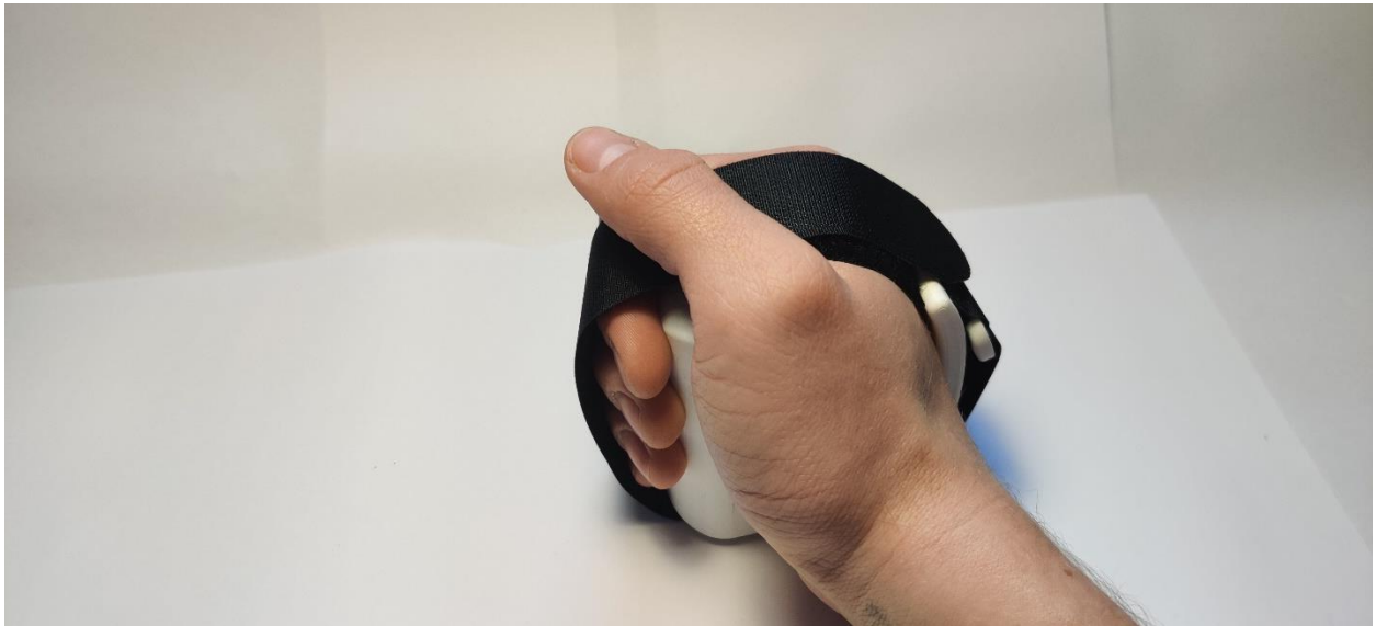
Figure P4. Hand fixation concept 1 with hand fastened and fingers underneath strap.
