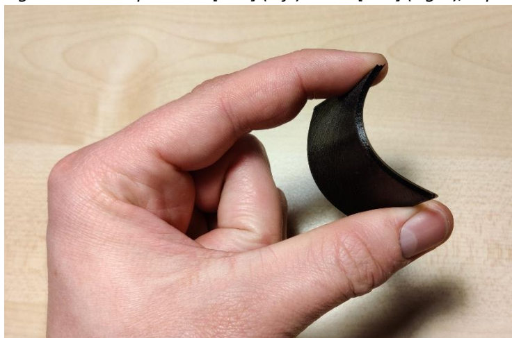
Figure FF2. Bending the TPU (2 [mm]) piece.
