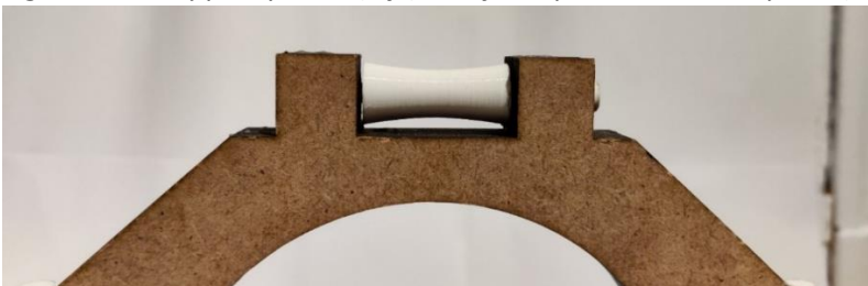
Figure H24. Pulley with axle integrated into wrist standard (v2).
