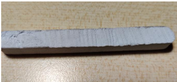
Figure FF4. Single-cell foam piece.
