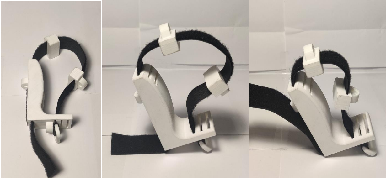
Figure H68. Concept 2 – V3 prototype with sliders and strap loose (left, middle) and fastened (right).
