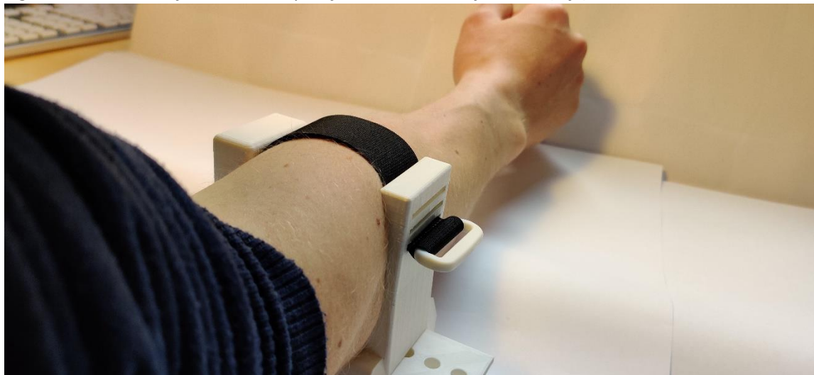
Figure L14. Forearm fixation concept 3 fastened around forearm (right).
