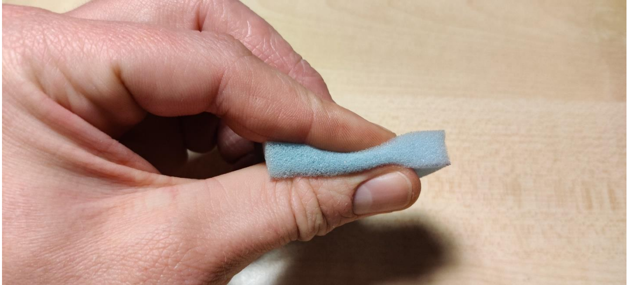
Figure FF9. Compressing the piece of polyether SG35.
