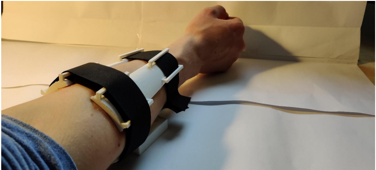
Figure L4. Forearm fixation concept 1 fastened around forearm (right).
