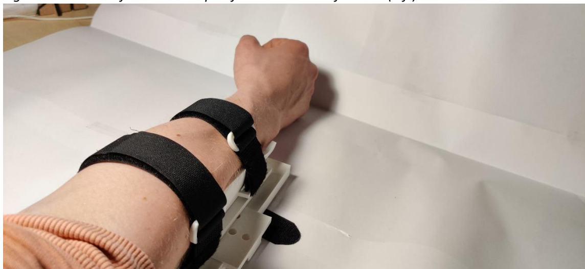
Figure L9. Forearm fixation concept 2 fastened around forearm (right).
