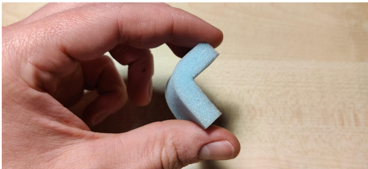
Figure FF8. Bending the piece of polyether SG35.
