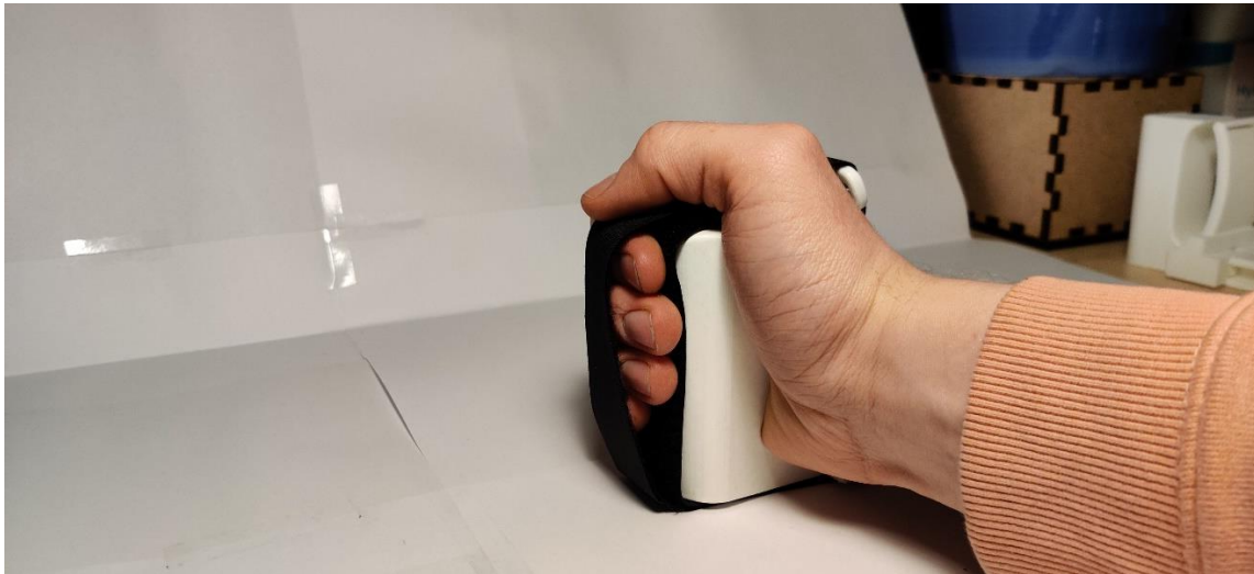
Figure P13. Hand fixation concept 3 with hand fastened with fingers underneath strap.
