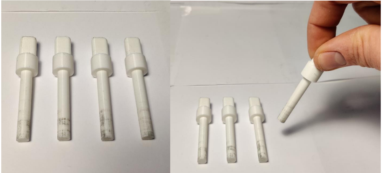
Figure H57. Small pins used to fix the position of the lower body part on the arm standard.
