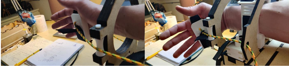
Figure AA1. Measuring required cable length for full wrist flexion movement (=12 [cm]).
