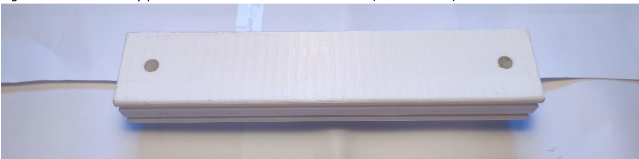
Figure H51. Lower body part with rails and attachment holes (top view).
