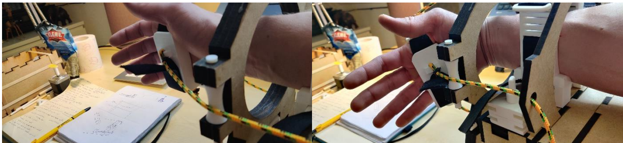
Figure X21. Measuring required cable length for full wrist flexion movement (=12 [cm]).
