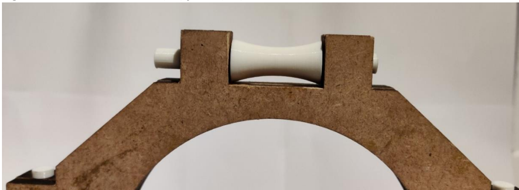
Figure H26. New pulley with axle integrated into wrist standard (v2).
