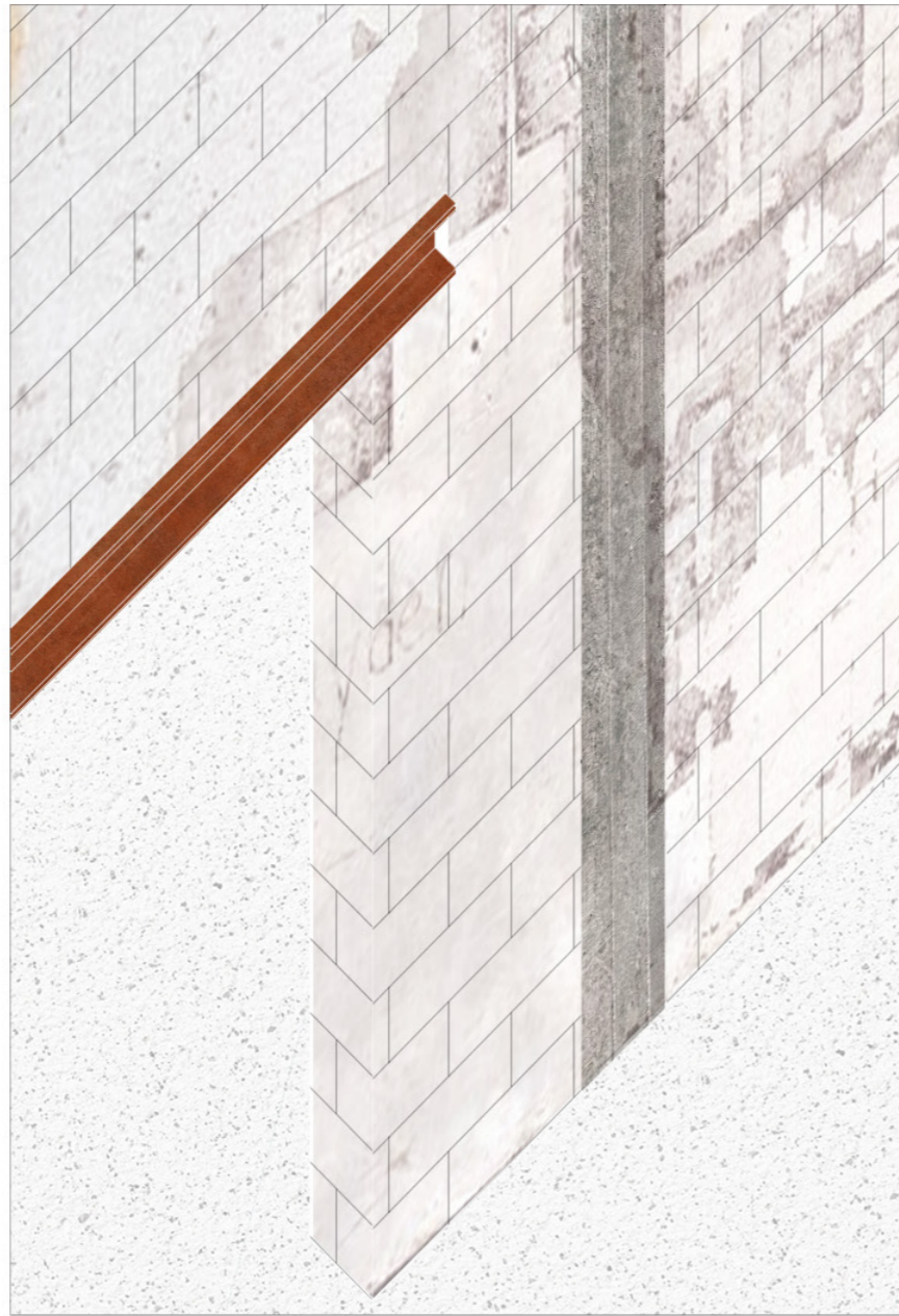
Portals existing blockwork wall aided by reused steel beam
