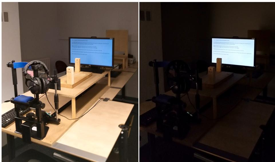
**Fig. 3.** Setup used in Experiment 2. Left: Setup in regular lighting conditions. Right: Setup in the lighting conditions of the experiment. The wooden structure was used for a test measurement for each participant and was removed before Task 1.
