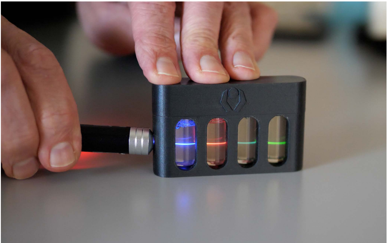
Figure 13: Paul Corstjens demonstrating the principle of photon upconversion. Different UCPs are present in the tubes. The UCPs are excited with a near-infrared laser.
