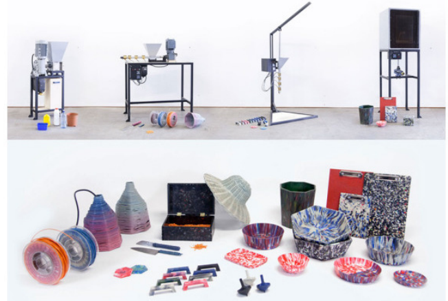
Fig. 3. The range of Precious Plastic machines (top) and examples of produced DIY plastics products (down).
