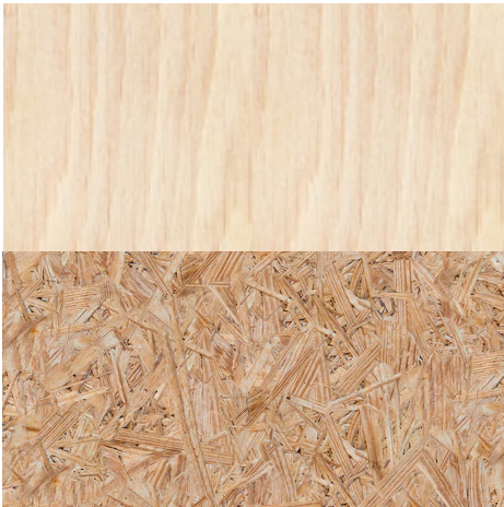
CLT & OSB OSB: recycled pressed wood flakes
