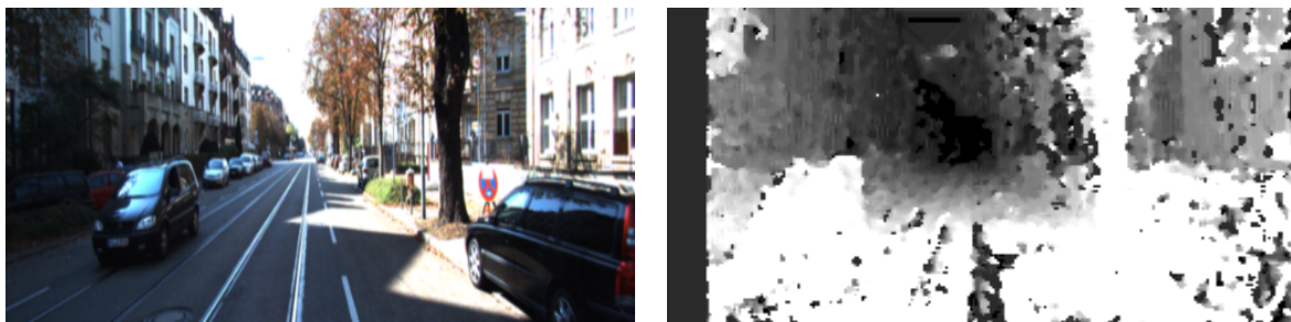
Figure 3.6: Demonstration of the output of SGBM. Input to the algorithm from KITTI [14] (left) Disparity output from SGBM algorithm (right)
