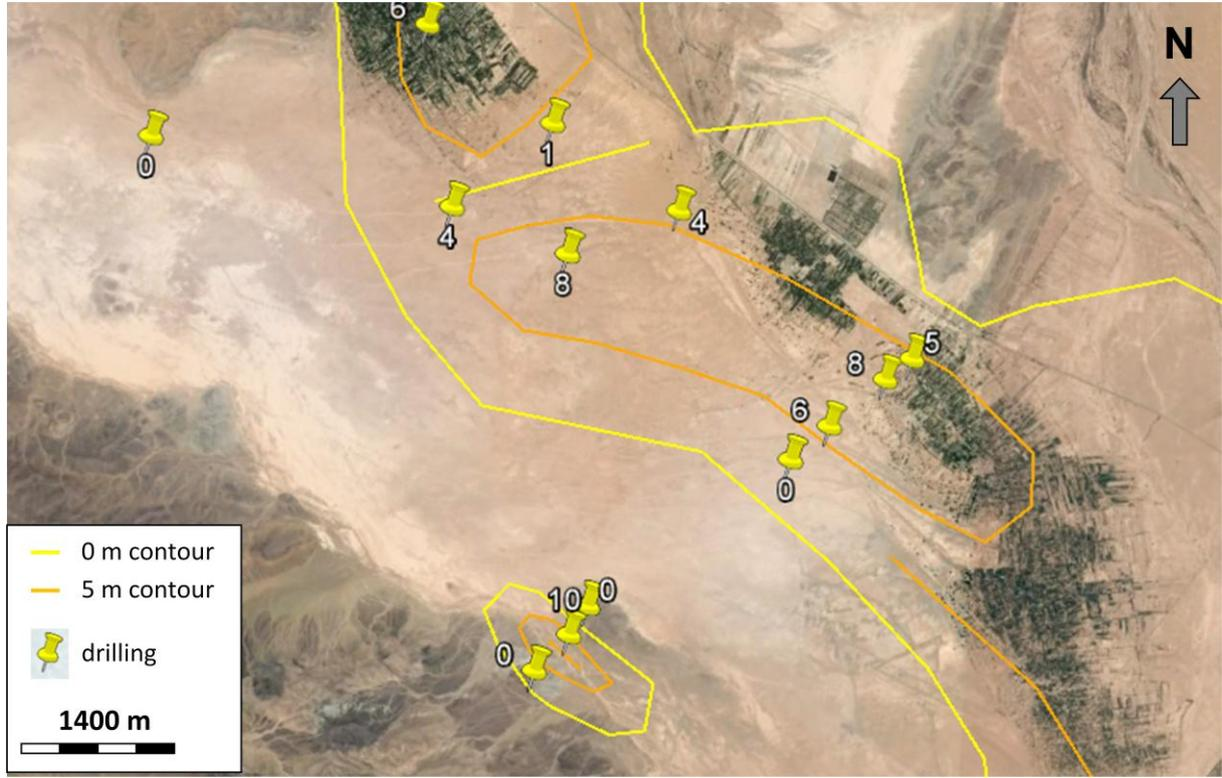
Figure 152: Drillings and contour information on the thickness of the gravel formation (zoom Hannabou).
