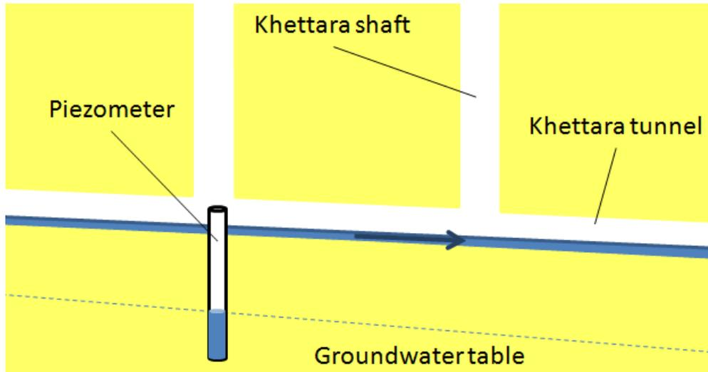
Figure 99: Schematization of a setting of a piezometer within a khattara tunnel.
