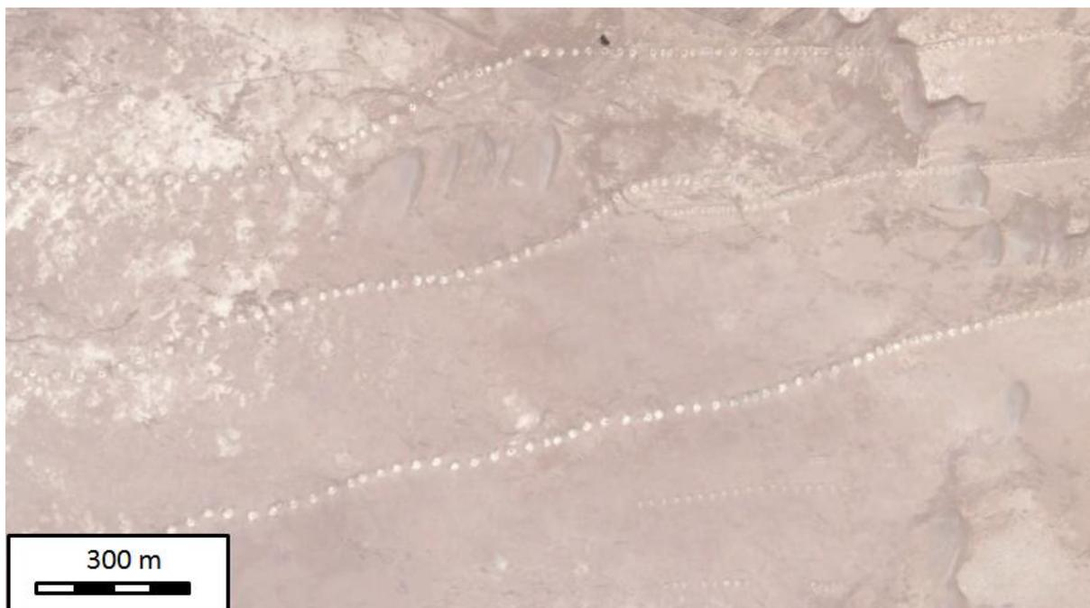
Figure 17: Satellite top view of several khetaras in the study area existing of hills which are made of excavation material from the shafts and the tunnel.
