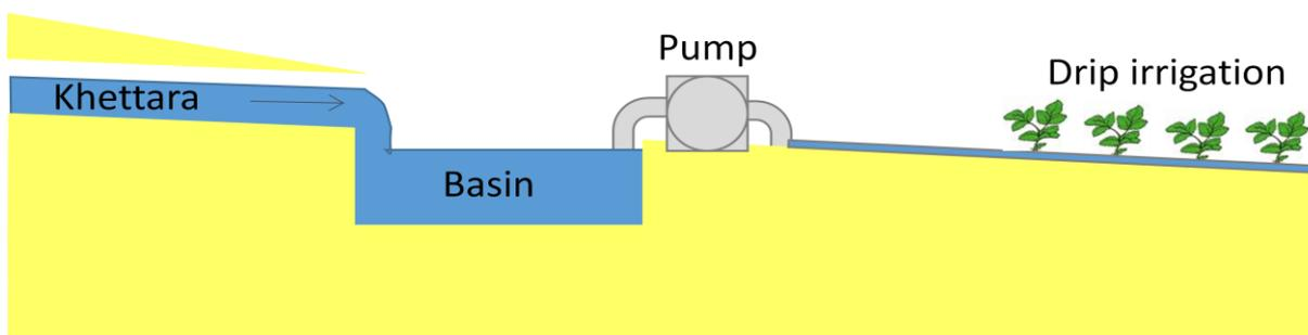
Figure 94: Schematic cross section of the combined use of khetaras and drip irrigation. The pressure is provided by a pump.
