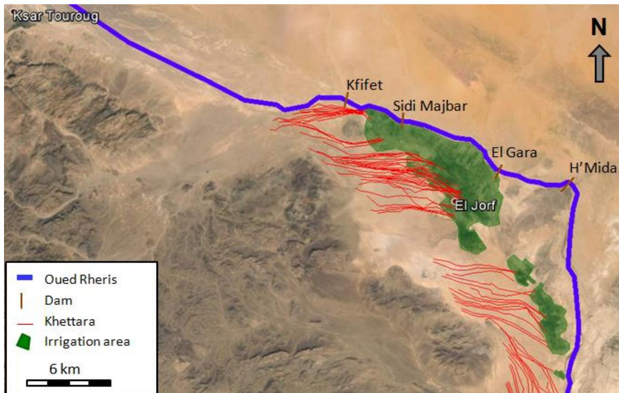
Figure 12: Hydrological map of the study area including water structures. A majority of the presented khattaras have fallen dry.
