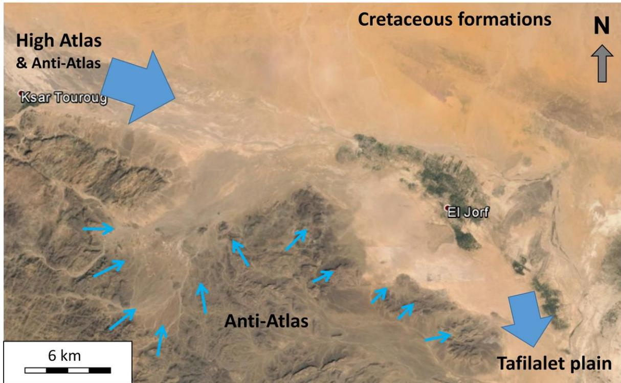
Figure 14: Groundwater in- and outflows and their origins/destinations.
