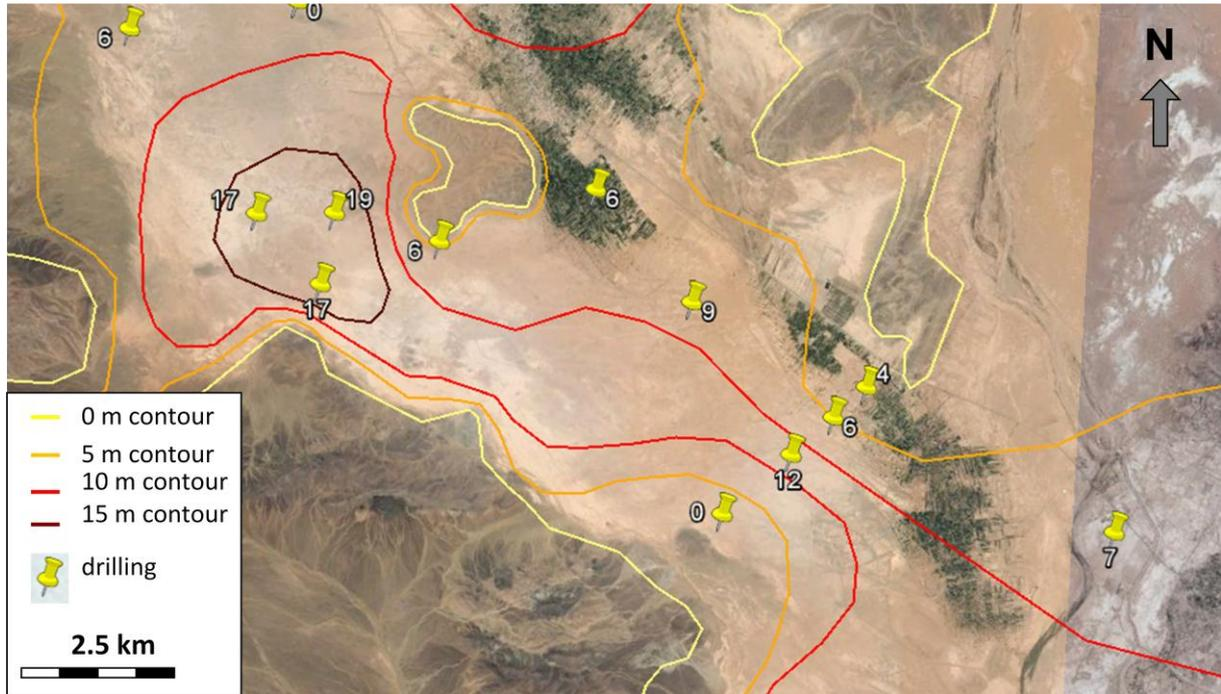
Figure 149: Drillings and contour information on the thickness of the silt formation (zoom Jorf and Hannabou).
