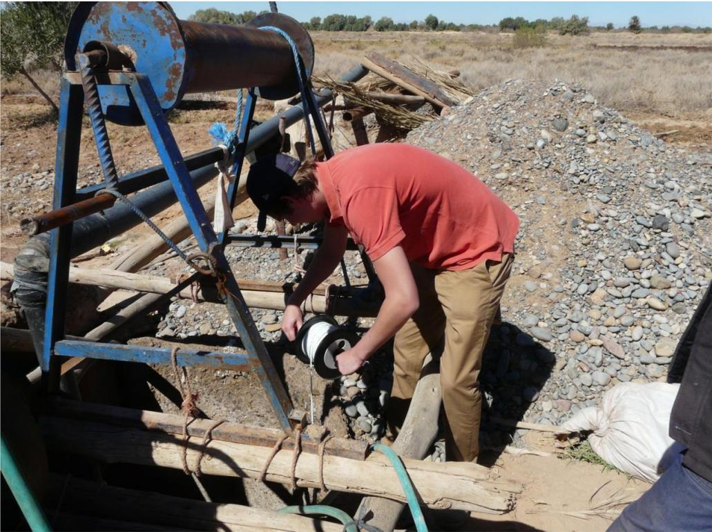
Figure 135: A water level measurement in an open well near Jorf with a water level meter. The loose pebbles on top of the hill, existing of excavation material from the well, indicate that the well goes down into poor cemented conglomerate (see location 5 in figure 130).
