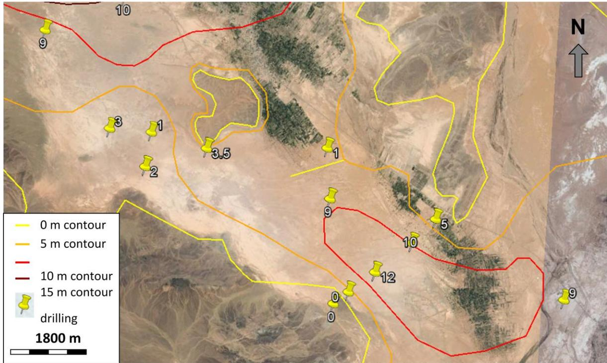
Figure 157: Drillings and contour information on the thickness of the conglomerate formation (zoom Jorf and Hannabou).
