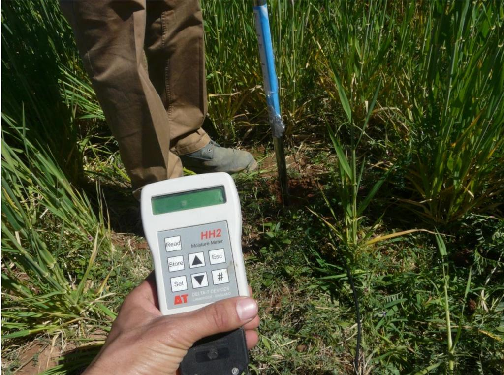
Figure 134: A water content test using an Edelman auger, a distance meter and a TDR-probe (see location 4 in figure 130).
