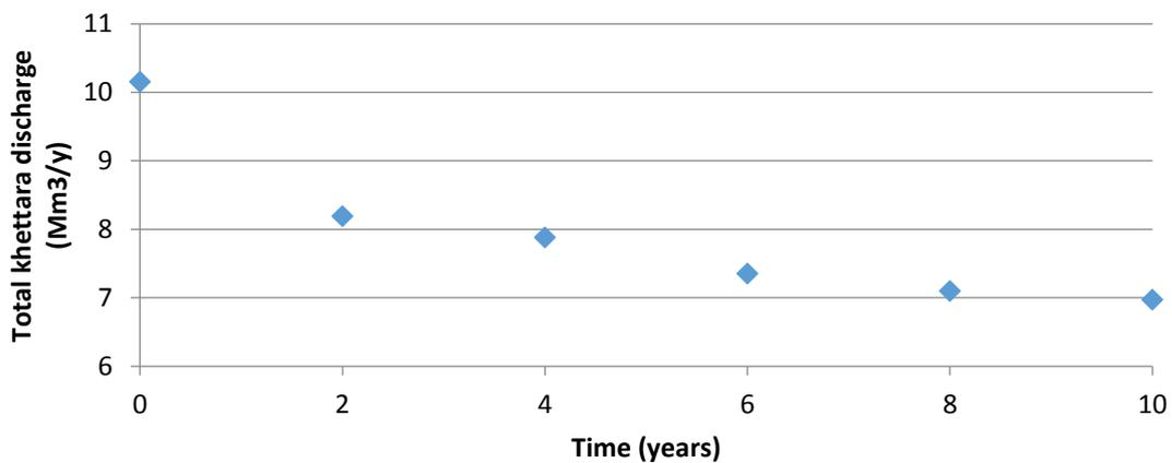
Figure 84: The calculated total khattara discharge in the model area during the entire drought period.
