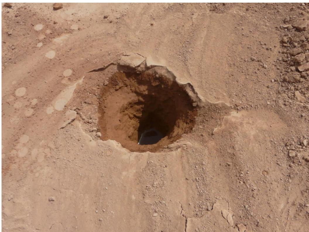
Figure 131: Infiltration test (see location 1 in figure 130). The drop of the water level was measured in time with a distance meter and a stopwatch. The hole was dug with an Edelman auger.
