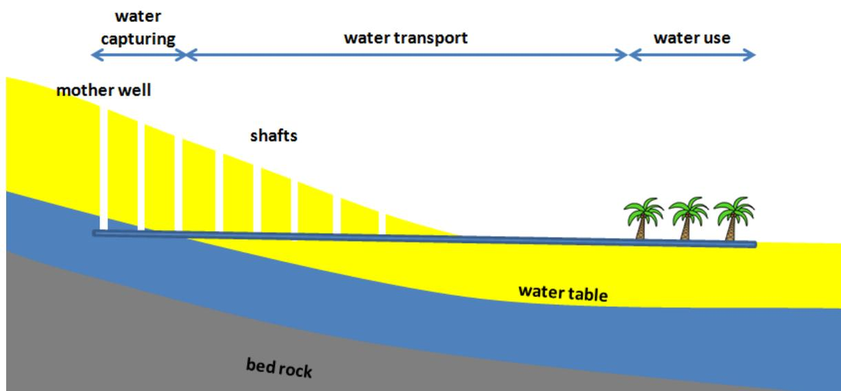
Figure 16: Schematic cross-section of a khettara.
