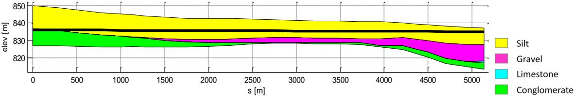
Figure 90: Cross section of the super khattara of Fezna in the model.
