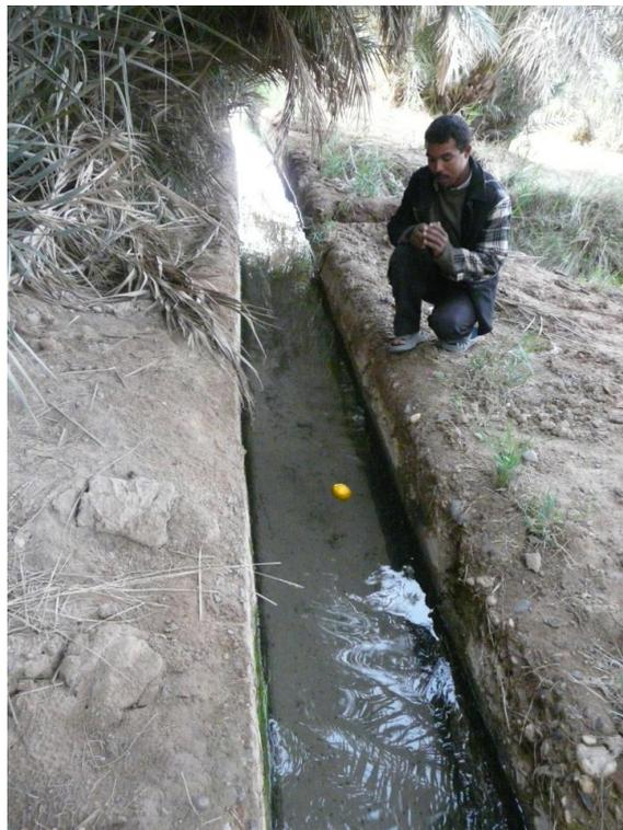
Figure 133: Khettara discharge measurement with a floating orange, a distance meter and a stopwatch (see location 3 in figure 130).
