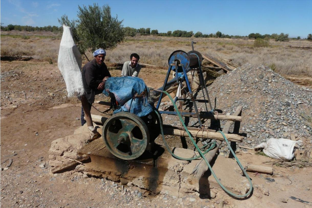
Figure 18: A typical diesel pump next to an open well. The hill behind exists of excavated material and indicates that the well reaches down to the conglomerate layer.
