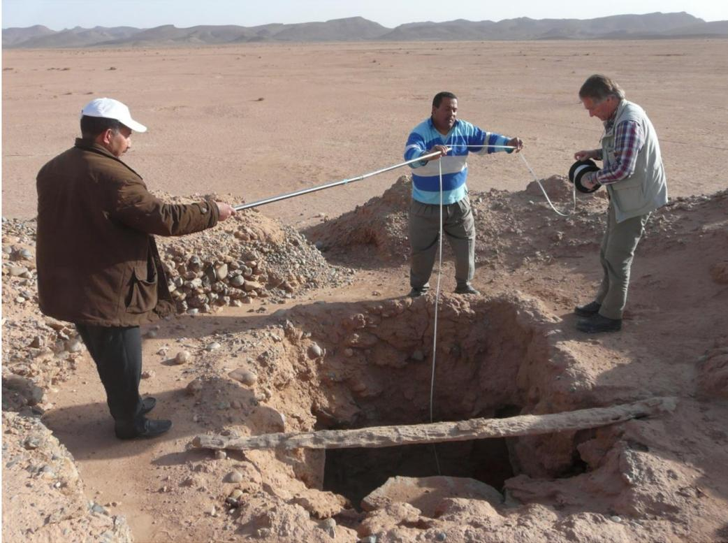
Figure 132: Measuring the mother well depth with a water level meter and a distance meter (see location 2 in figure 130).
