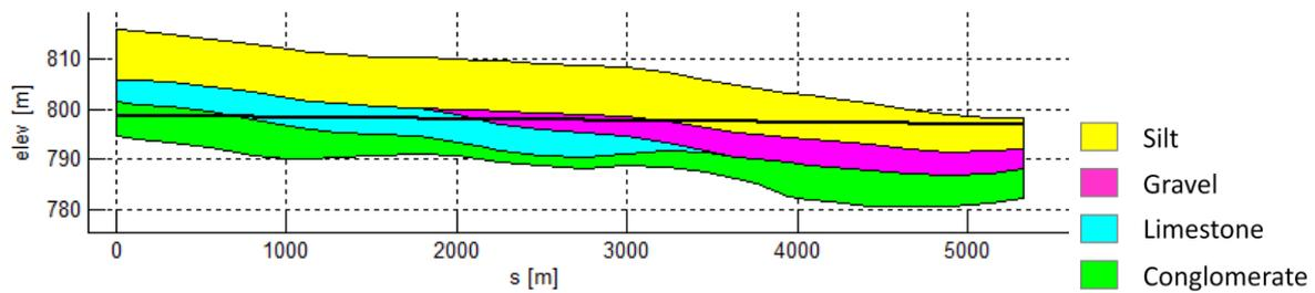
Figure 34: Cross-section of khattara Bouia Lakadima in the model (khattara of Hannabou). The black line represents the khattara, from upstream (left) to downstream (right).
