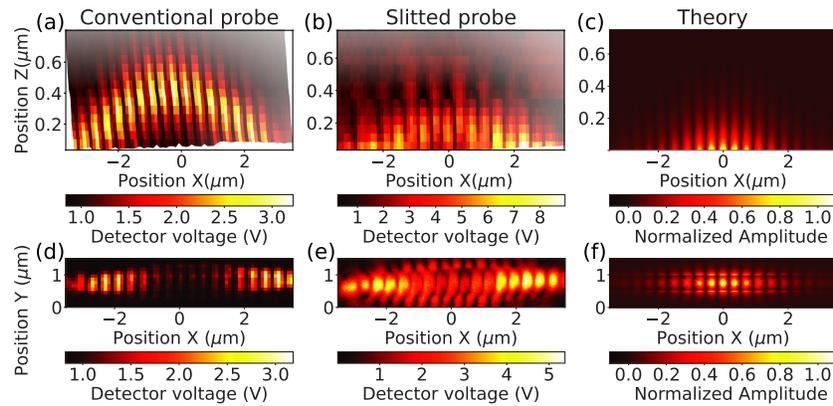
**Fig. 4.** Near-field amplitude maps measured through a near-field aperture probe at a wavelength of 1576.2 nm: (a) and (b) on the  $x - z$  plane, (d) and (e) on the  $x - y$  plane; (a) and (d) using a conventional probe, (b) and (e) using a nanostructured cloaked probe. The cloaked probe used here is Probe 3 in Fig. 3. These figures can be compared to the numerical calculations for the amplitude of  $E_y$  in the resonant cavity, presented in panels (c) and (f).
