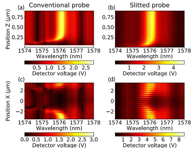
**Fig. 2.** (a) and (b) Transmission spectral measurements for the nanophotonic cavity in Fig. 1, with (a) a conventional or (b) a cloaked probe (Probe 3 in Appendix A) approaching the center of the cavity from the top. (c) and (d) Transmission maps with probes in contact with the sample and approaching the center of the cavity along its mirror-symmetry axis.
