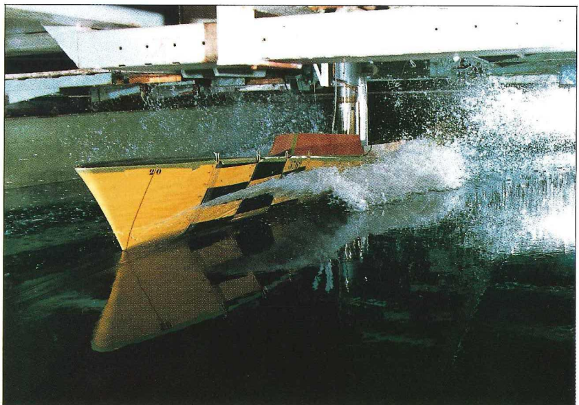
Tests in waves with a high speed ship. One of a family of hull forms, studied in a joint program with the Dutch and U.S. Navy.
