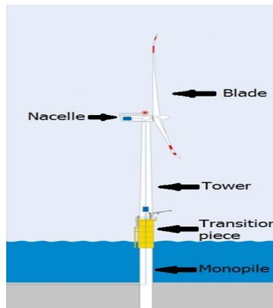
Figure 1: Different components of an offshore WTG.
