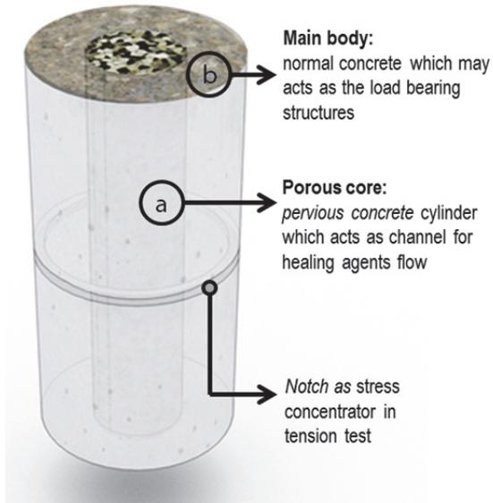
**Figure 2.11.** Artist render of Porous Network Concrete specimen. The cylinder specimen was designed to accommodate trial experiment proving the healing mechanism proposed.
