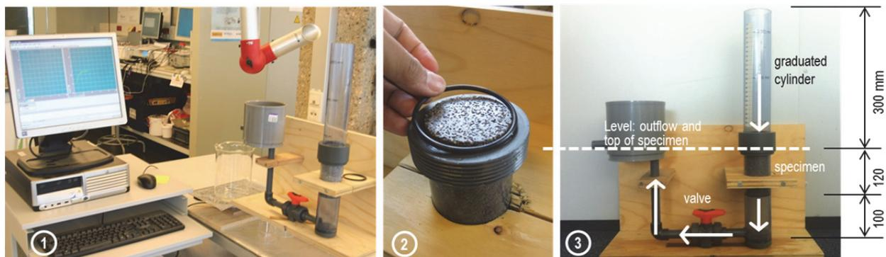
**Figure 2.10.** Setup of falling head permeability (hydraulic conductivity) test where (1) the permeameter is connected to PC for recording the time and weight increment of outflow water. (2) Specimen is inserted into permeameter setup and O-ring rubber is mounted to seal the setup from leakage. Frame (3) shows the scheme of water flow and dimension of the test cell.
