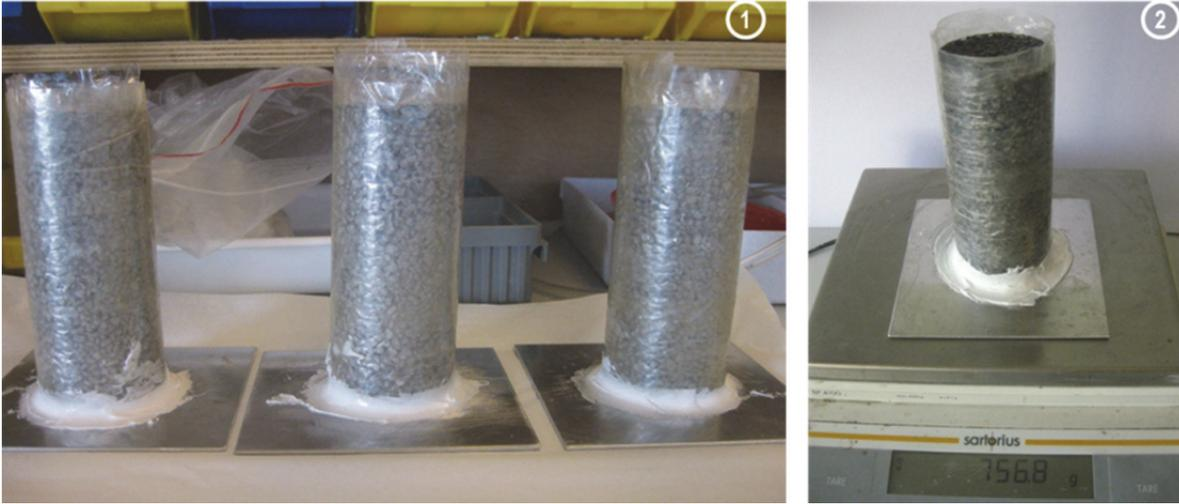
**Figure 2.6.** (i) Three porous concrete cylinders  $\text{Ø}56 - 120$  were enveloped with plastic membrane for measuring volumetric porosity, (ii) specimen was weighed on a scale.
