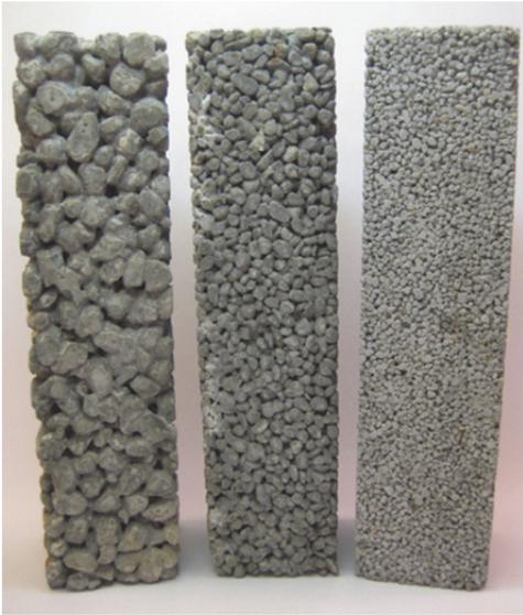
**Figure 2.5.** Three porous concrete prisms 40 × 40 × 160 mm were made with different aggregate size, from left to right; 4-8 mm, 2-4 mm, and 1-2 mm.
