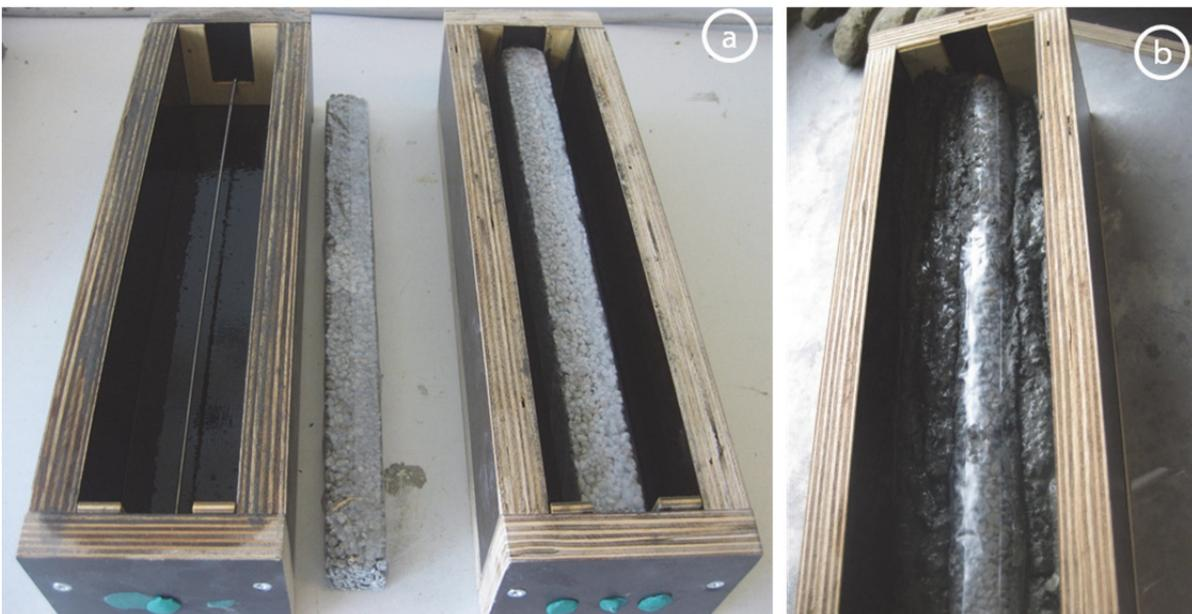
**Figure 2.16.** Production of PNC prism; Figure (a) shows the mould with  $\varnothing 2$  mm steel rebar that was put underneath the porous core prism which is supported by a wooden hook. Figure (b) demonstrates how the 'dense-normal' concrete is cast around the core.
