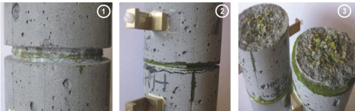
**Figure 4.4.** (1) The crack formation in the notch, (2) the new crack formation after the first was healed, and (3) the new crack face
