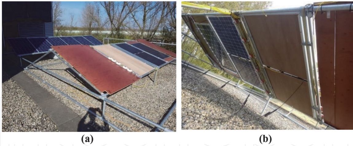
Figure 15. (a) Measuring POA^{rear} irradiance with the front side coverage of the PV module, and (b) Measuring POA irradiance with the rear side coverage of the PV module. This is then subtracted from the output of the second uncovered module.
