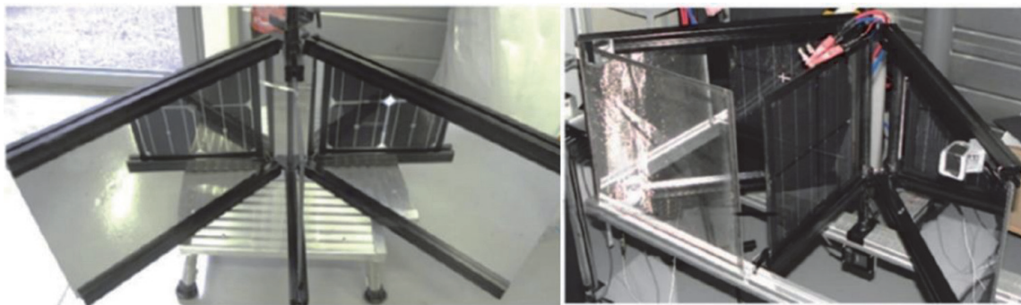
Figure 3. Two-mirror setup for bifacial PV module characterization [81].
