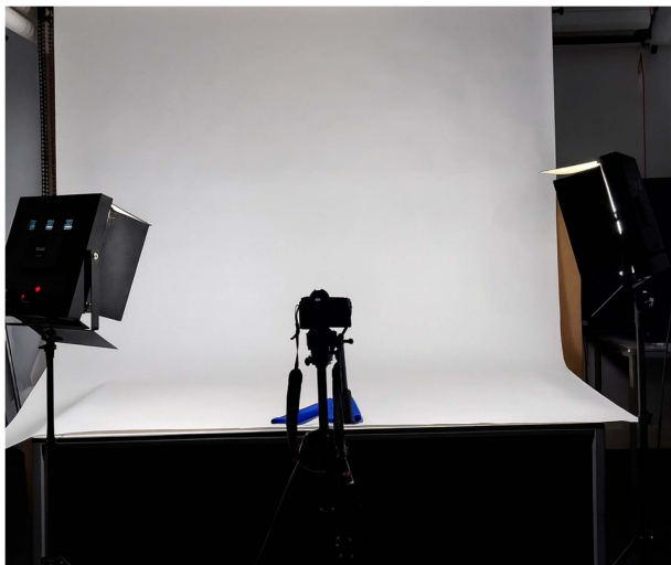
Fig. 2. Photographic setup consisting of two LS-1200 LED Panels for bright, homogeneous lighting, a Canon EOS 5D Mark II camera on a tripod, a white paper backdrop, and a blue velvet fabric (32 x 46 cm).
