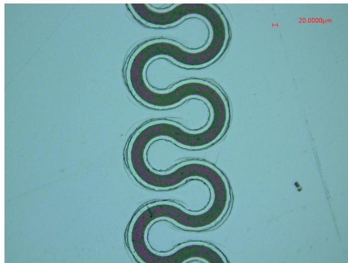
Figure 5.19: Illustration of two TiN contact of Electrode encapsulated between two layers of polyimide above PDMS polymer.
