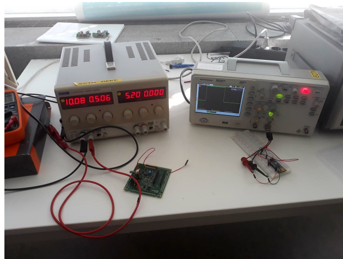
Figure 4.3: Entire measurement set up which includes the power supply of 30V, an oscilloscope, a multimeter and the testing PCB.
