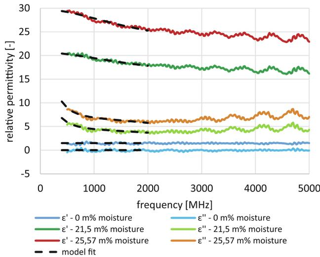
**Fig. 5.** Dielectric spectra of soil samples at 0 m%, 21.50 m%, and 25.57 m%. The spectra are measured with Agilent equipment: an 85070E performance probe kit, an E5071C network analyzer, and an N4691B ECal module.
