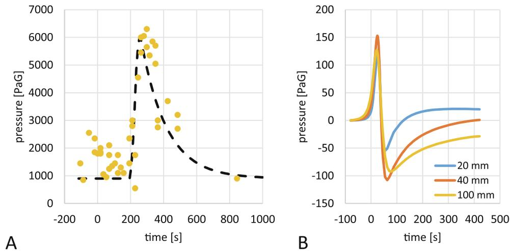
**Fig. 13.** Measurements of pressure at a depth of 10 cm during a field trial (left), and simulated pressure transients (right). A SMC PSE543A pressure transducer was used for the measurement. The dashed line is included to guide the eye.
