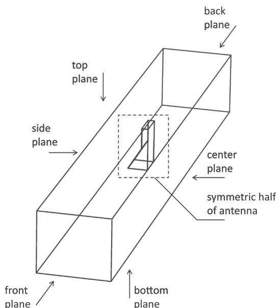
Fig. 2. Model geometry.
